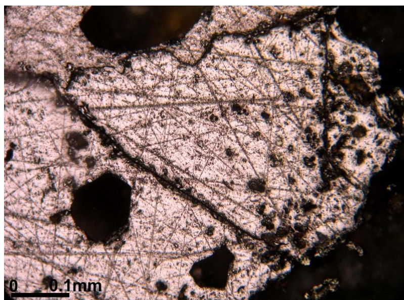
Figure 5-19. Photomicrograph of massive ore showing a highly fractured pyrite, a result of strong mechanical deformation (Sample KA79).
