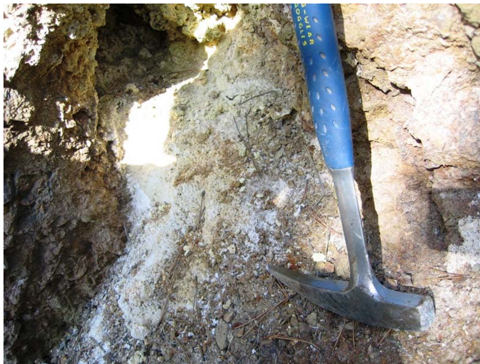
Figure 4-12. Late-stage argillic alteration of gossanized basalt outcrop proximal to the sulfide-bearing quartz veins within Karaboyalık Stream.
