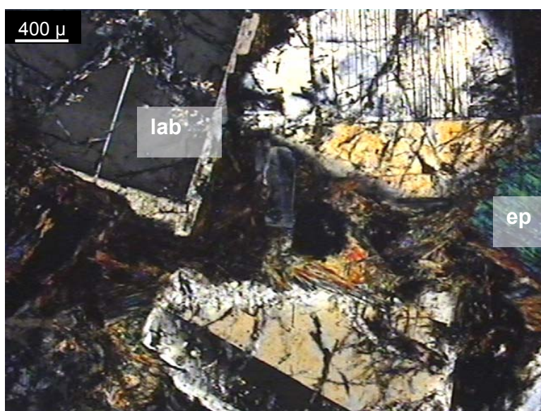
Figure 5-13. Photomicrograph of a coarse-grained gabbro sample showing labradorite (lab) phenocrysts with typical Carlsbad and albite twins. Interstices between labradorite crystals are occupied by epidote (ep) grains (Sample KA29, x4, XPL).
