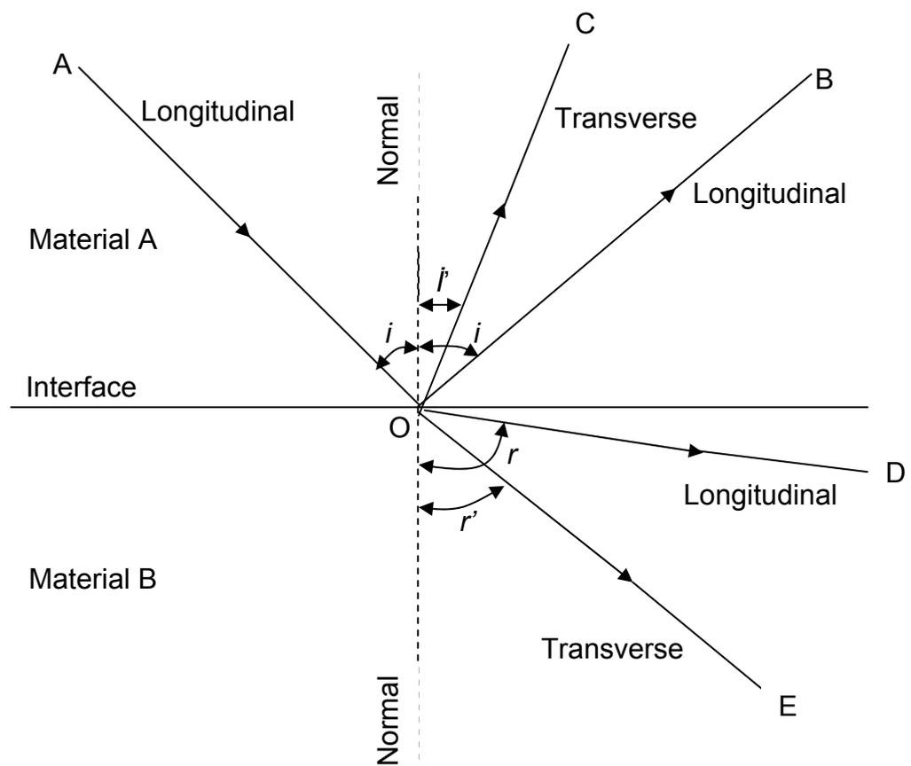
**Figure 7. Reflection and Refraction of Ultrasound at a Boundary**
