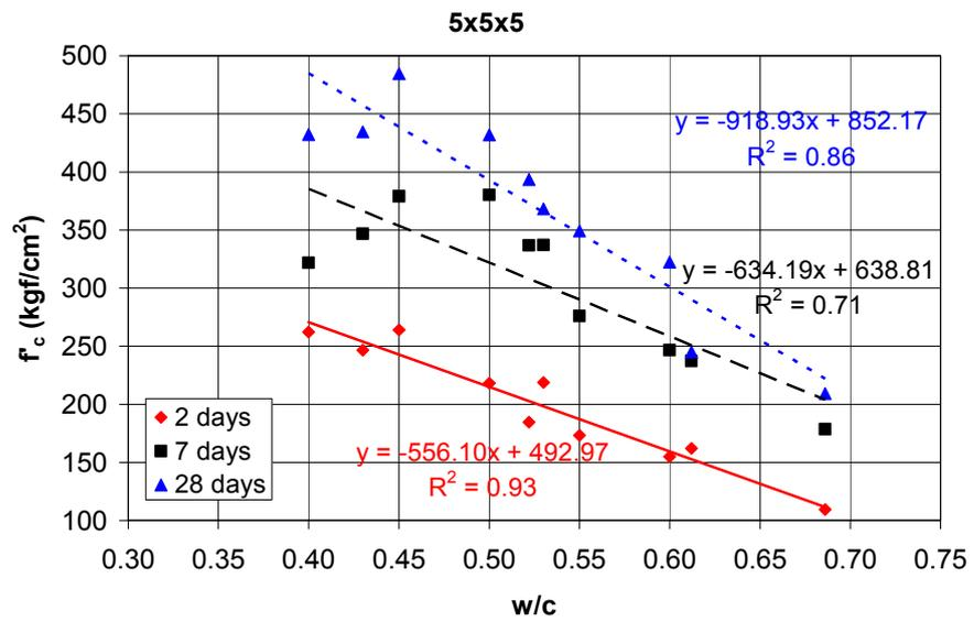
**Figure 18. Effect of w/c ratio on Compressive Strength**
