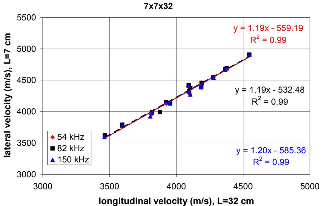
**Figure 26. Longitudinal and Lateral Pulse Velocity of Mortars with different Frequencies at 28 days**
