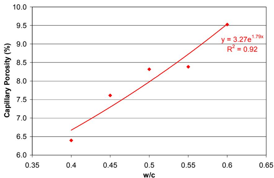
Figure 27. The relationship between the w/c ratio and capillary porosity
