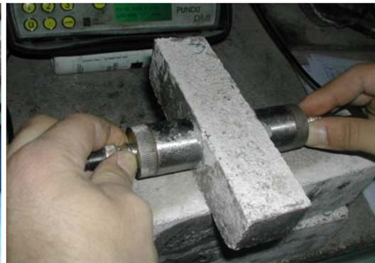
**(b) Through the cross section of a prismatic beam**
