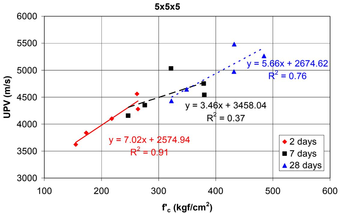
**Figure 25. The relationship between Compressive Strength and UPV (150 kHz)**
