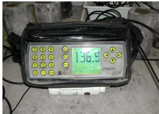
**Figure 10. Pulser-Receiver and the Display Device used in This Study**
