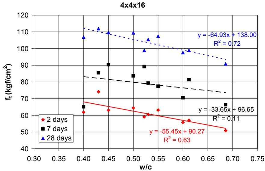
**Figure 19. Effect of w/c ratio on Flexural Strength**
