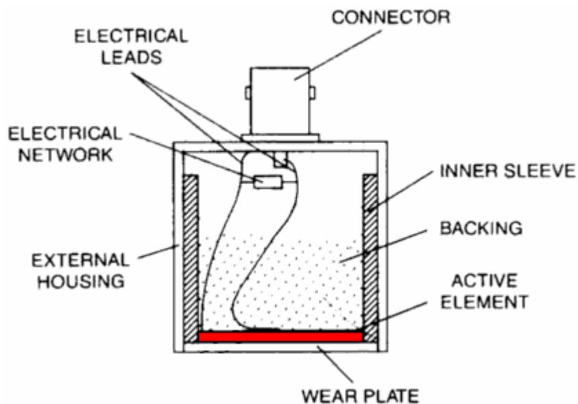
**Figure 9. Schematic Description of Piezoelectric Transducers [NDT Resource Center web site 2004].**
