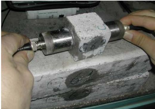
**(c) Through the length of a cubical specimen**
