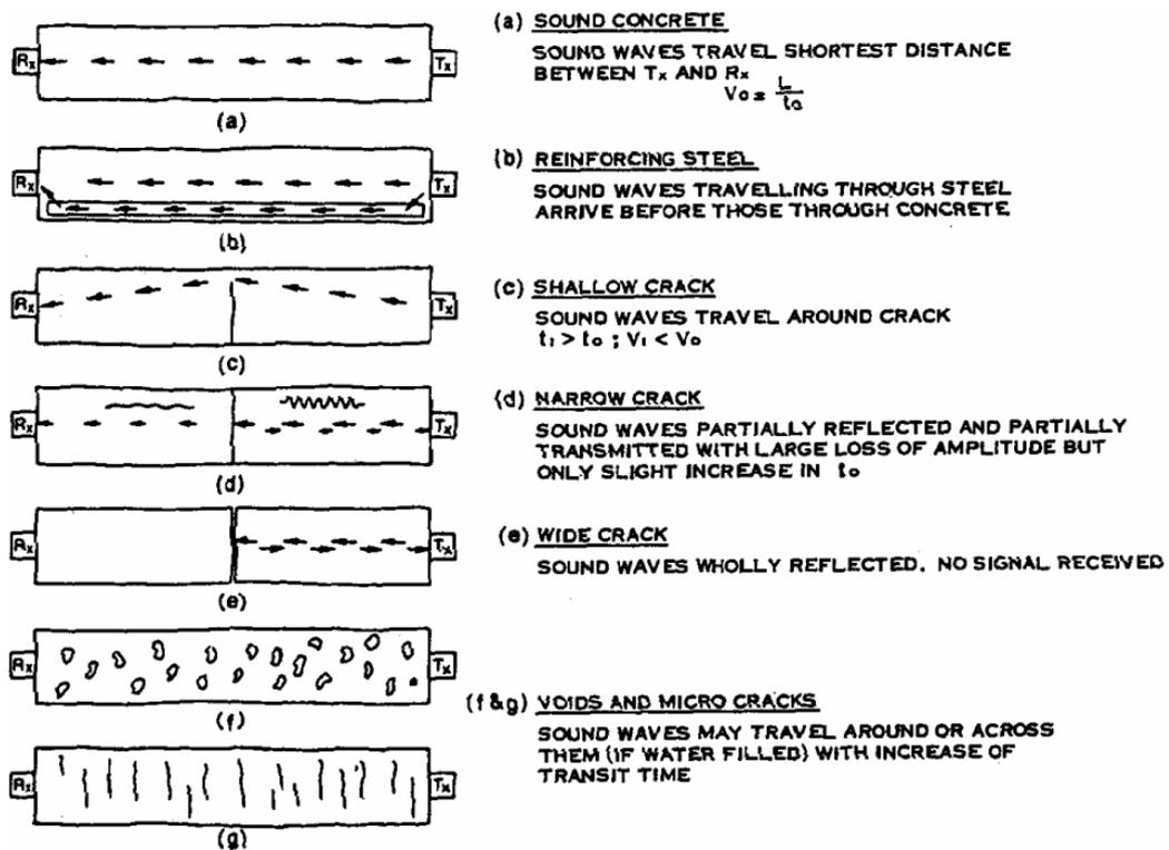
Figure 11. Conditions that Influence Transmission of Sound Waves in Concrete [Sturup et.al. 1982]
