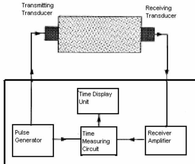
**Figure 8. Schematic Description of Pulse Velocity Testing Unit [ASTM C 597]**
