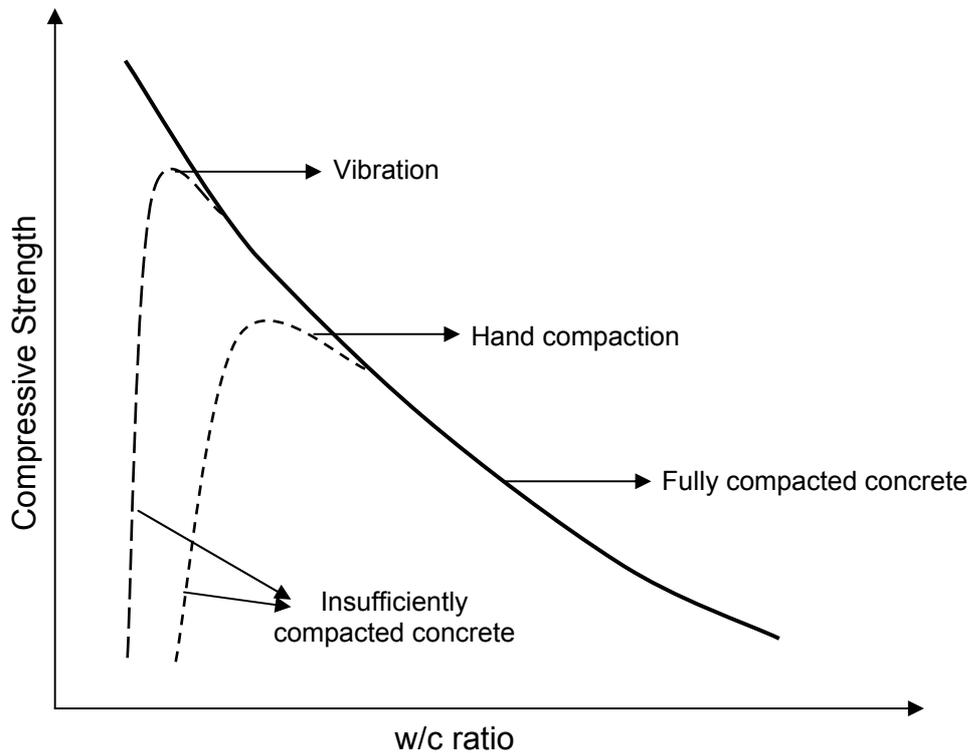
**Figure 17. Relationship between the w/c Ratio and Strength [Erdoğan 2002]**
