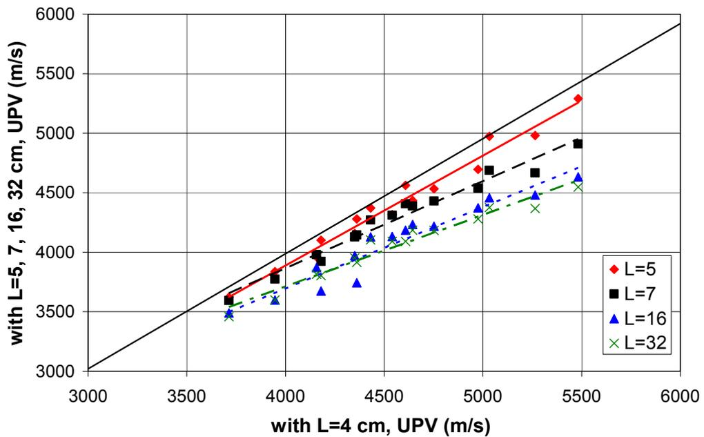
Figure 23. Reduction in UPV with Changing Measurement Length (150 kHz)
