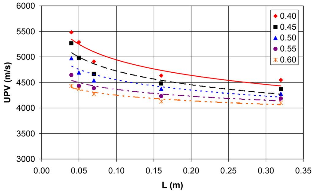
Figure 22. The relationship between UPV and Measurement Length (28 days and 150 kHz)
