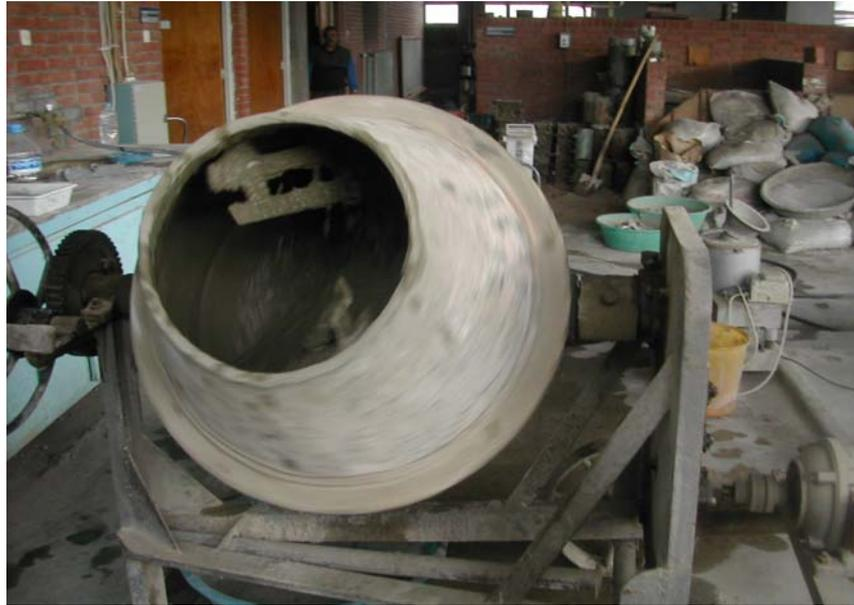
**Figure 12.The Mechanical Mixer**
