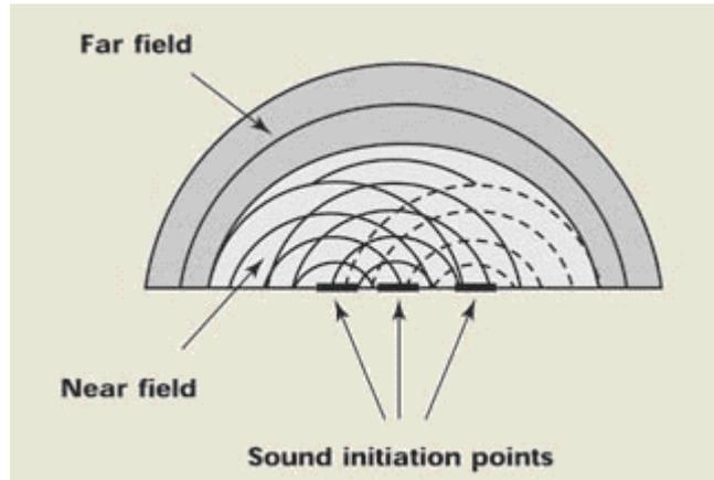
**Figure 5. Near Field Zone in Ultrasonic Testing [ASNT web site 2005]**
