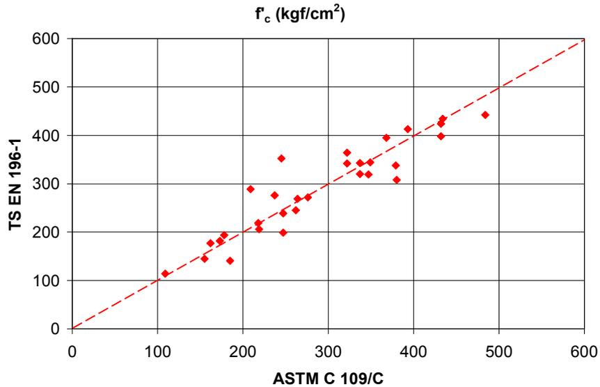
**Figure 21. Comparisons of ASTM C 109/C and TS EN 196-1**
