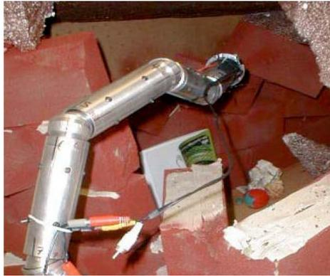
Figure (1.1) Search and Rescue Demonstration by a Serpentine Robot [6].
