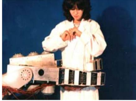
Figure (2.23) The flexible gripping action by the Soft Gripper II on a human body
