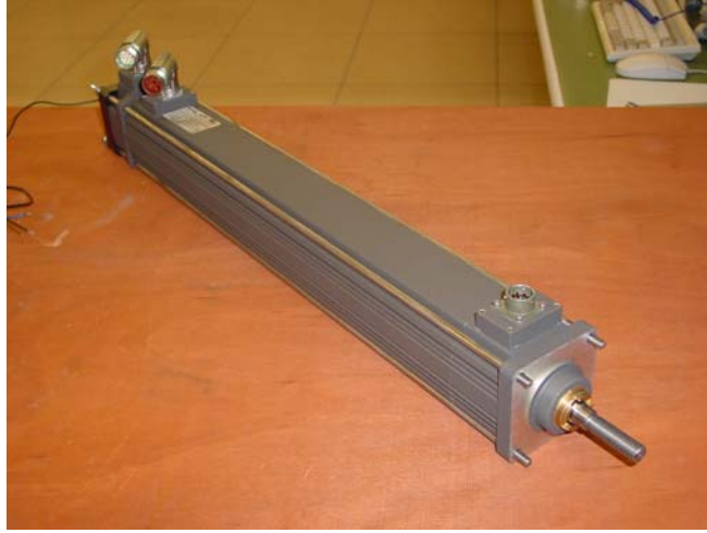
Figure 4.3: Linear actuator used in the tank simulator
