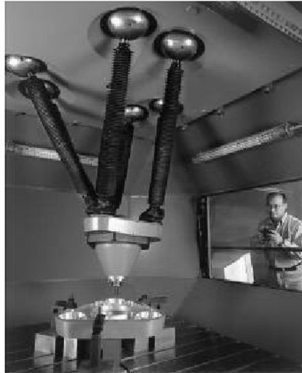
Figure 1.4: Stewart Platform as a machine tool
