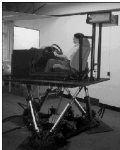
Figure 1.3: A typical Stewart Platform as motion simulator
