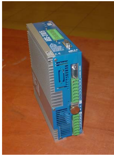
Figure 4.4: Motor driver used in the Stewart Platform
