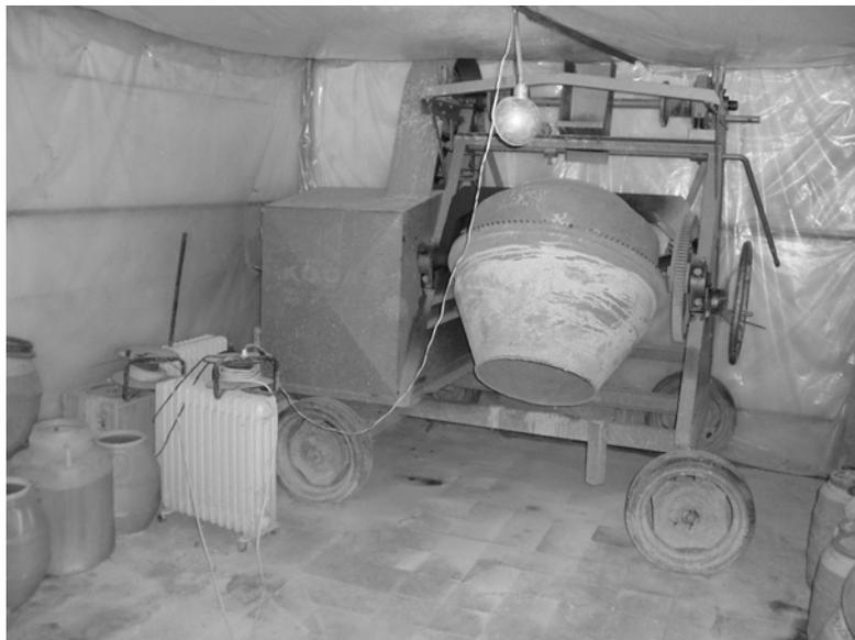
Figure 3.2 Mixer used for prolonged mixing of concrete and containers for curing of concrete at 50°C
