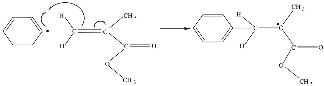
**Figure 1.7** Initiation step of MMA polymerization
