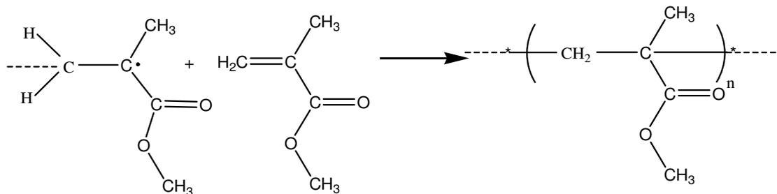
**Figure 1.8** Propagation step of MMA polymerization
