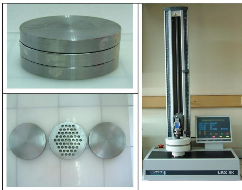
**Figure 3.2** Compression mould and test set up
