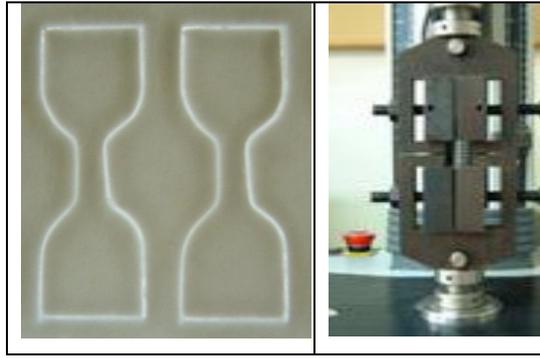
**Figure 3.1** Tension test samples and test set up
