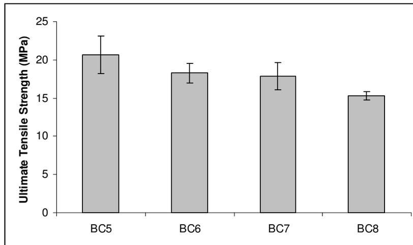
**Figure 4.10** Ultimate tensile strength values of DDM containing bone cements
