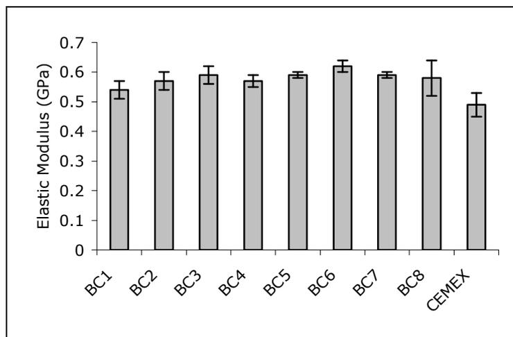
**Figure 4.20** Elastic modulus values of prepared bone cements
