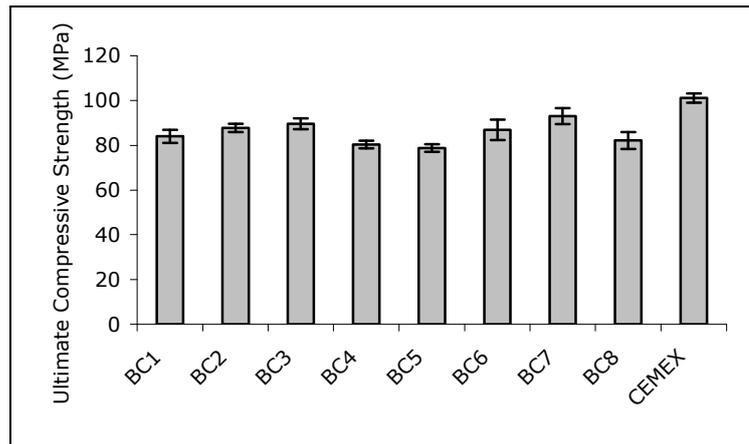
**Figure 4.19** Ultimate compressive strength values of prepared bone cements
