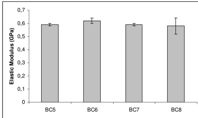
**Figure 4.18** Elastic Modulus of values of DDM containing bone cements
