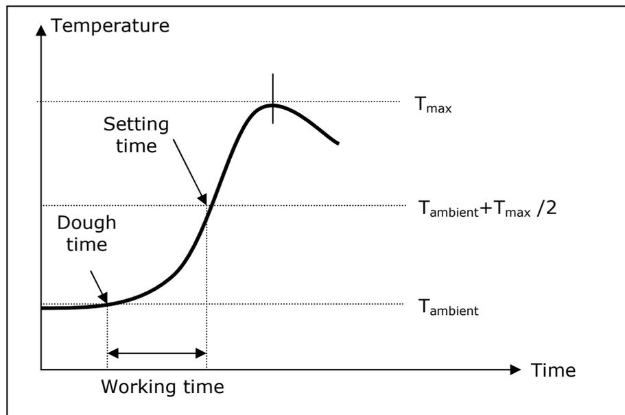
**Figure 3.3** Typical temperature versus time graph [31]
