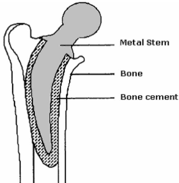
**Figure 1.4** Schematic illustration of bone cement in hip joint prosthesis
