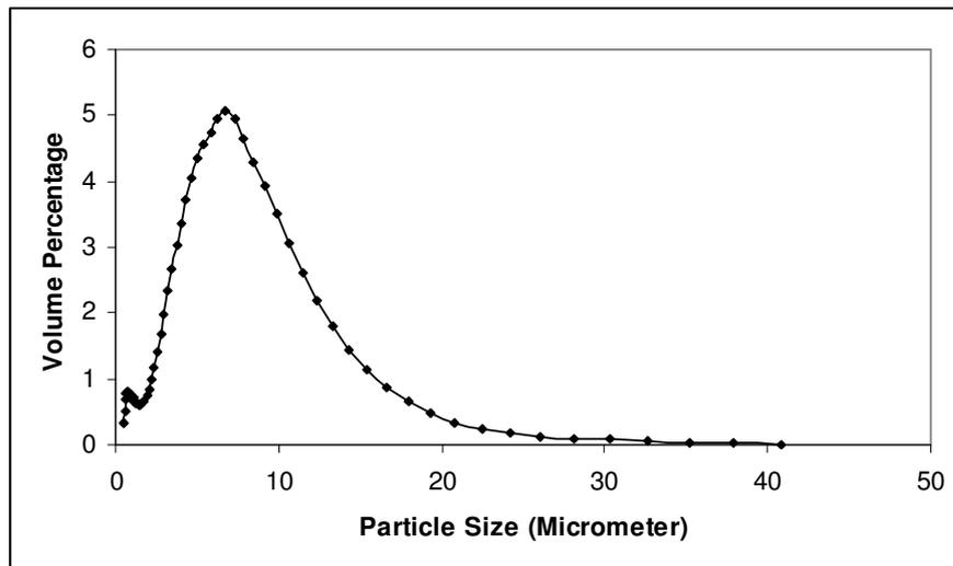
**Figure 4.7** Particle size distribution of BaSO<sub>4</sub> particles
