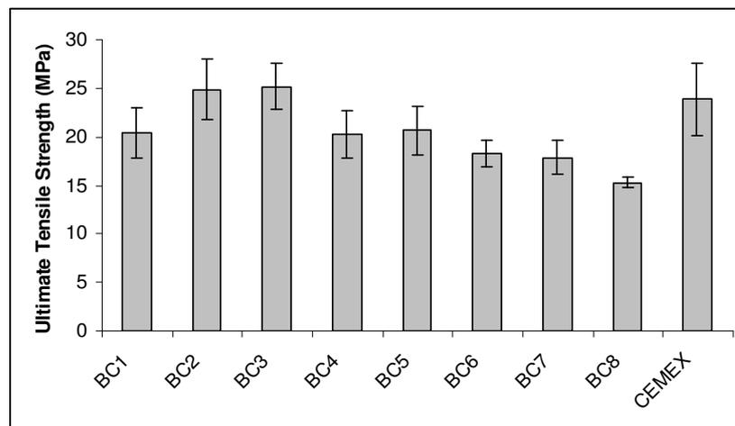
**Figure 4.12** Ultimate tensile strength values of the prepared bone cements
