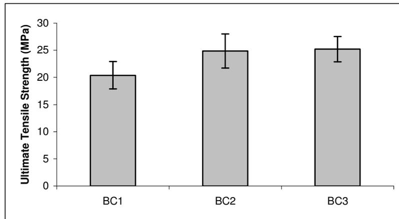
**Figure 4.8** Ultimate tensile strength values of HA containing bone cements
