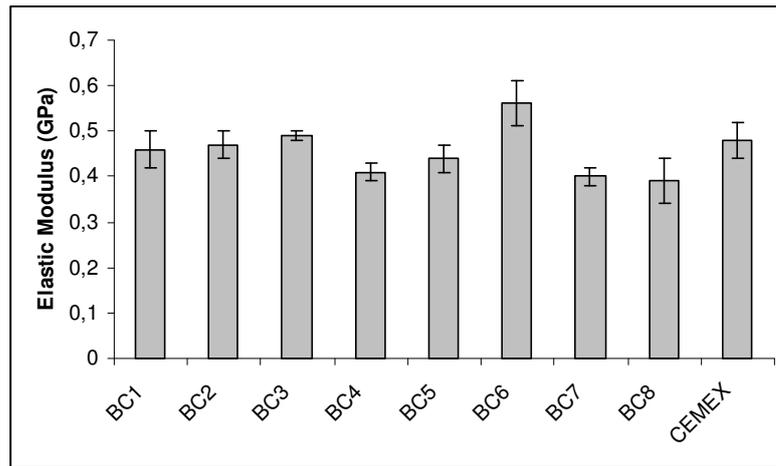
**Figure 4.13** Elastic modulus values of the prepared bone cements
