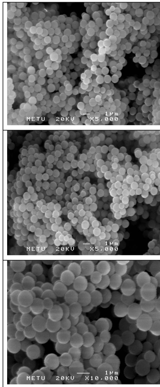
**Figure 4.4** Scanning electron micrographs of PMMA microspheres
