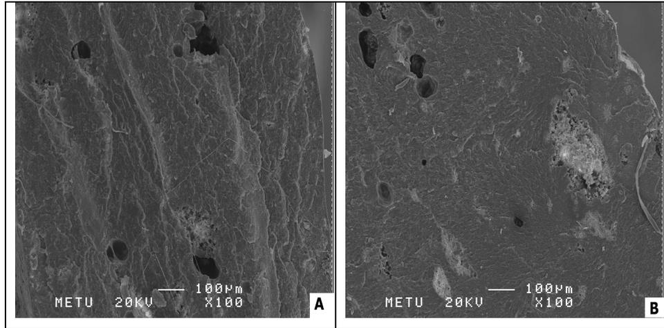
**Figure 4.23** Pore distribution of bone cements A) with 1% DDM (BC6) and B) with 3% DDM (BC7)
