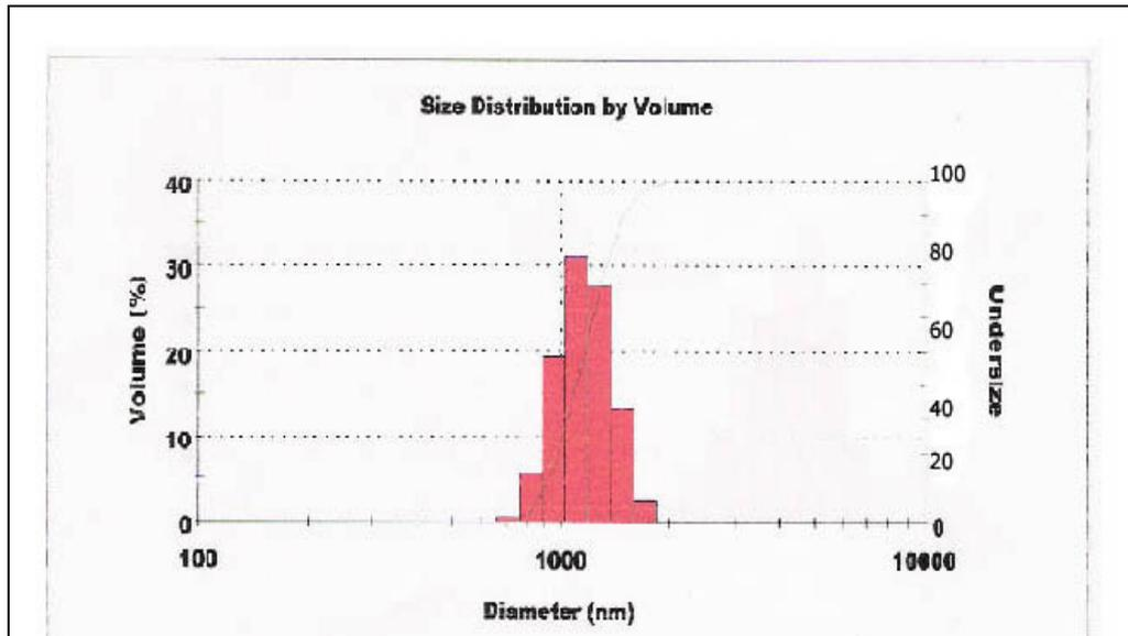
**Figure 4.5** Particle size distribution of PMMA microspheres
