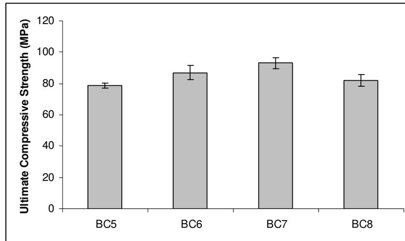
**Figure 4.17** Ultimate Compressive Strength values of DDM containing bone cements
