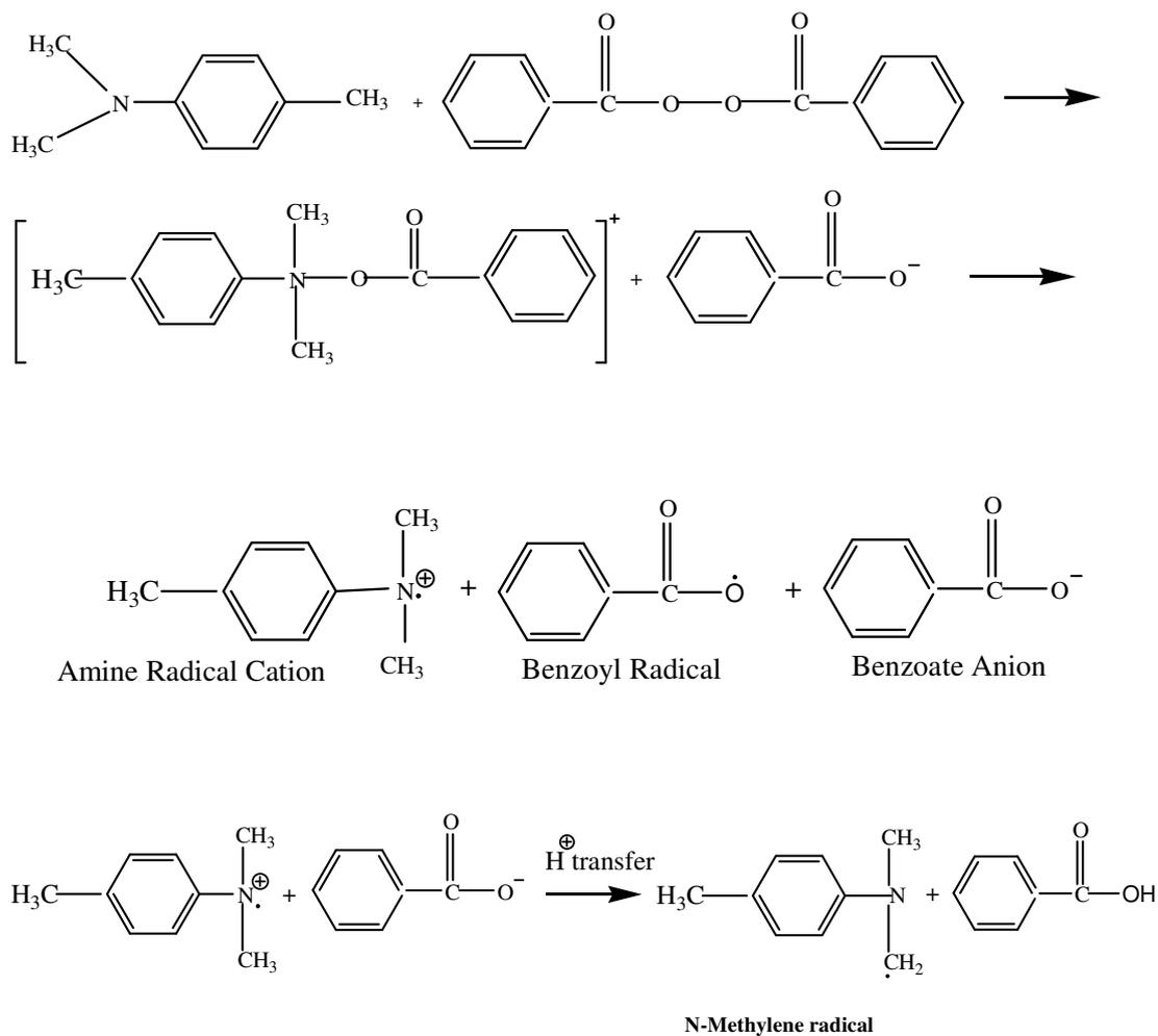
**Figure 1.5** Redox reaction between BPO and DMPT
