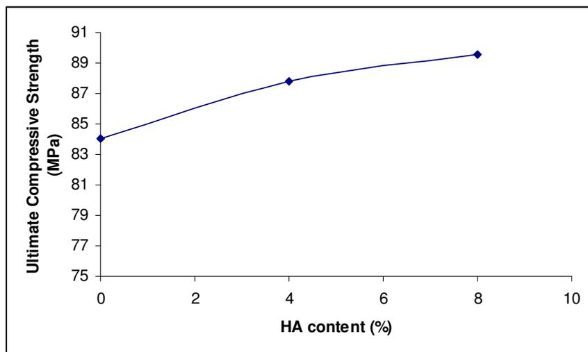
**Figure 4.15** Change in ultimate compressive strengths of 0%, 4%, 8% HA containing bone cements
