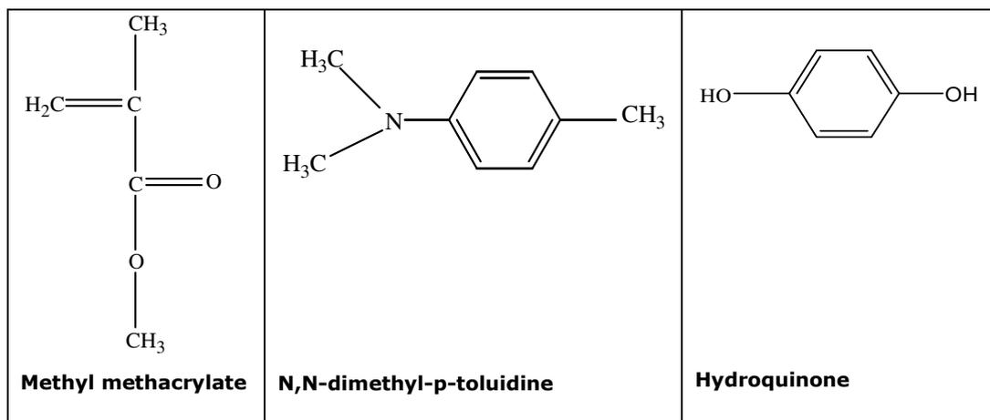
**Figure 1.3** Chemical structures of liquid components
