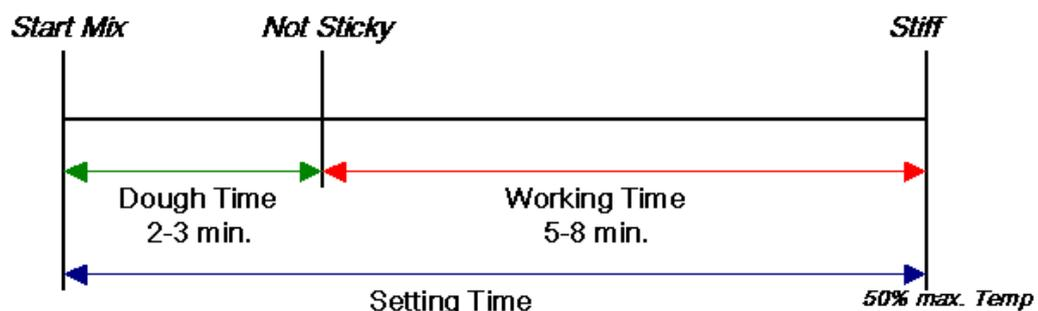
**Figure 1.10** Illustration of dough time, working time and setting time
