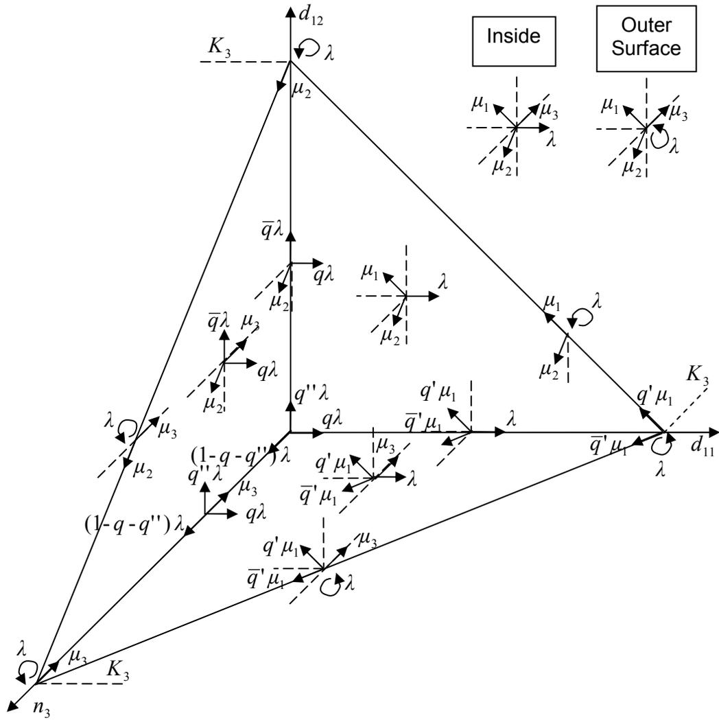
Figure 3.12(a) State-Transition Diagram of the Submodel for  $d_2 = 0$ .
