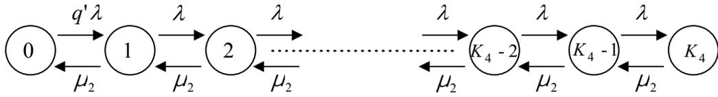
Figure M.5 State-Transition Diagram of the Partially Aggregated Model in Figure 3.16 with State Description  $d_{12}$ .
