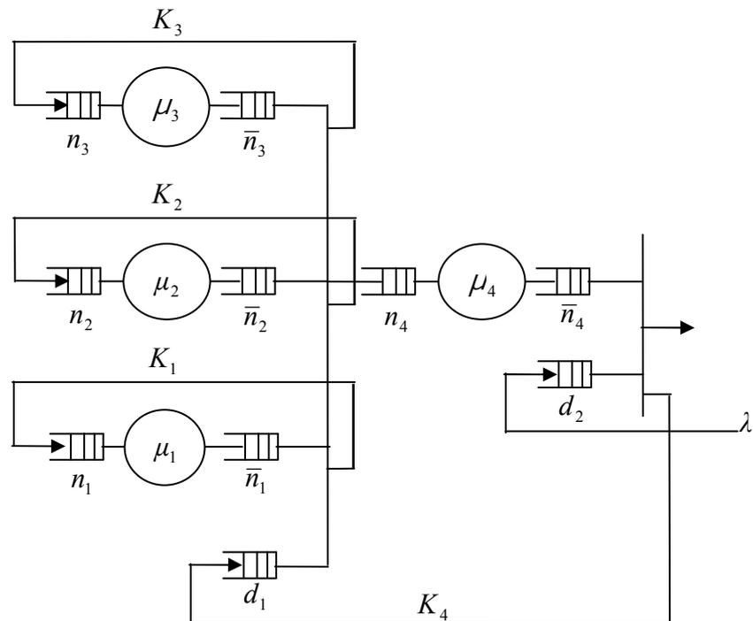
Figure M.1(a) Three-Component Assembly System with Simultaneous Release of Kanbans.
