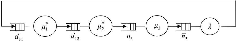
Figure 3.13(a) Equivalent Closed Network of the Submodel for  $d_2 = 0$
