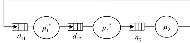
Figure 3.13(b) Equivalent Closed Network of the Submodel for  $d_2 > 0$ .
