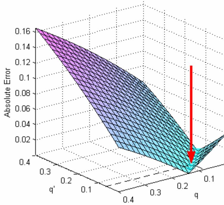
Figure 4.3 (a) Absolute errors for FR in the combined model of SKCS with  $\rho_i = 0.5$ ,  $K_i = 3$ ,  $i = 1, 2, 3$ .
