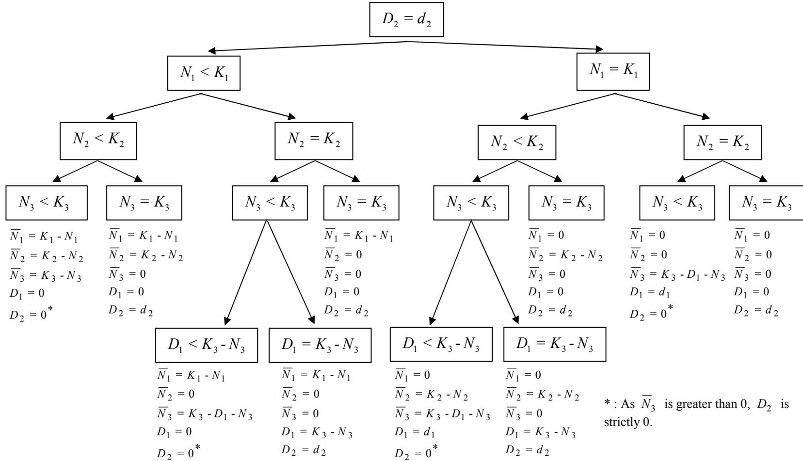
Figure A.1 Tree Structure of the Relations in the Original Model of SKCS with state description  $(n_1, n_2, n_3, d_1, d_2)$
