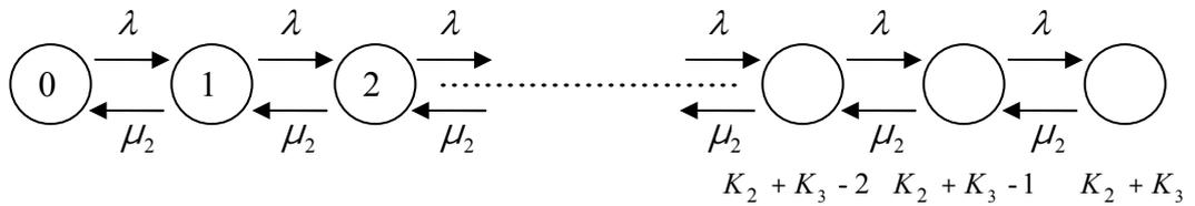
Figure 3.17 State-Transition Diagram of the Model in Figure 3.16 with State Description  $m_2$ .
