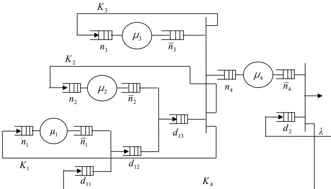
Figure M.2(a) Alternative Model for the Simultaneous Assembly Kanban System.
