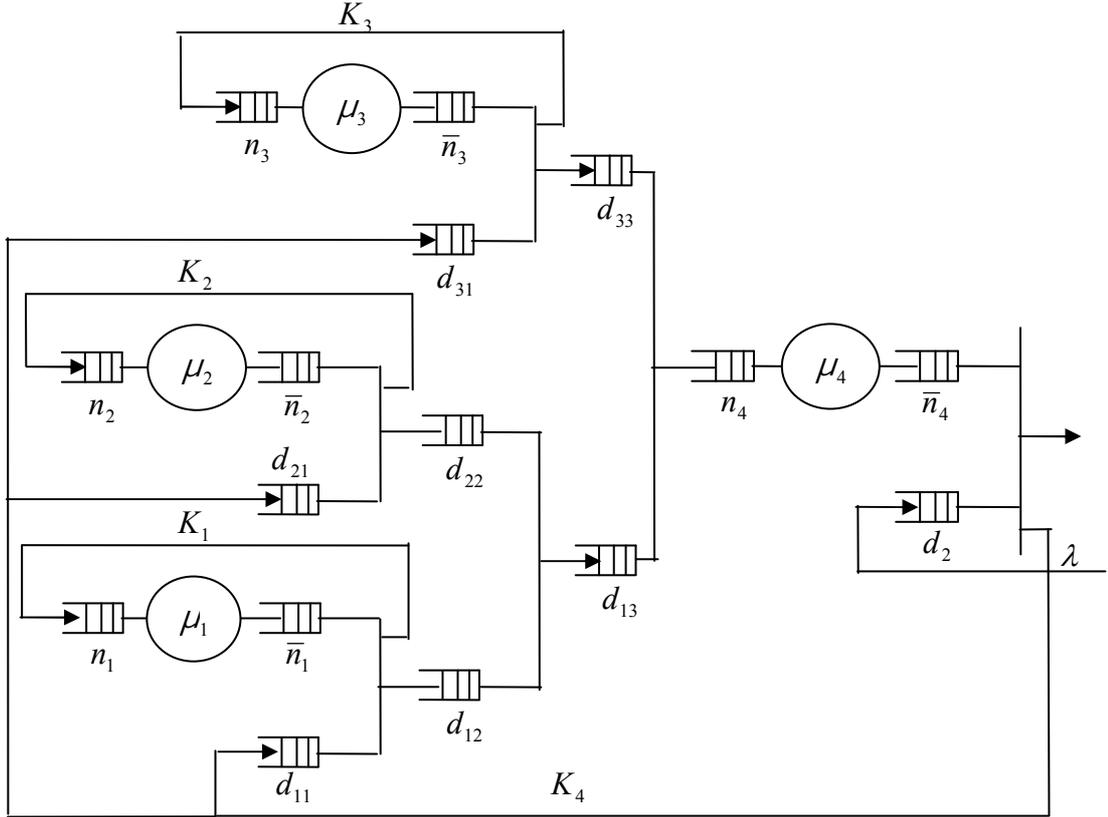
Figure M.2(b) Alternative Model for the Independent Assembly Kanban System.
