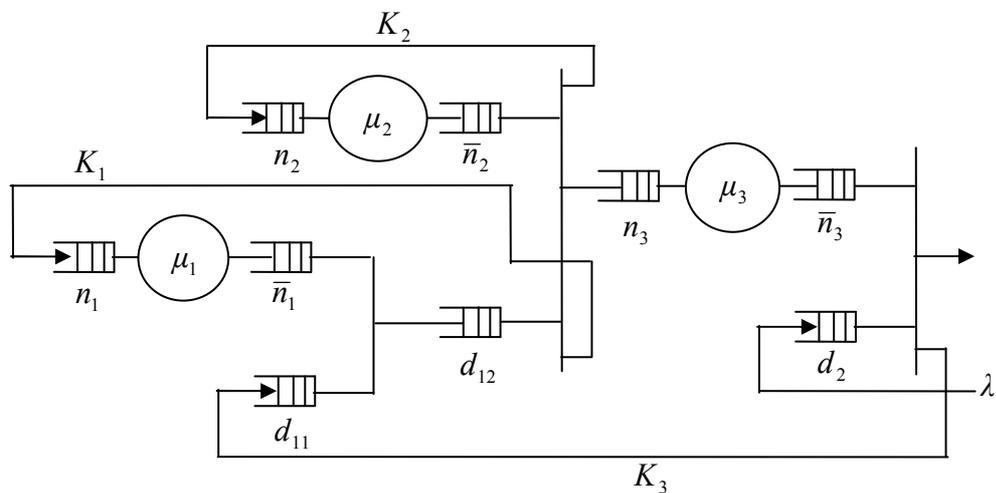
Figure 3.2 Alternative Model for the Simultaneous Kanban Control System.
