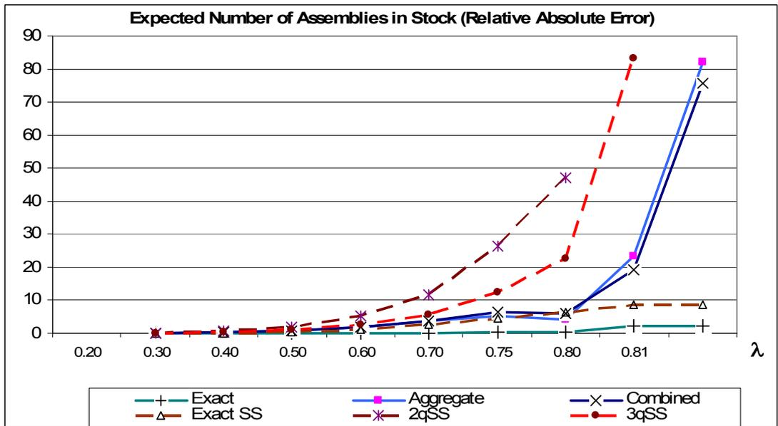
Figure 4.4 (b) Errors for expected number of assemblies in stock for SKCS with  $K_1 = 3, K_2 = 3, K_3 = 5$ .
