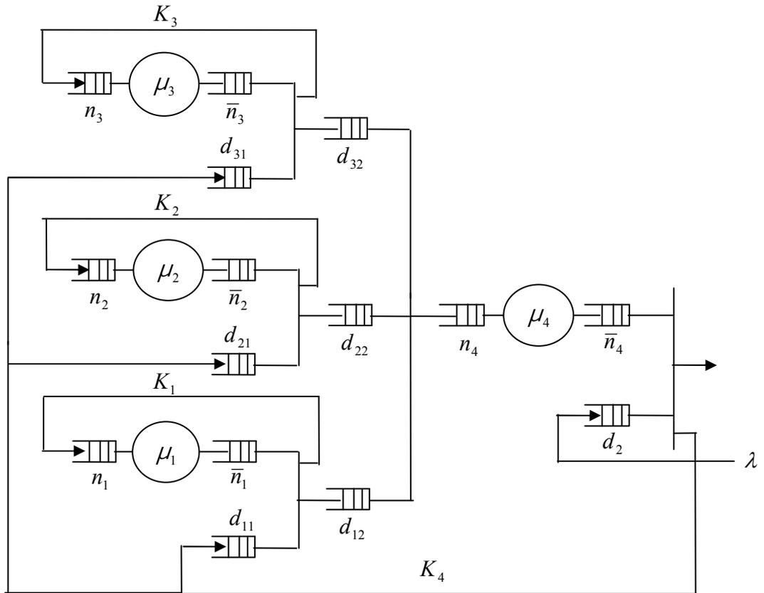
Figure M.1(b) Three-Component Assembly System with Independent Release of Kanbans.
