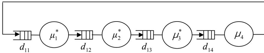
Figure M.3(b) Equivalent Closed Network of the Submodel for  $d_2 > 0$ .
