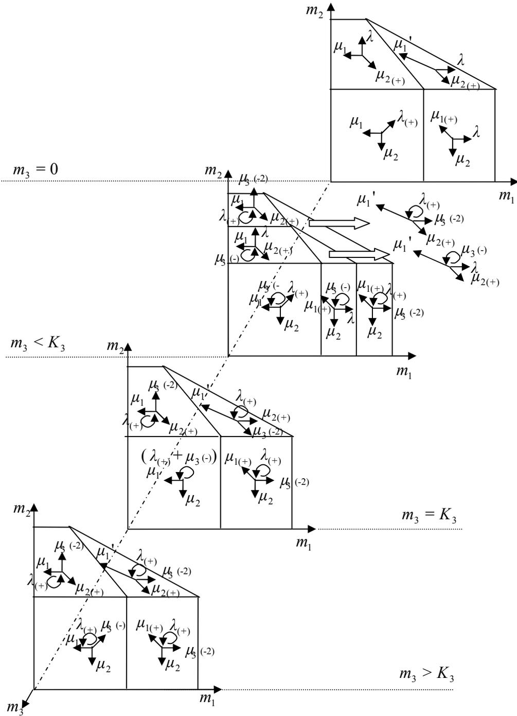
Figure 3.3 Cross-Sections of the State-Transition Diagram for the Model with State Description  $(m_1, m_2, m_3)$ .
