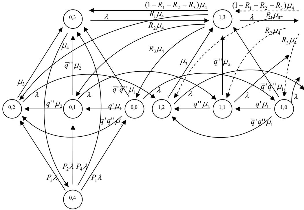
Figure M.4 Transition Diagram of the Combined Model for Three-Component System.
