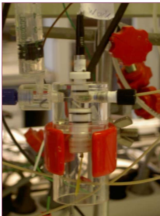
**Figure 2.2.** Constructed four-electrode flow cell
