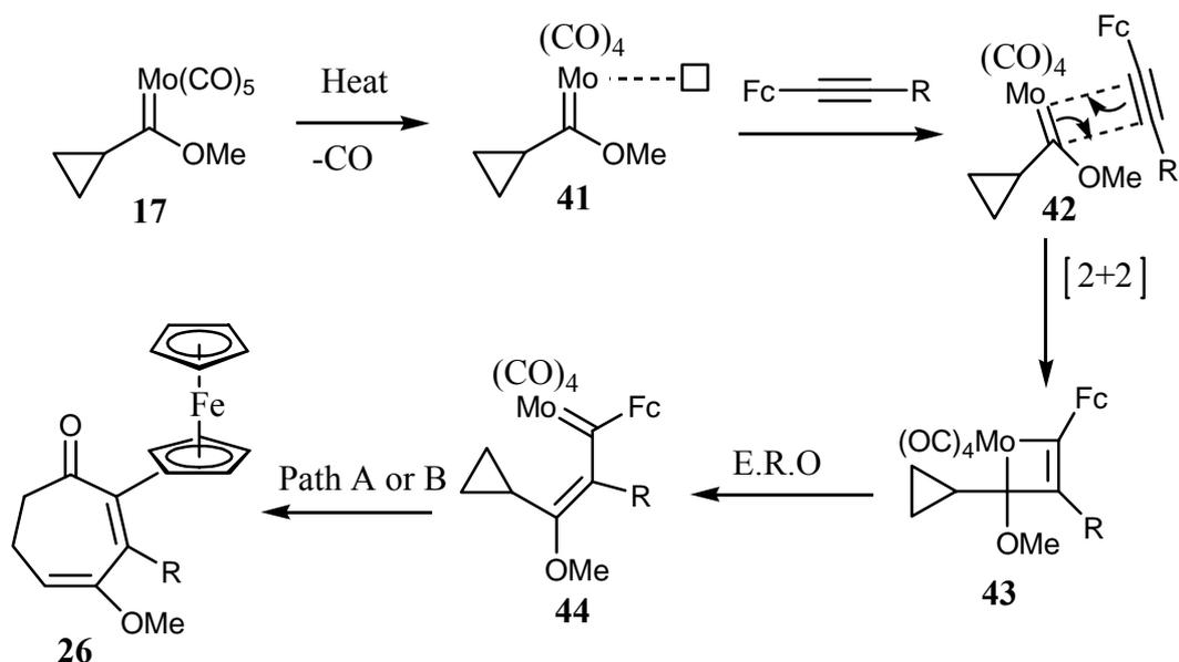
**Figure 36.** Proposed mechanism for the reaction of carbene complex **17** with ferrocenyl alkynes **25**
