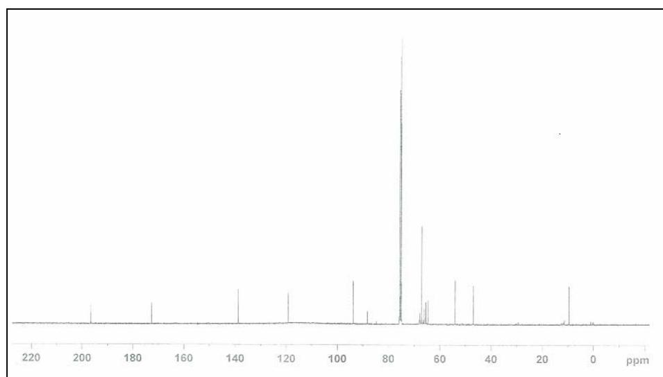
**Figure A8.** <sup>13</sup>C-NMR Spectrum of ferrocenyl cycloheptadienone **28B**
