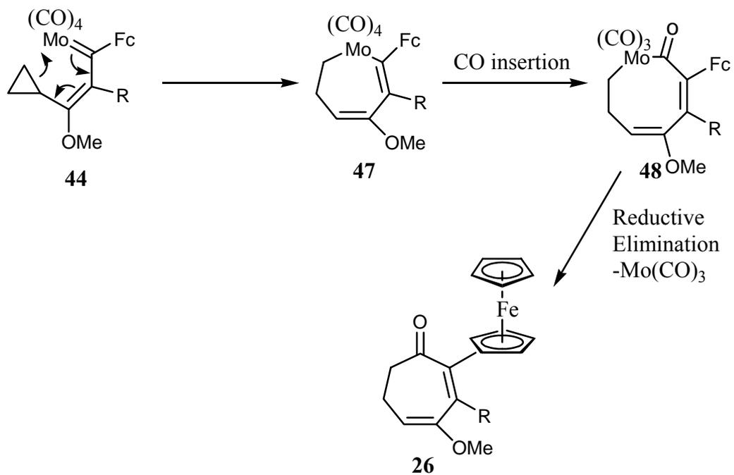
**Figure 38.** Proposed mechanism for the formation of cycloheptadienone **26** via Path B
