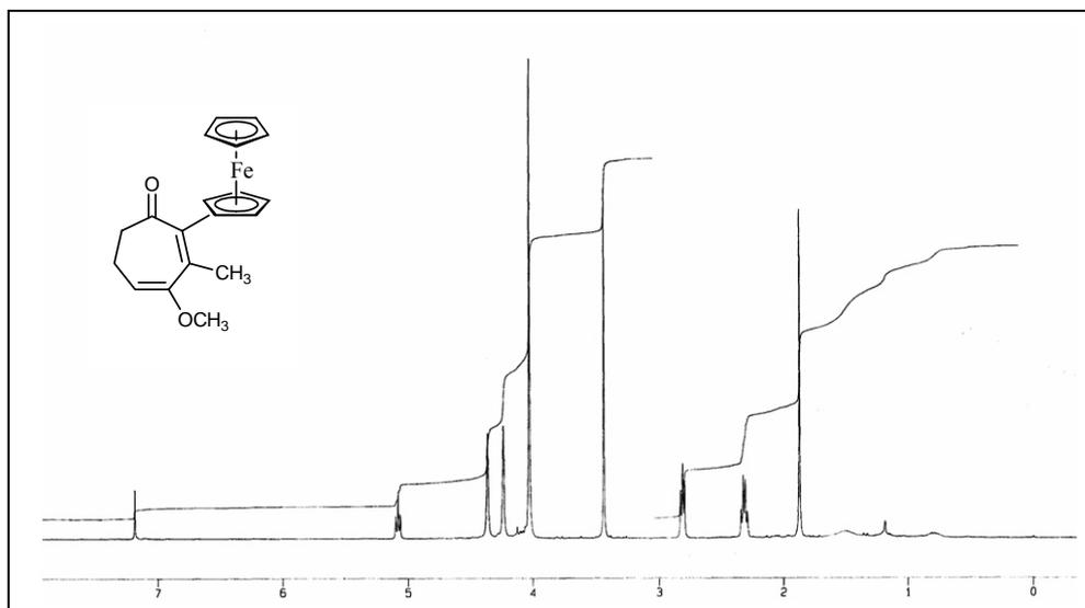
**Figure A1.** <sup>1</sup>H-NMR Spectrum of ferrocenyl cycloheptadienone **26B**
