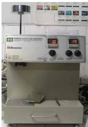
**Figure 3.11** Omega Melt Flow Indexer
