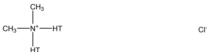
**Figure 3.1** Chemical structure of organic modifier (2M2HT<sup>+</sup>) and anion (Cl<sup>-</sup>) of Cloisite® 15A.
