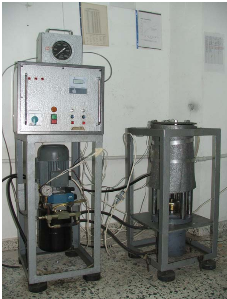
Figure A.1. The High Hydrostatic Pressure Unit.
