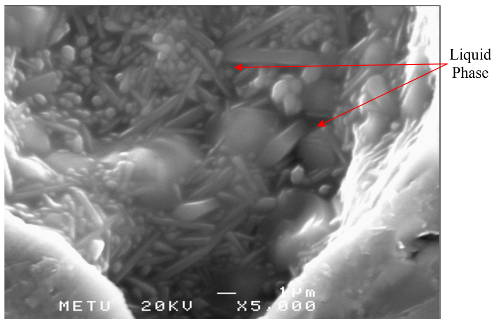
Figure 4.29 The SEM micrograph of the HAP + wollastonite ceramic sintered with 15 wt% NCAS frit.
