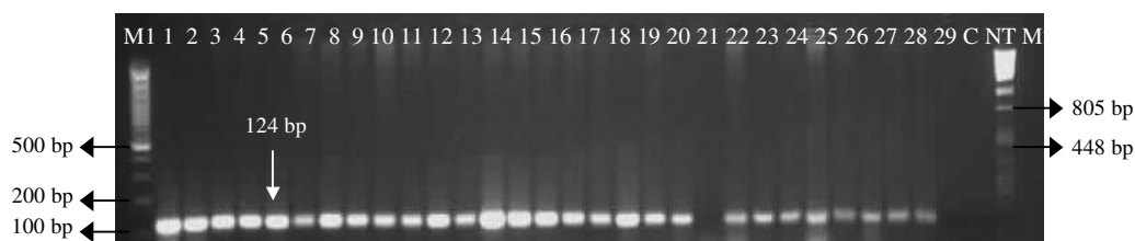
Figure 3.1; Patatin specific PCR results: line M1; 100bp molecular weight marker, line 1-29 samples, line C; negative control maize DNA, line NT; no template, line M2; pst I digested lambda ( \lambda ) DNA
