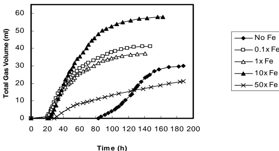
**Figure 3.8 Total volume of hydrogen gas production for various concentrations of Iron**
