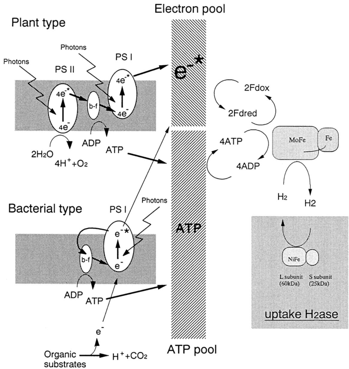
**Figure 1.2 Mechanism of light to hydrogen conversion by photosynthetic bacteria (Miyake *et al.*, 1999)**
