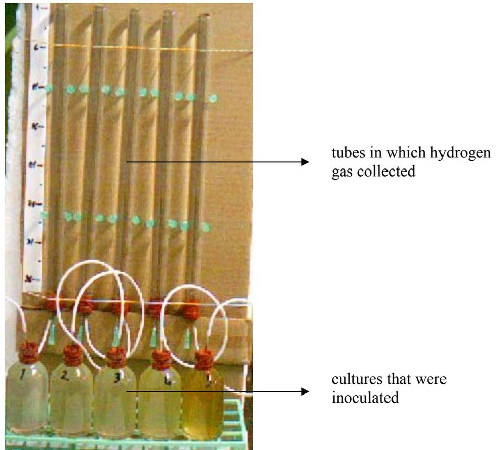
**Figure 2.1 Experimental set up for hydrogen growth**
