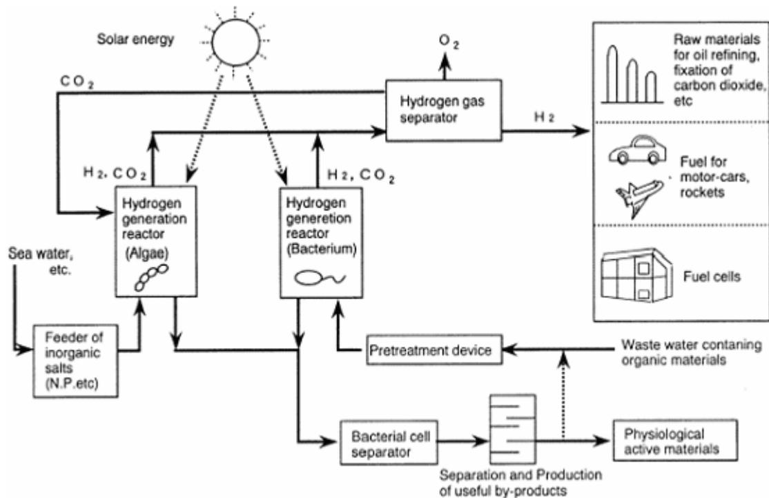
**Figure 1.1 Concept of biological hydrogen production and utilization. (Miyake et al., 1999)**
