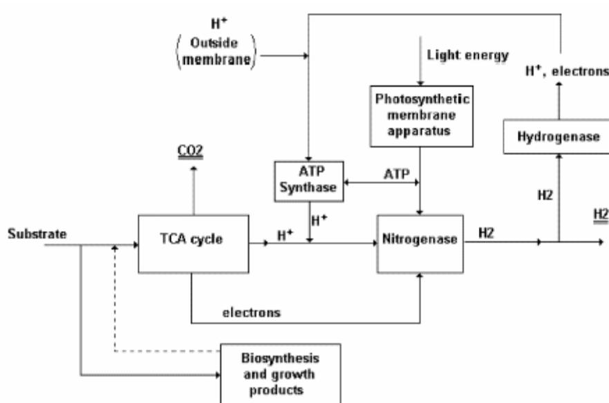
**Figure 1.7** The overall scheme of hydrogen production by PNS bacteria (Koku *et al.*, 2002)
