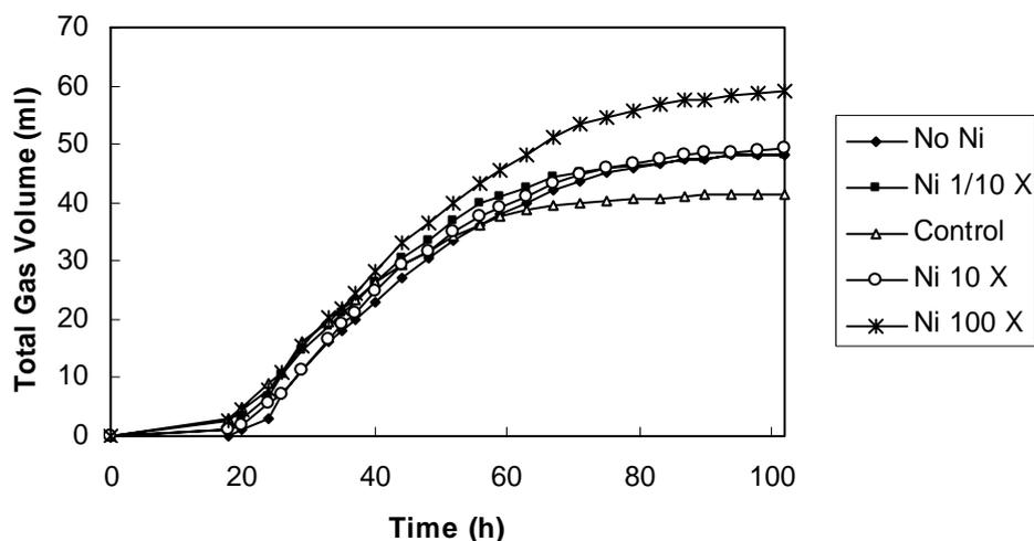
**Figure 3.7 Hydrogen gas production at various concentrations of nickel ion**
