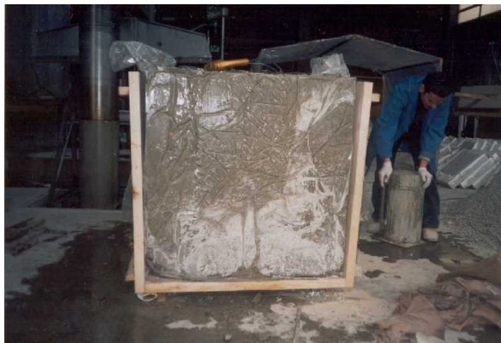
Figure 3.17. The specimens could be taken out easily by removing only one face of the modular formwork
