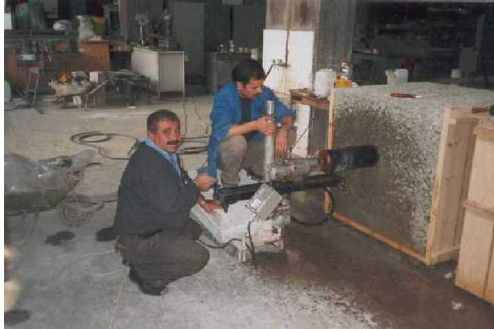
Figure 3.4. One of the three core specimens, which have been located as shown at Figure 3.3, is being taken (the one that belongs to portion 2 according to Figure 3.3)
