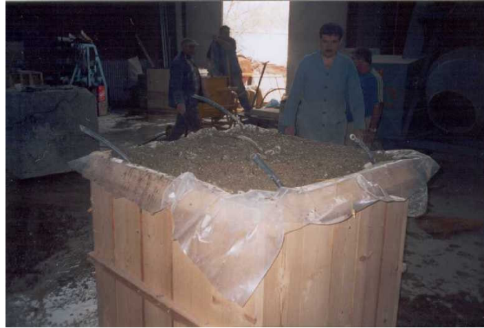
Figure 3.13. The length of the insert pipes were chosen in such a way that an extension of 20-30 cm was obtained above the surface of the aggregate mass
