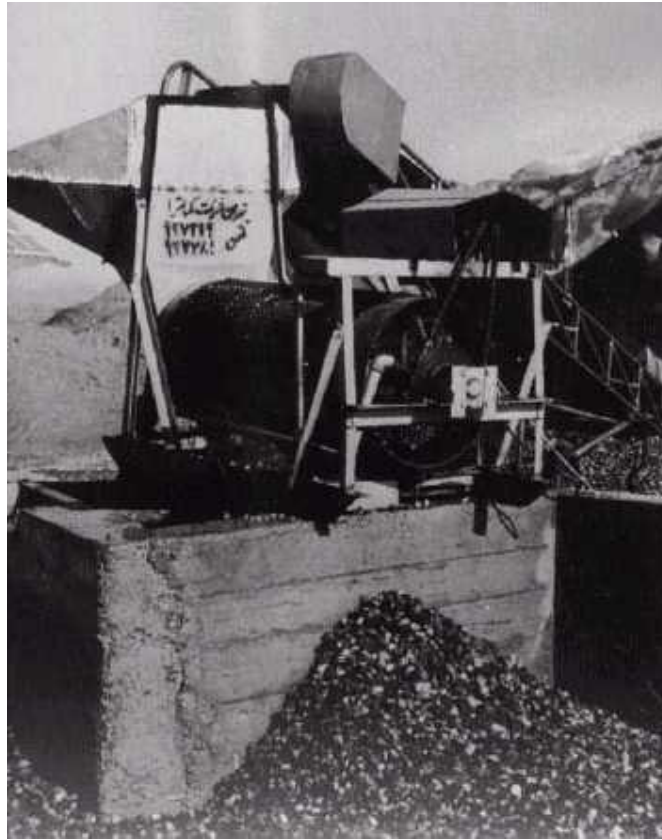
Figure 2.7. The coarse aggregates are being washed by rotary screen in order to remove the undersize particles
