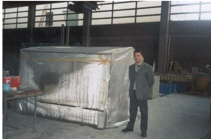
Figure 3.2. The tent which was used as a portable curing room for the huge concrete specimens
