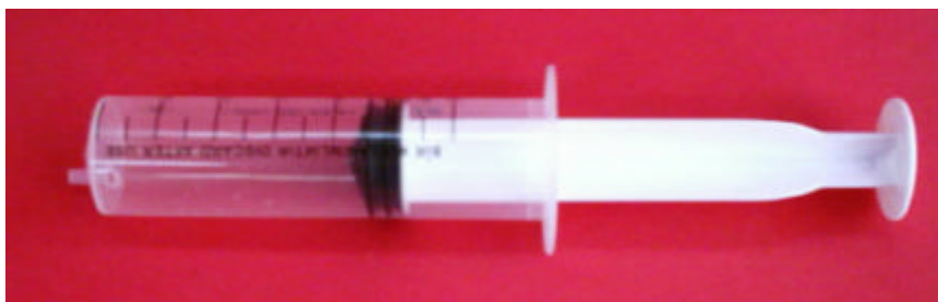
Figure G.1 Syringe filled with air before compression.
