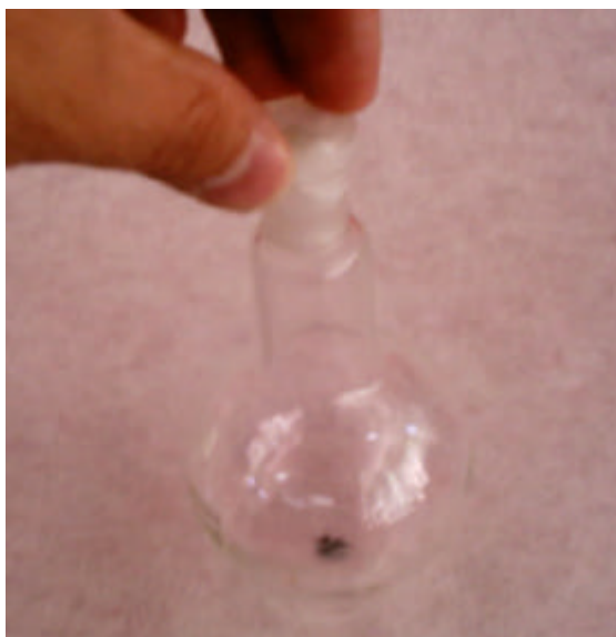
Figure H.1 Flask with solid iodine before heating.
