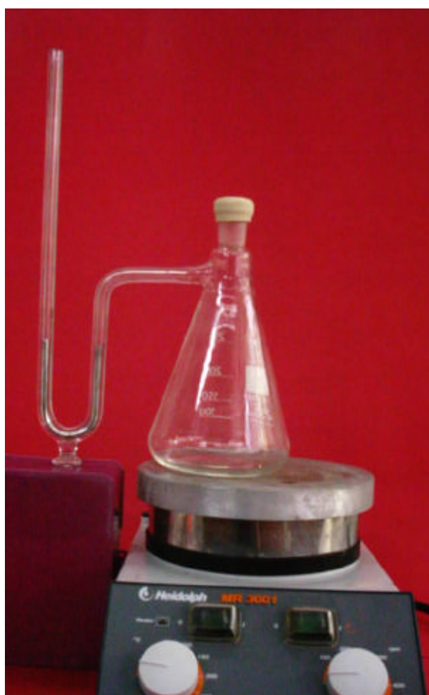
Figure K.1 Mercury levels of the manometer are equal before heating.
