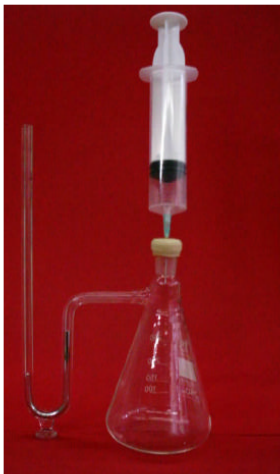
Figure L.2 Mercury levels of the manometer are not equal after evacuating some amount of air.
