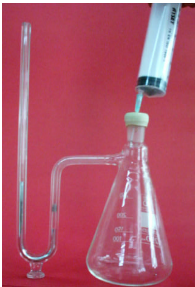
Figure L.3 Mercury levels of the manometer are not equal after adding some amount of air.
