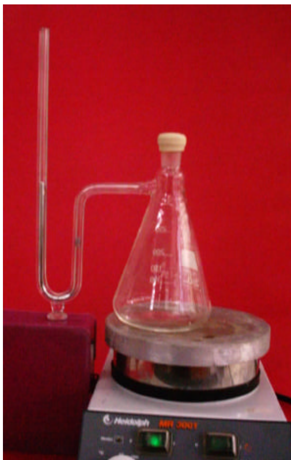
Figure K.2 Mercury levels of the manometer are not equal after heating.
