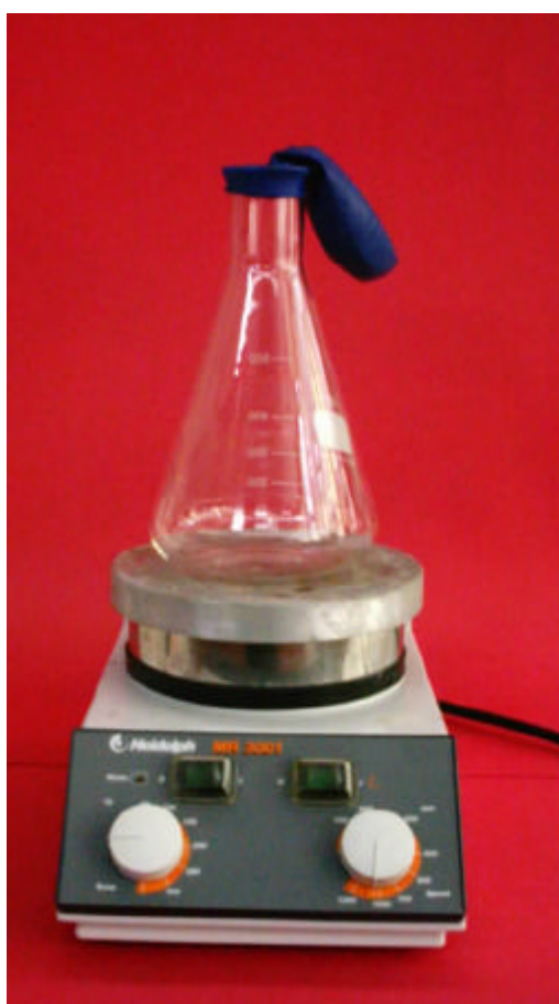
Figure I.1 Flask filled with air before heating.
