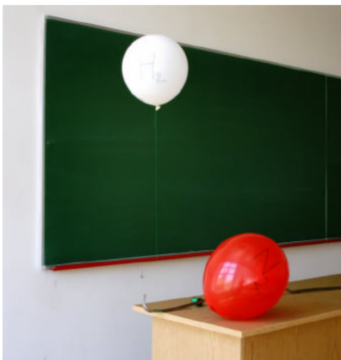
Figure J.1 Balloon filled with hydrogen rose when balloon filled with nitrogen fell to the floor.
