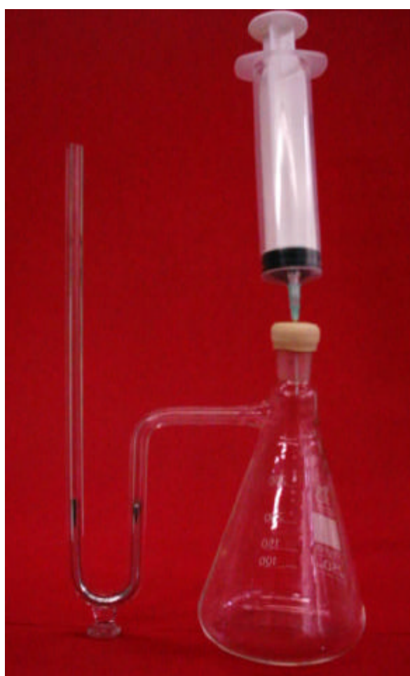
Figure L.1 Mercury levels of the manometer are equal before adding air.
