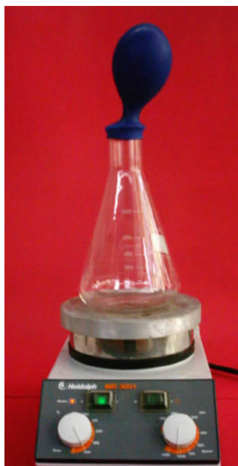
Figure I.2 Flask filled with air after heating: the balloon inflated.
