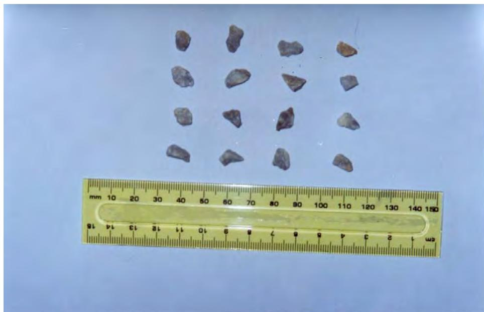
Figure 4.7 Limestone particles retained on 4.75 mm sieve size
