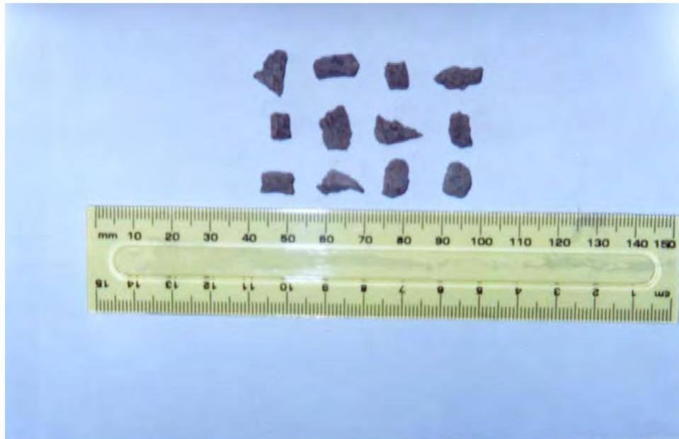
Figure 4.16 Steel-slag particles retained on 4.75 mm sieve size
