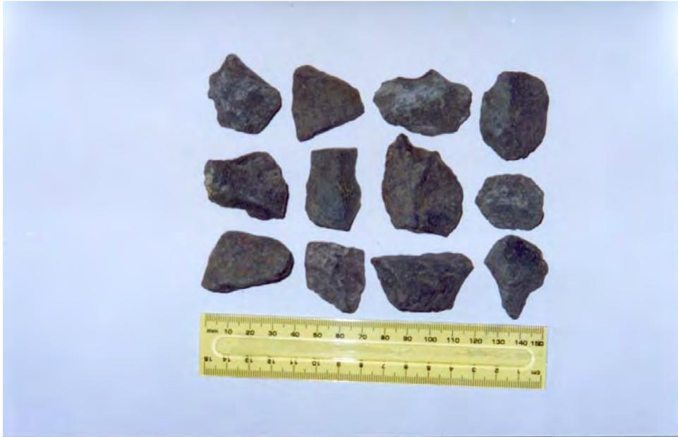
Figure 4.14 Basalt particles retained on 12.7 mm sieve size
