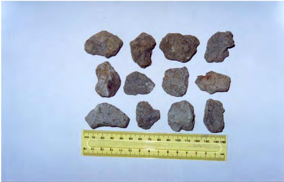
Figure 4.19 Steel-slag particles retained on 12.7 mm sieve size
