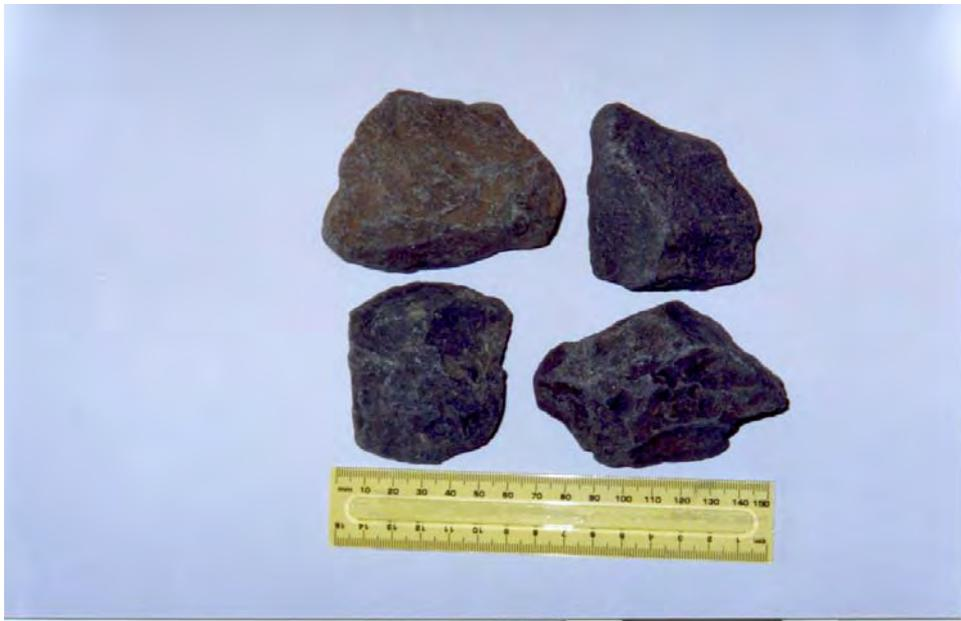
Figure 4.15 Basalt particles retained on 38.0 mm sieve size (prototype)
