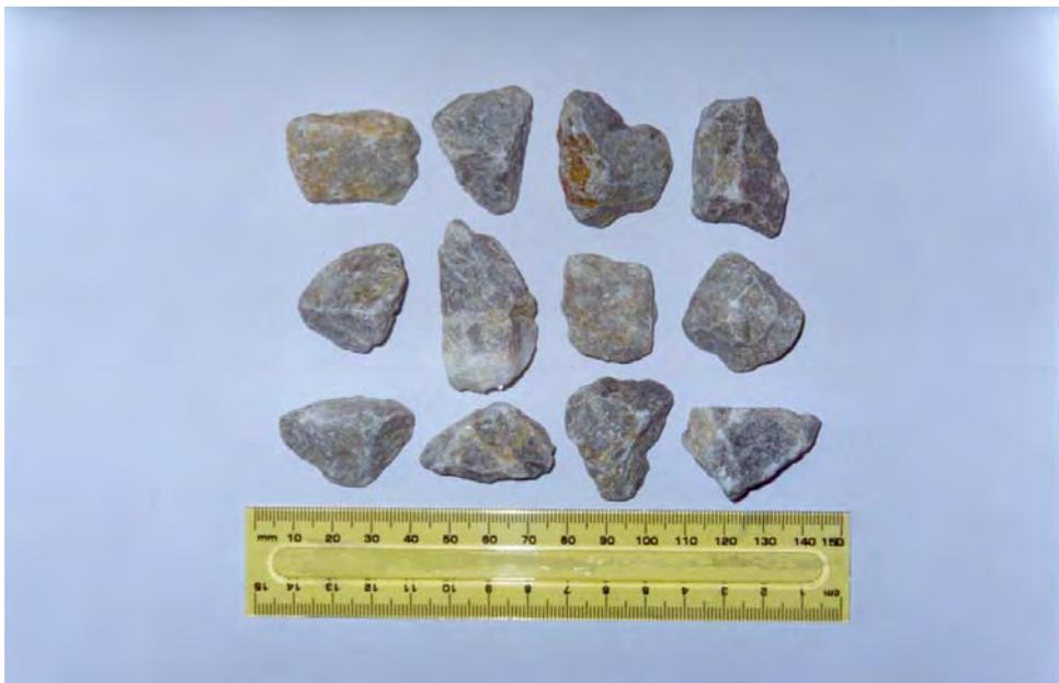
Figure 4.9 Limestone particles retained on 12.7 mm sieve size
