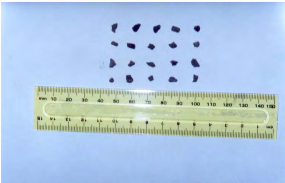
Figure 4.11 Basalt particles retained on 2.36 mm sieve size
