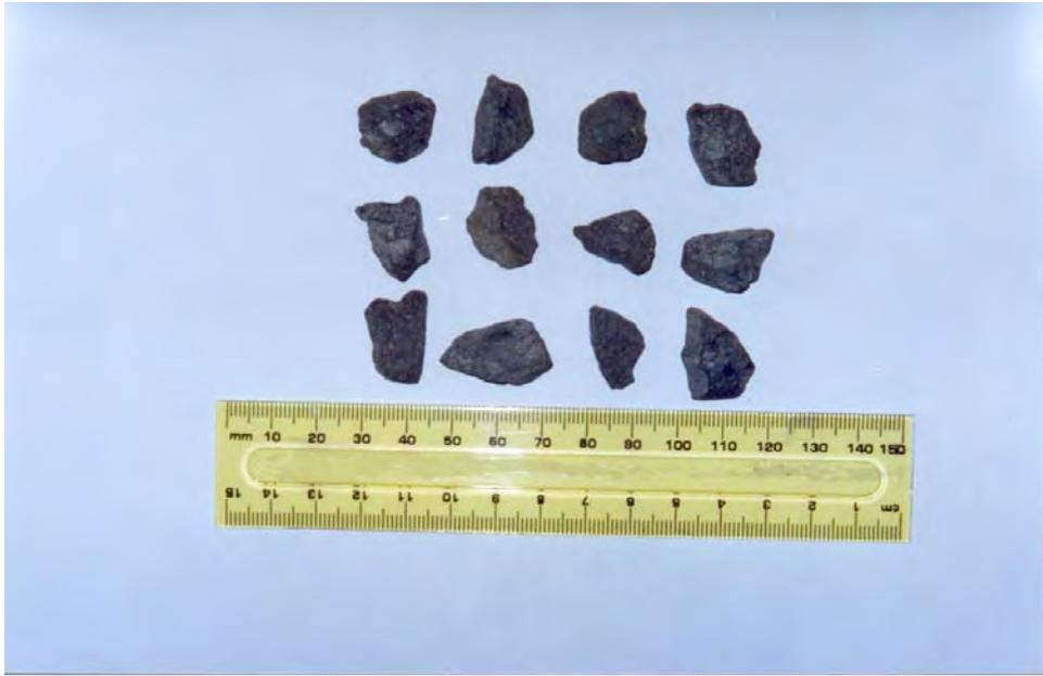
Figure 4.13 Basalt particles retained on 9.5 mm sieve size
