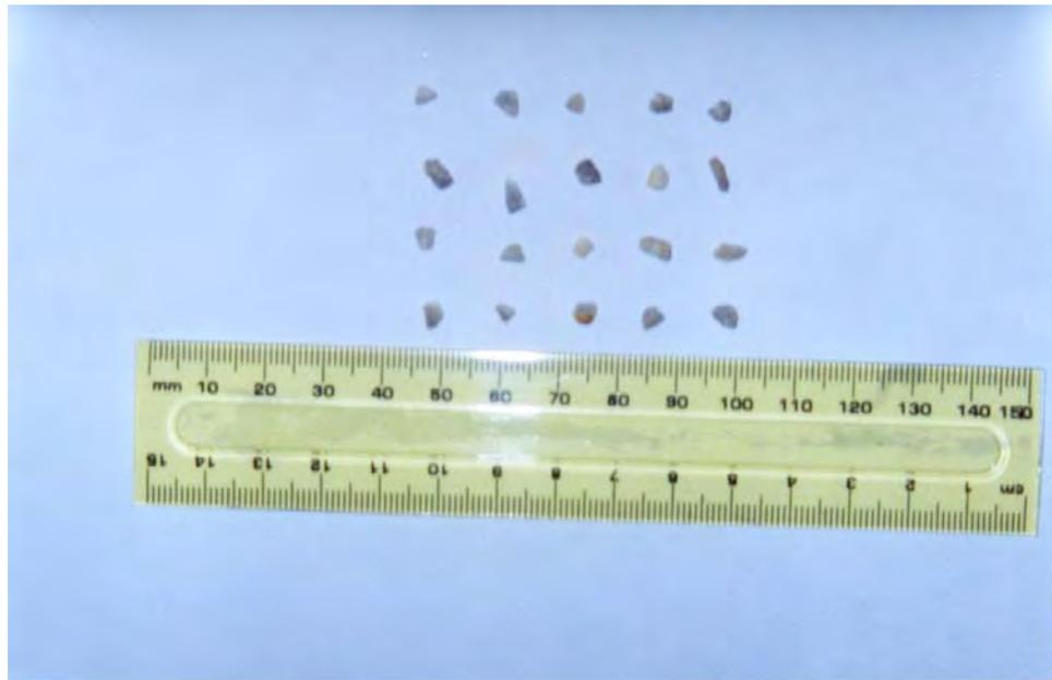
Figure 4.6 Limestone particles retained on 2.36 mm sieve size
