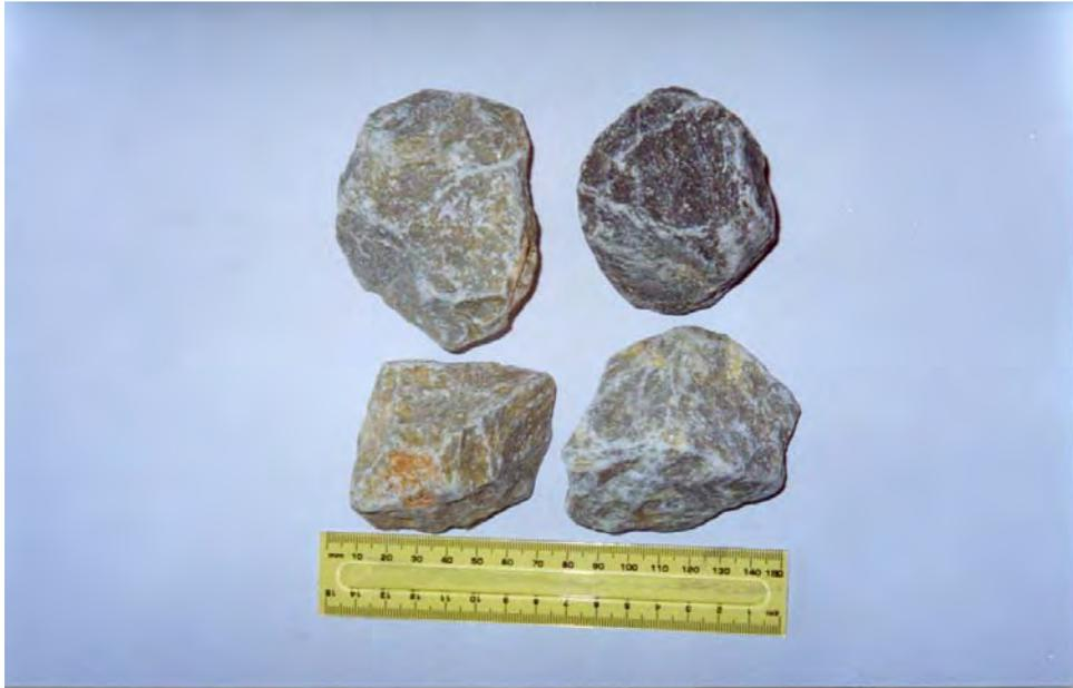
Figure 4.10 Limestone particles retained on 38.0 mm sieve size (prototype)
