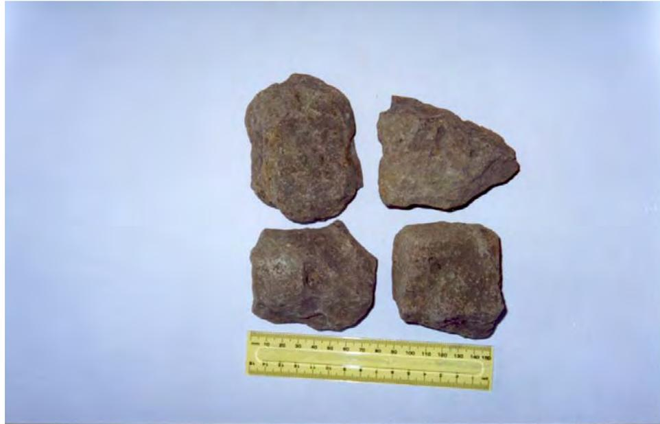
Figure 4.20 Steel-slag particles retained on 50.0 mm sieve size (prototype)
