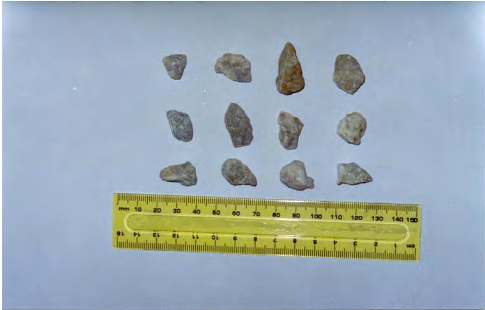
Figure 4.8 Limestone particles retained on 9.5 mm sieve size
