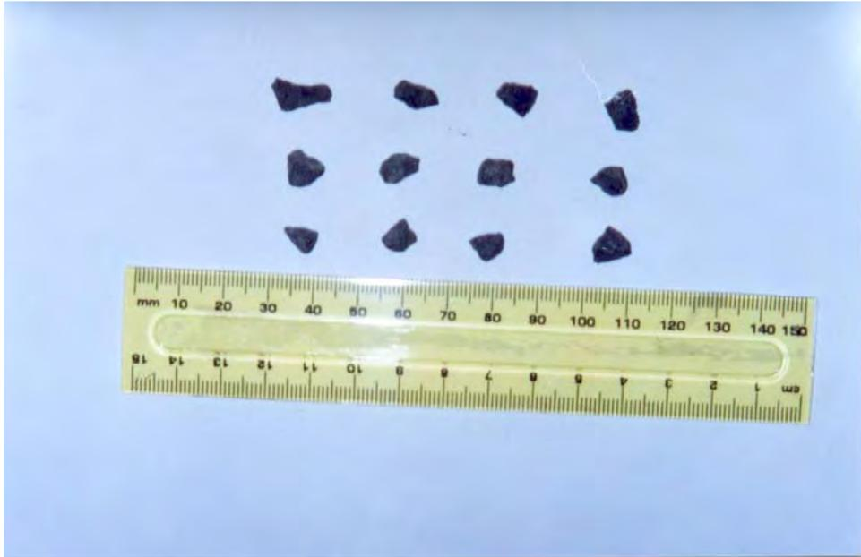
Figure 4.12 Basalt particles retained on 4.75 mm sieve size
