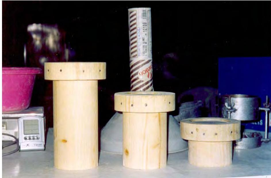
Figure 4.22 Special wooden blocks to compact each layer of specimen
