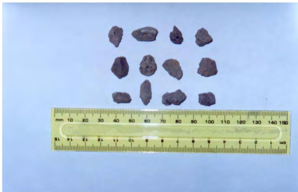
Figure 4.17 Steel-slag particles retained on 6.35 mm sieve size
