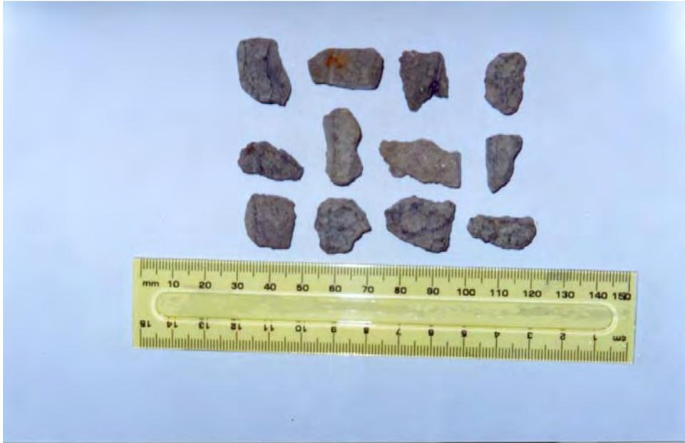
Figure 4.18 Steel-slag particles retained on 9.5 mm sieve size
