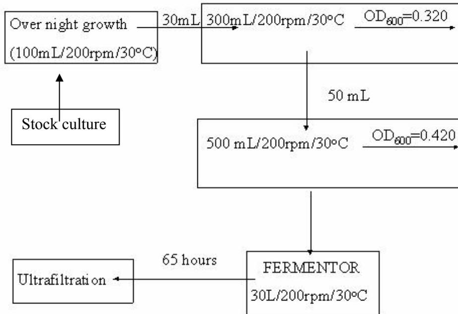
**Figure 2.1.** Schematic description of inoculum preparation, fermentation and downstream.
