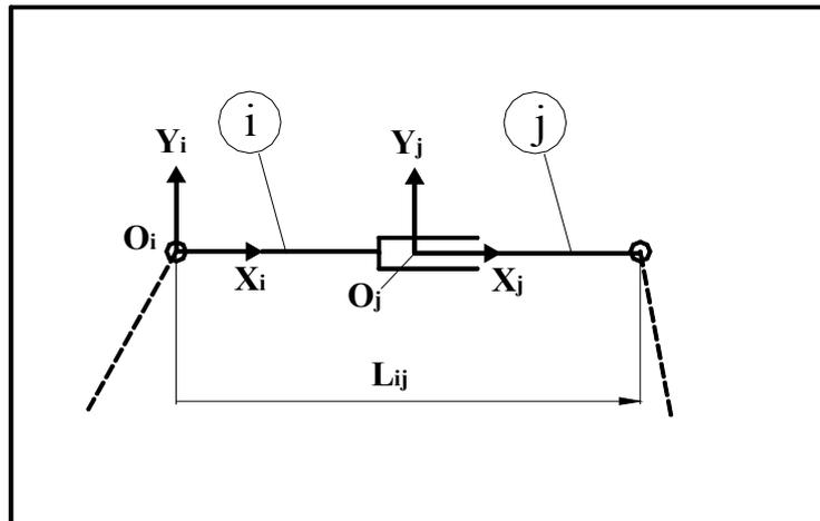
Figure 2.2 Link i of a Kinematically Adjustable Mechanism
