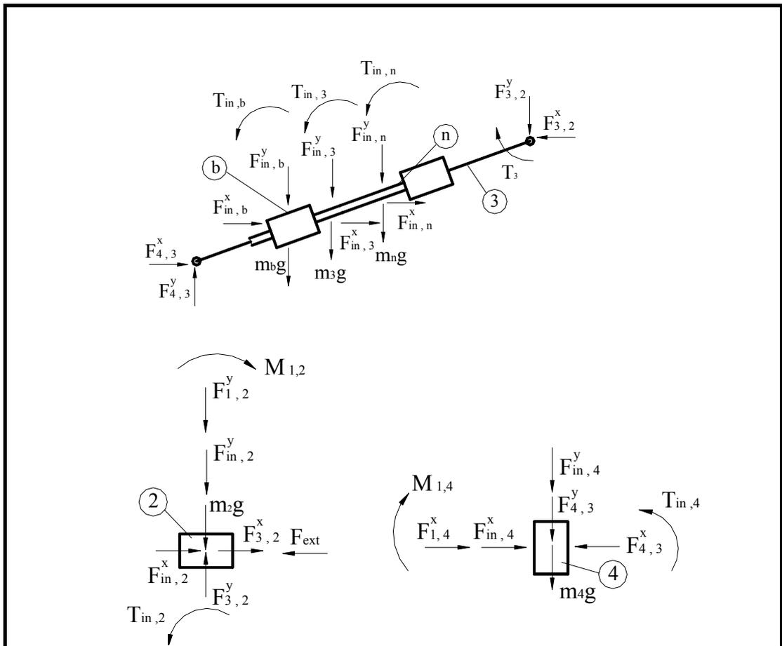
Figure 4.2 Free-body Diagrams of the Dynamically Adjustable OET
