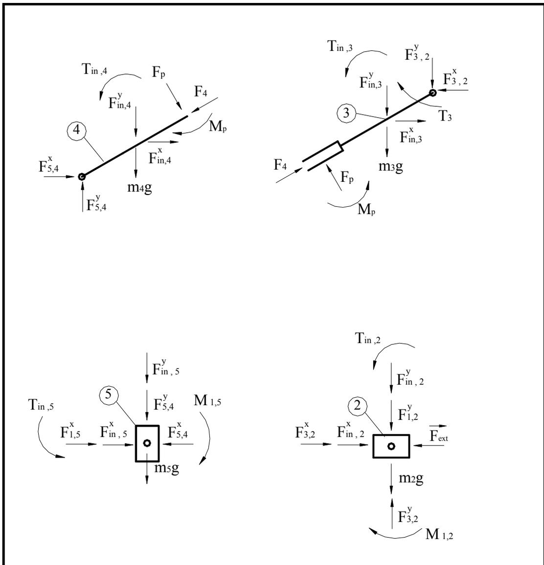
Figure 4.31 Free body diagrams of the Kinematically Adjustable OET
