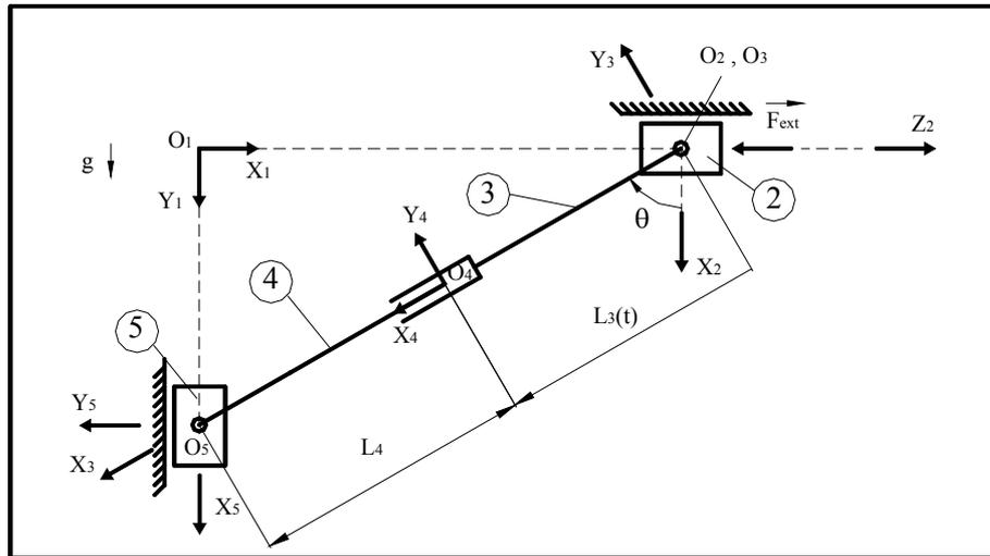
Figure 4.30 The Kinematically Adjustable Oscillating Elliptic Trammel
