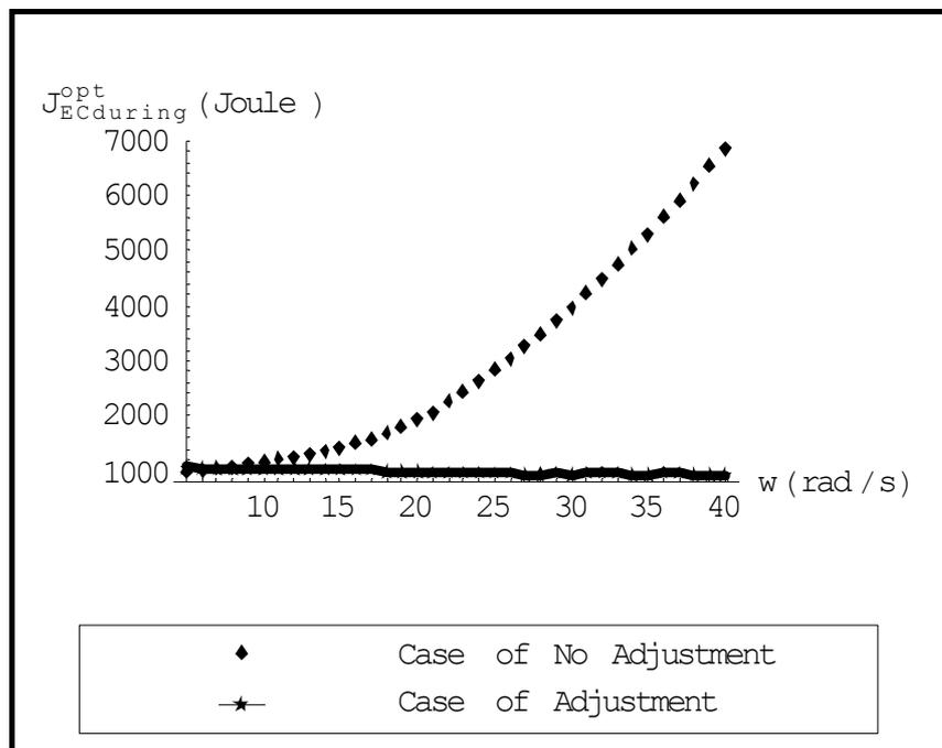
Figure 4.23 Variation of  $J_{ECduring}^{opt}$  with respect to  $\omega$
