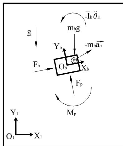
Figure 2.15 Free body diagram of the moving block
