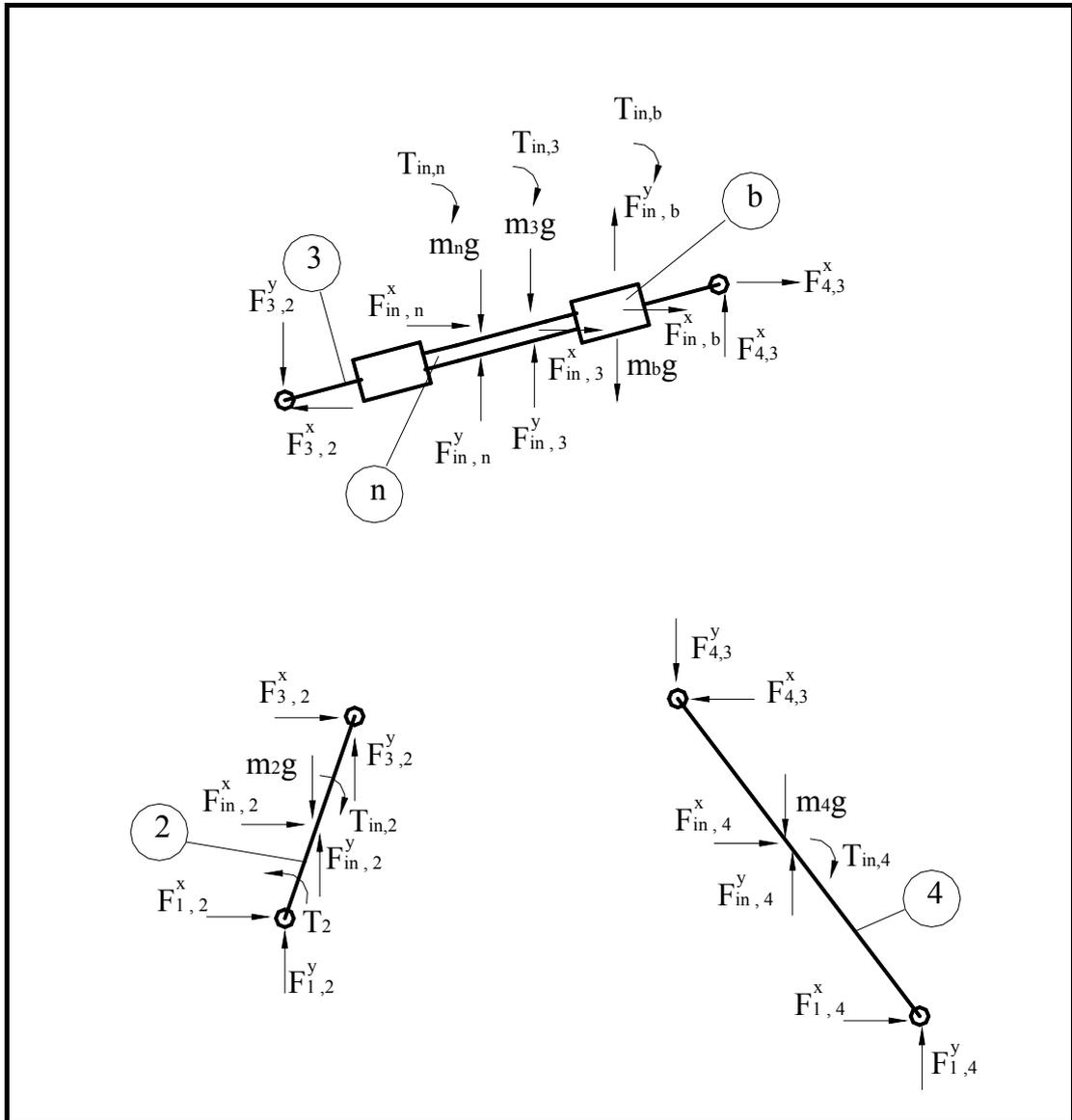
Figure 4.42 Free body diagrams of the Adjustable Fourbar Mechanism
