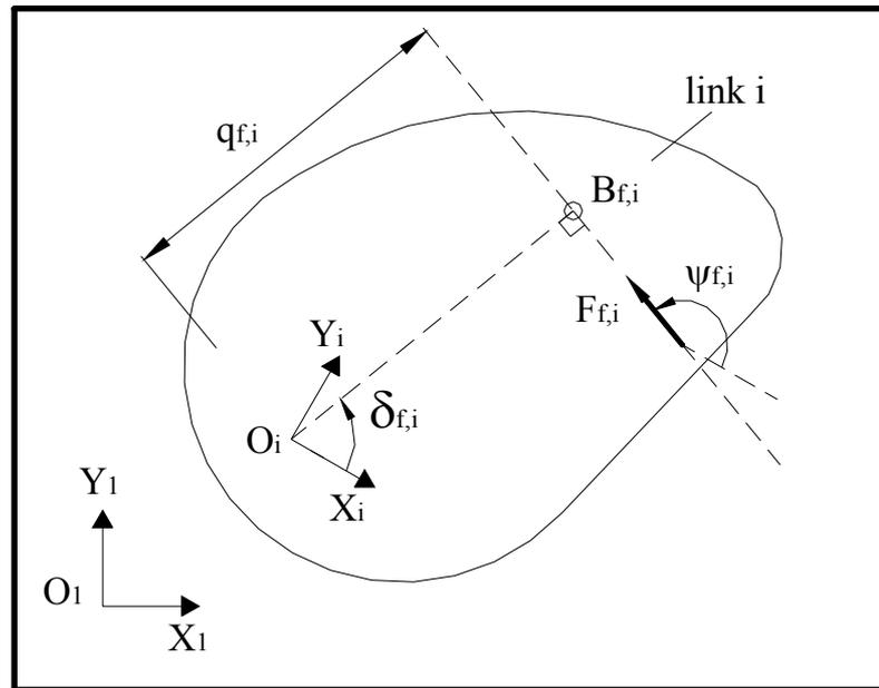
Figure 2.8  $f$ 'th externally applied force acting on link  $i$
