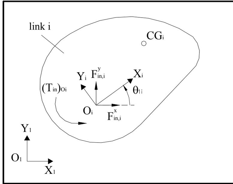
Figure 2.12 Inertia force system acting at  $O_i$
