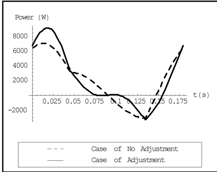
Figure 4.35 Variation of power with respect to time for  $\omega = 35$  rad/s
