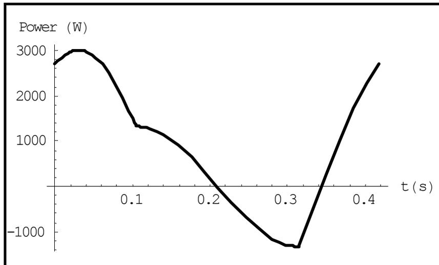
Figure 4.34 Variation of power with respect to time for  $\omega = 15 \text{ rad/s}$
