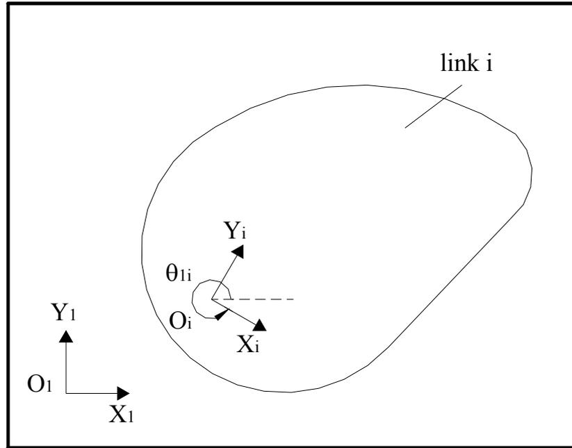
Figure 2.3 Body fixed and inertial coordinate systems
