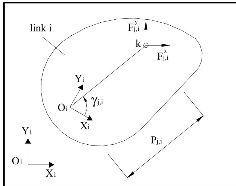
Figure 2.4 Revolute joint reaction on link i
