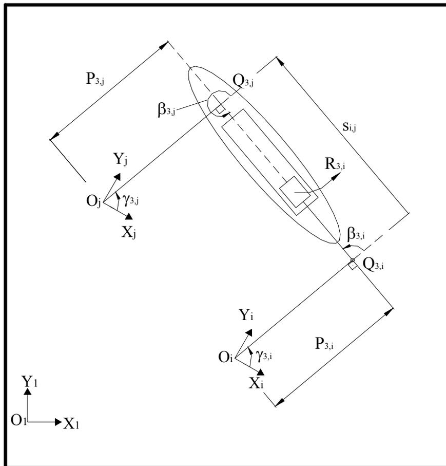
Figure 2.7 Prismatic joint number 3 connecting links  $i$  and  $j$
