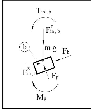
Figure 4.3 Free-body diagram of the moving block
