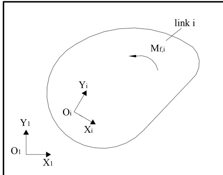
Figure 2.9  $m$ 'th externally applied moment acting on link  $i$
