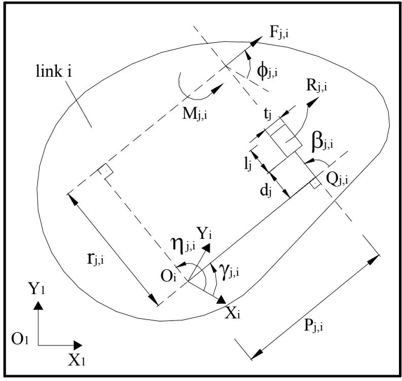
Figure 2.5 Slider ( numbered j ) on link i
