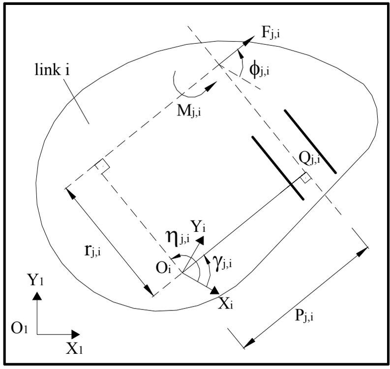
Figure 2.6 Slot ( numbered j ) on link i
