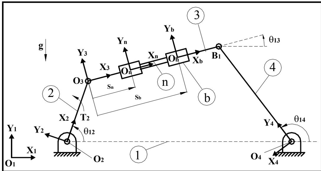
Figure 4.41 The Dynamically Adjustable Fourbar Mechanism
