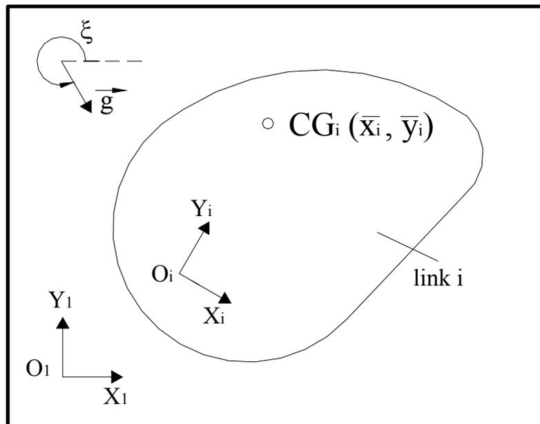
Figure 2.10 Coordinates of the center of gravity of link  $i$
