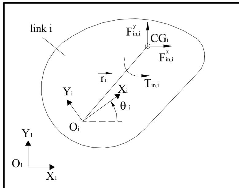
Figure 2.11 Inertia force system acting at  $CG_i$
