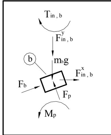
Figure 4.43 Free body diagram of the moving block
