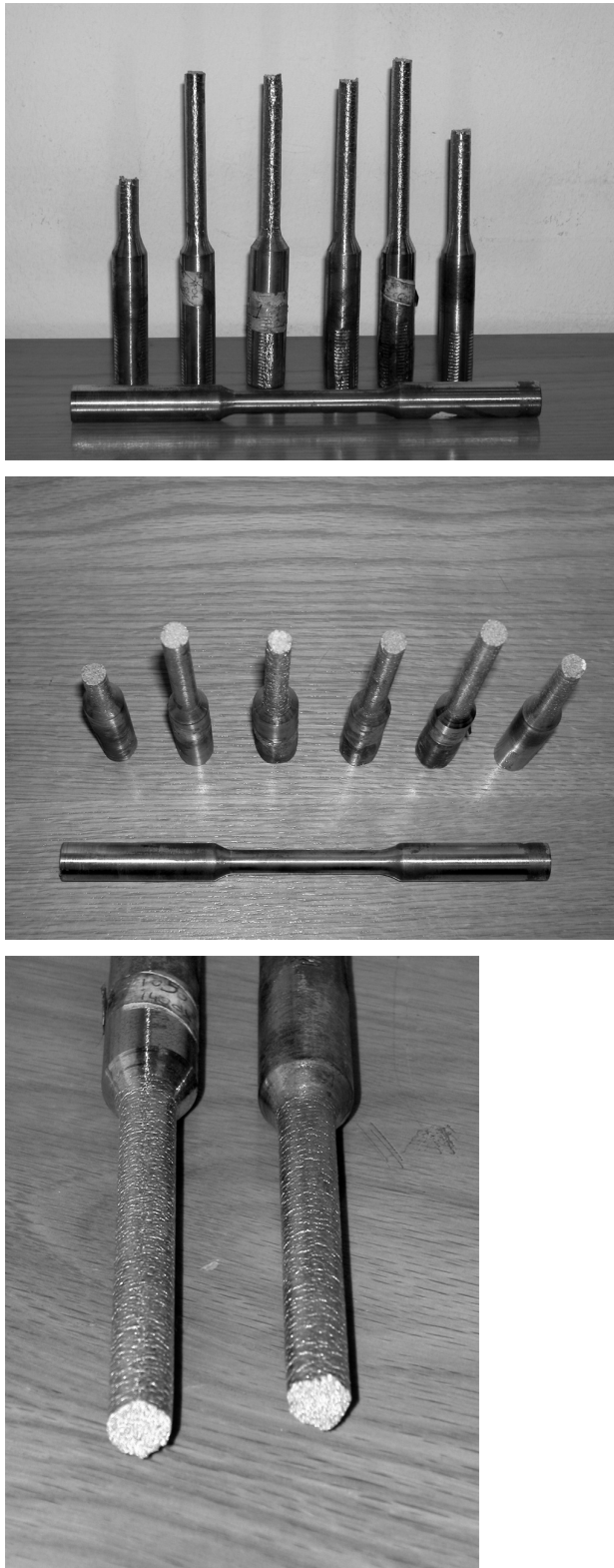
Fig. 4.7: Sample photographs of specimens after tensile test
