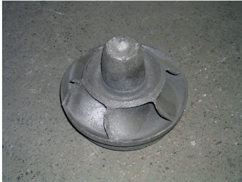
Figure A.3 – Photograph of impeller before machining
