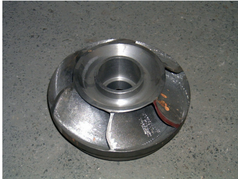
Figure A.4 – Photograph of impeller after machining
