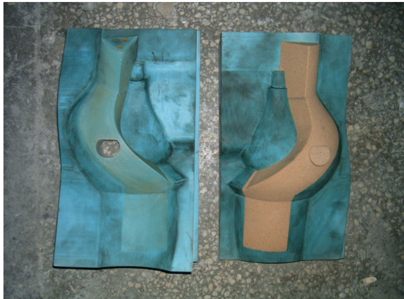
Figure A.2 – Photograph of bowl core and core box
