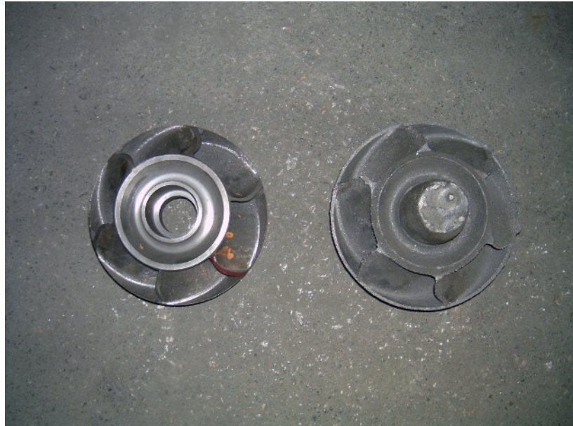
Figure A.5 – Photograph of impeller after and before machining from top view
