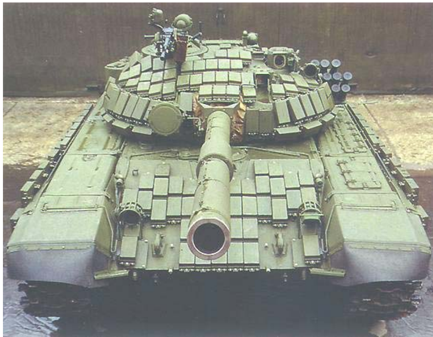
Figure 2-7 Russian T-72S MBT equipped with ERA packages, with different surface normal directions [23]
