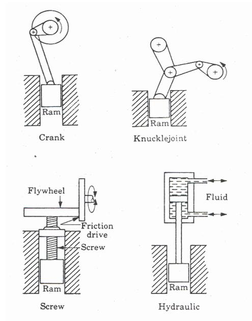
Figure 1.1 Schematic Illustration of Various Types of Presses Used in Forging [2]
