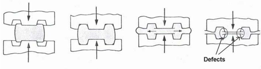
Figure 1.2 Internal Defects Because of an Oversized Billet in Forging
