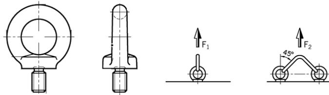
Figure 4.2 A Lifting Eye Bolt with Two Loading Configurations [28]
