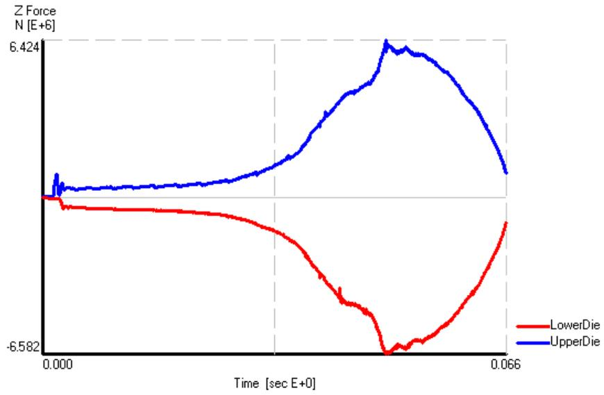
Figure 4.9 Die Load vs. Time Graph of C60 at 1150 °C
