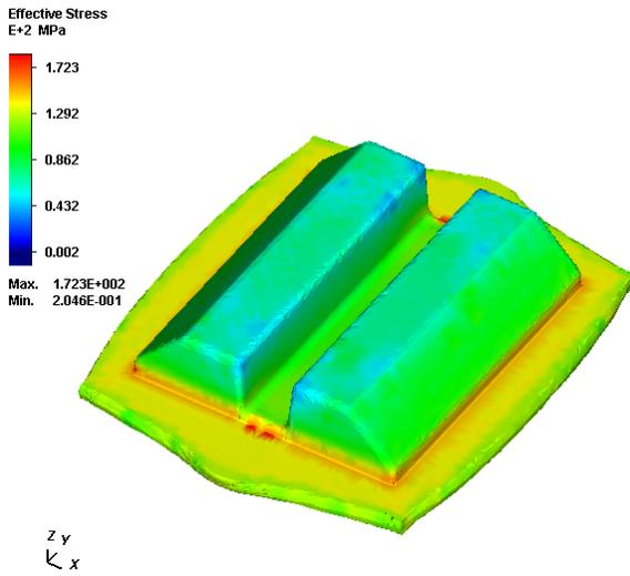
Figure 5.8 Effective Stress Distributions for Carbon Steel at 80 % of the Final Stroke
