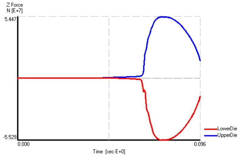
Figure 5.7 Die Loads in the Final Stage of Process for the Carbon Steel, C45
