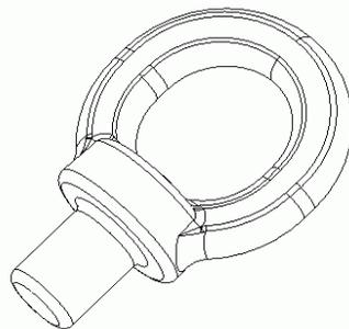
Figure 4.1 Forging Model of a High Tensile Eye Bolt
