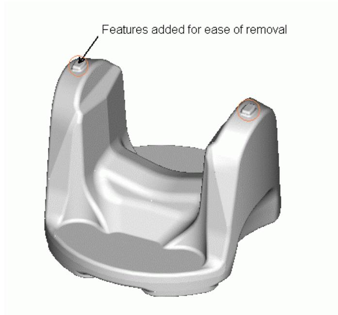
Figure 3.3 Addition of the Features to a Forging Model for Ease of Removal and not to Harm the Part
