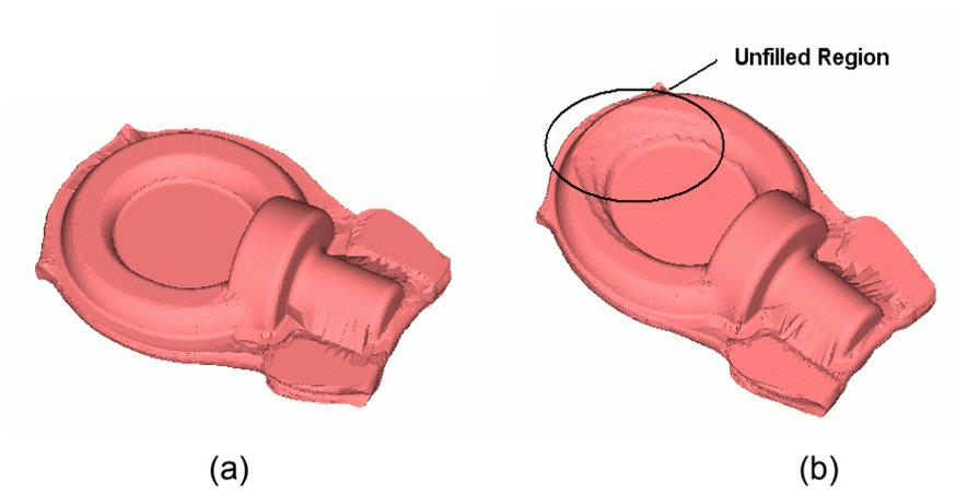
Figure 4.17 Final Product in Forging M30 Showing (a) Filled and (b) Unfilled Regions
