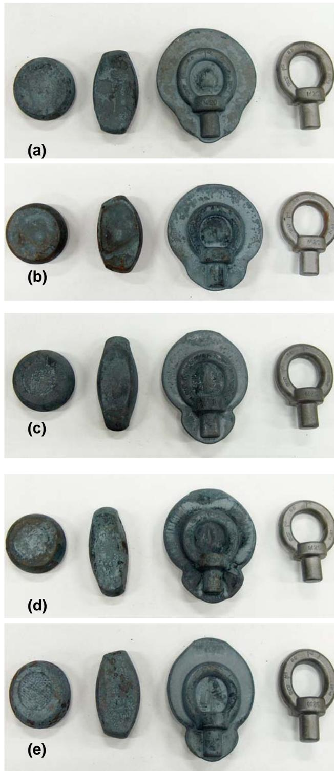
Figure 4.7 The Steps of the Forging Process of M20 Eye Bolt with Different Materials (a) C45 (b) C60 (c) X20Cr13 (d) 42CrMo4 (e) 100Cr6
