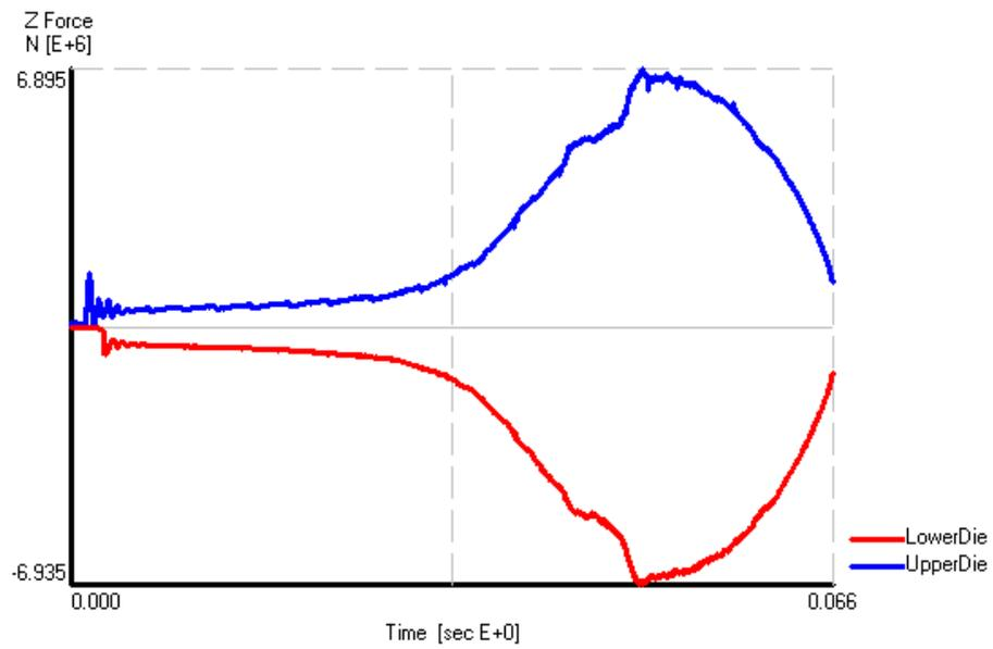
Figure 4.11 Die Load vs. Time Graph of X20Cr13 at 1180 °C
