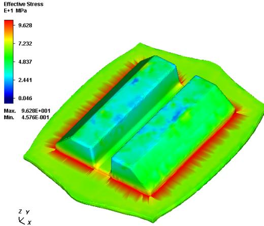
Figure 5.9 Effective Stress Distributions for Bearing Steel at 90 % of the Final Stroke
