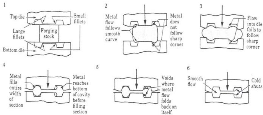
Figure 1.3 Effect of Fillet Radius on Defect Formation in Forging. On The Right Side of Drawings Small Fillets are Shown Causing Defects [2]
