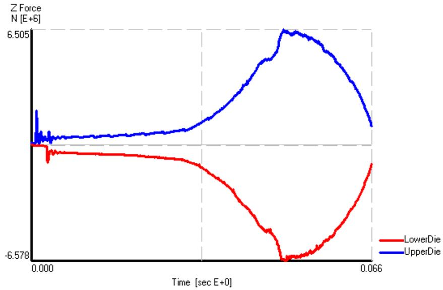
Figure 4.10 Die Load vs. Time Graph of C60 at 1100 °C
