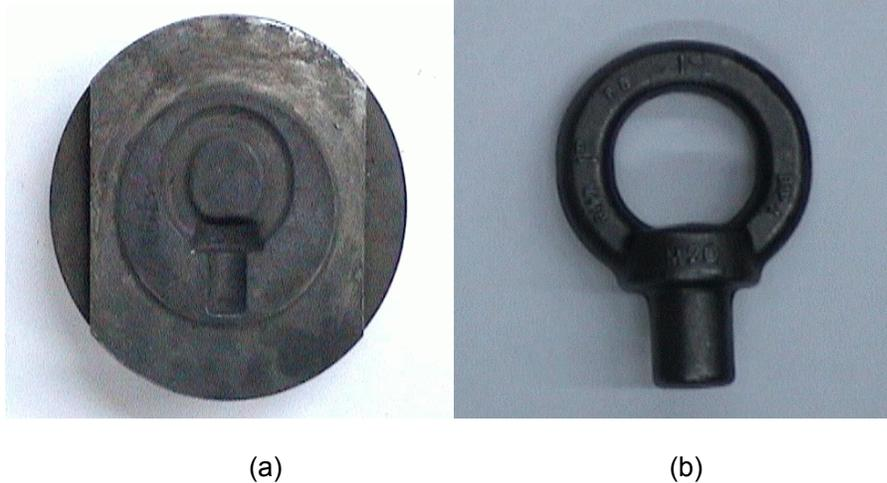
Figure 4.3 (a) Finish Die Used for the Forging of M20 Eye Bolt and (b) The Final Product
