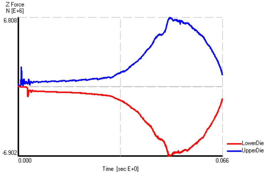
Figure 4.8 Die Load vs. Time Graph of C45 at 1100 °C
