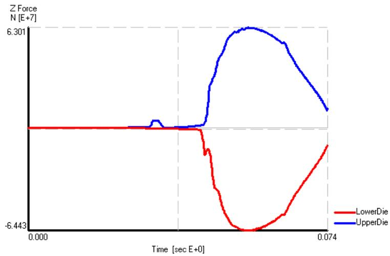
Figure 5.6 Die Loads in the Final Stage of Process for the Bearing Steel, 100Cr6
