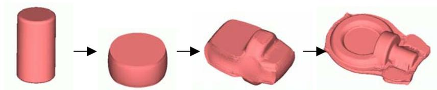
Figure 4.16 Process Simulation of Forging M30 Eye Bolt
