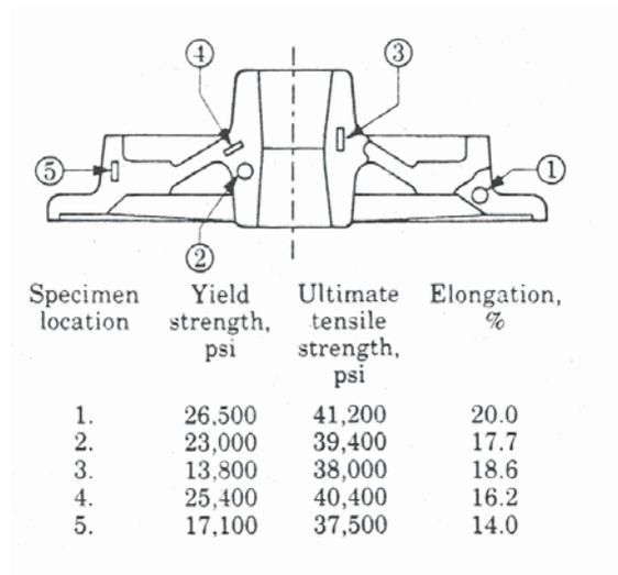
Figure 1.4 Mechanical Properties of Five Tensile Test Specimen Taken at Various Locations and Directions in an AZ61 Magnesium Alloy Forging [2]
