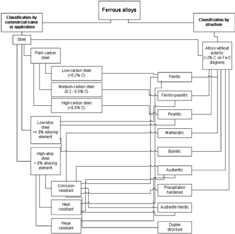
Figure 2.2 Classification of Ferrous Alloys [17]
