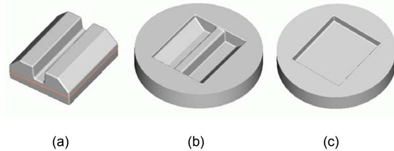
Figure 5.4 (a) The Final Product, (b) The Upper Die, (c) The Lower Die
