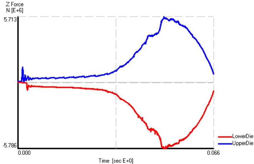
Figure 4.14 Die Load vs. Time Graph of 100Cr6 at 1100 °C
