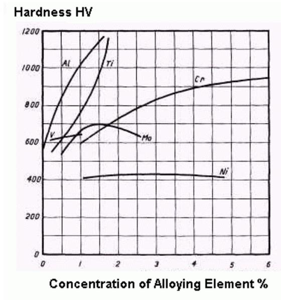
Figure 2.1 Hardening Effects of Alloying Elements in Solid Solution After Nitriding [17]
