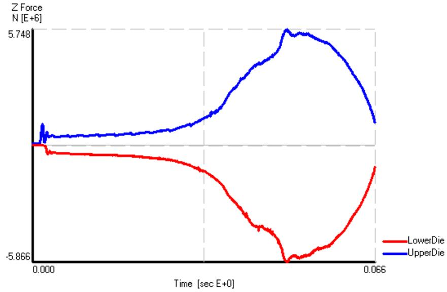
Figure 4.12 Die Load vs. Time Graph of 42CrMo4 at 1150 °C
