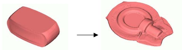
Figure 4.6 The Final Forging Stage of the Operation
