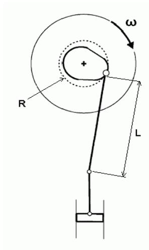
Figure 4.4 Input Parameters for the 10 MN (1000 tonf) Mechanical Press
