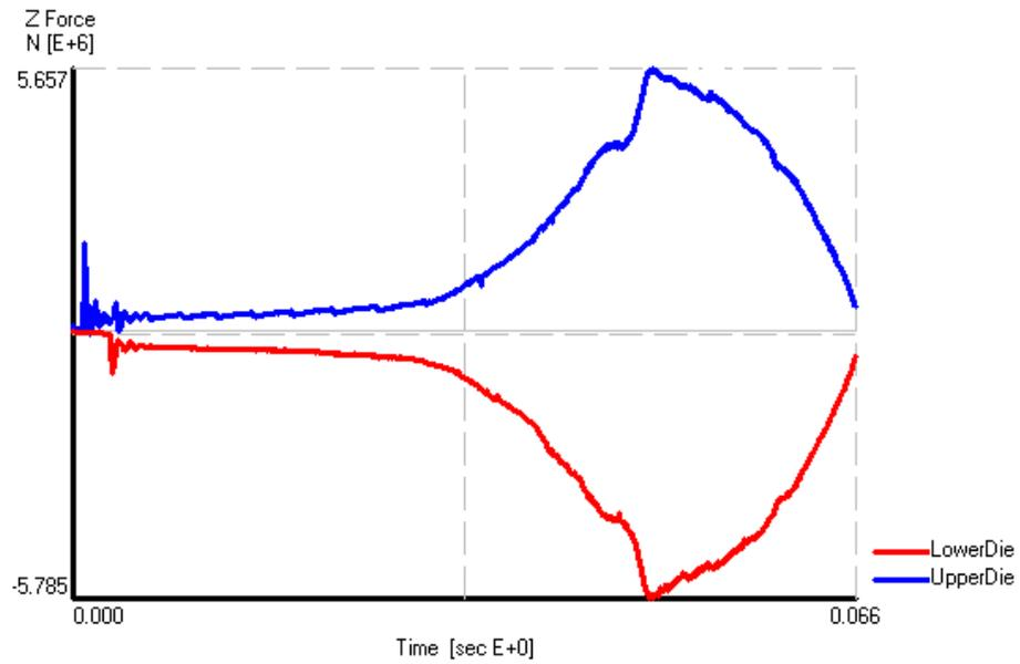
Figure 4.13 Die Load vs. Time Graph of 100Cr6 at 1150 °C
