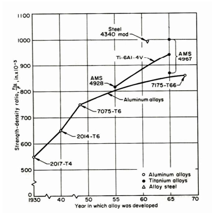
Figure 1.5 Room Temperature Strength-Density Ratios of Aerospace Materials [5]
