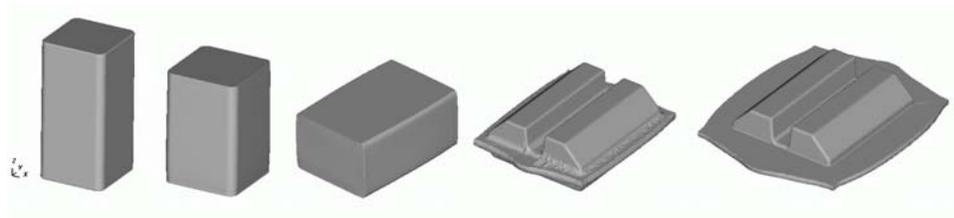
Figure 5.5 Simulation of the Forging Sequence
