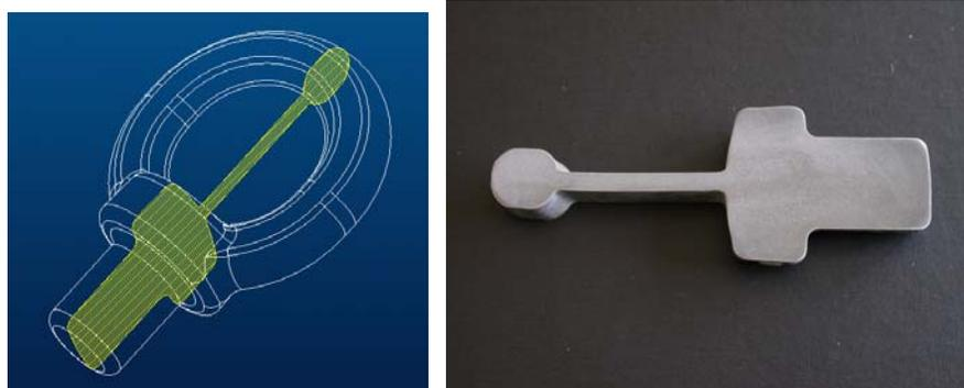
Figure A.1 A C45 Sample Taken out from the Symmetry Plane
