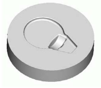
Figure 4.15 The Proposed Geometry of the Preform of M30 Eye Bolt
