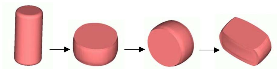
Figure 4.5 Upsetting and Flattening Stages of M20 Forging
