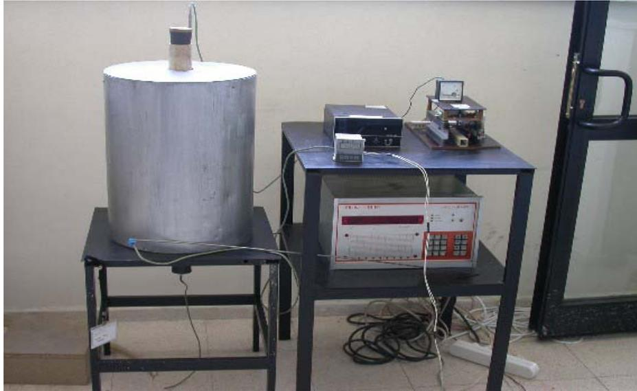
**Figure 3.9.** Furnace used in the foaming experiments.
