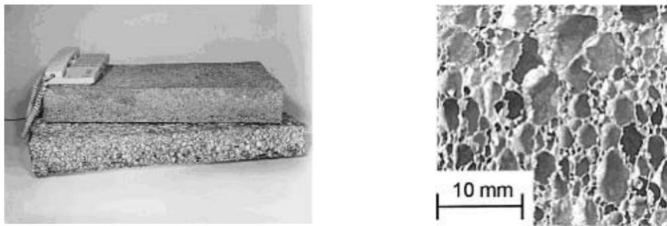
**Figure 2.2.** Structure of Cymat foams produced by gas injection method (Banhart, 2001 and Körner et al. 2000)
