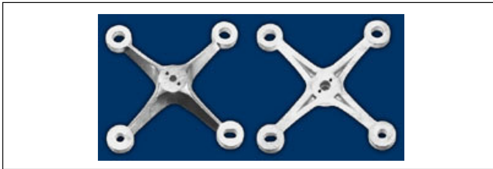
Figure 4.5. Aluminium with satin finished surface, produced by lost wax casting method, heavy-duty spiders for steel supported structures. Source: www.sadev.com , 2003
