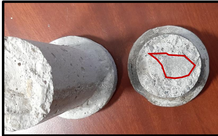
Figure 3-9 Location of Single Coarse Aggregate in the sample with M1 tested at the 29 th day
