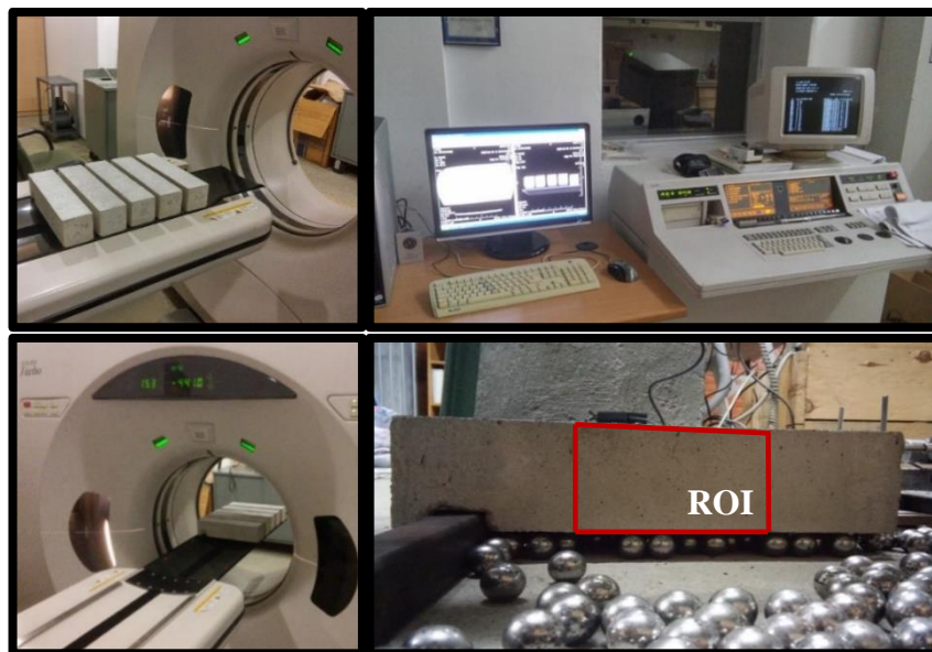
Figure 4-12 Scanning Concrete Samples via Tomography
