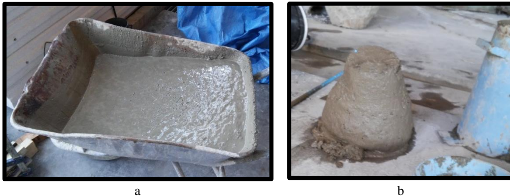
Figure 3-5 Concrete Mix (a), Slump Test (b)
