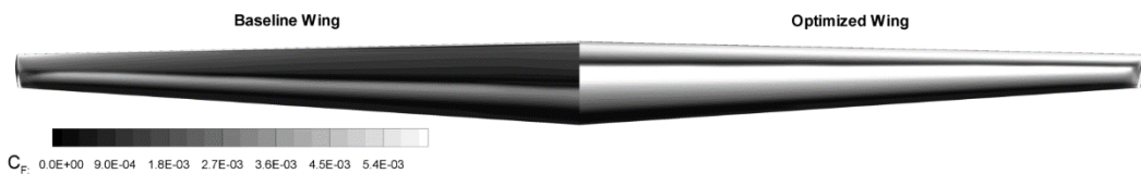
Figure 3-55 Skin friction coefficient distribution on the upper surfaces of the baseline and the optimized wing
