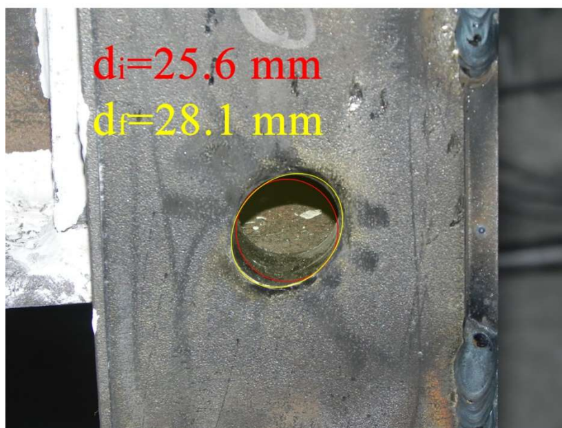
Figure 4.16. Bolt hole elongation
