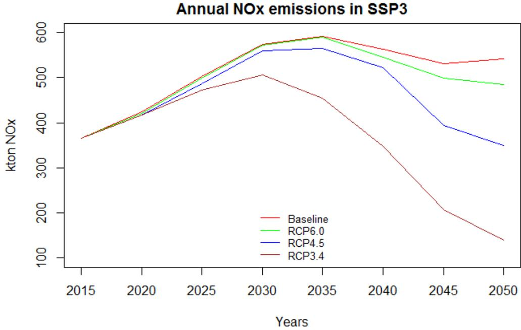
Figure 3.63:  $NO_x$  emissions from power generation for RCPs in SSP3
