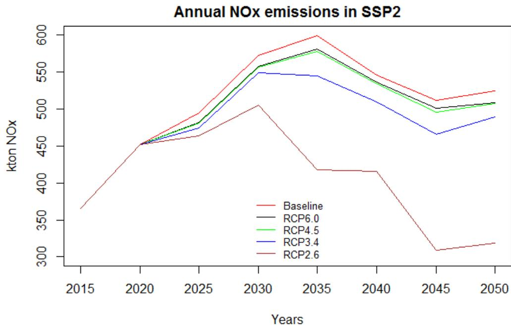
Figure 3.61:  $NO_x$  emissions from power generation for RCPs in SSP2
