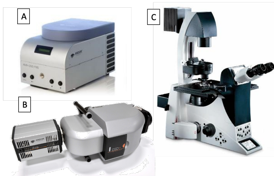
Figure 2.4: Image of the microscope components showing A: Andor AMH200 Metal Halide lamp, B: Zyla 5.5 sCMOS and DSD2 Differential spinning disc and C: Leica DMI4000B.
