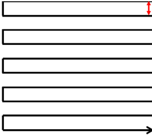
Figure 1.4: Raster scan diagram used for laser structuring
