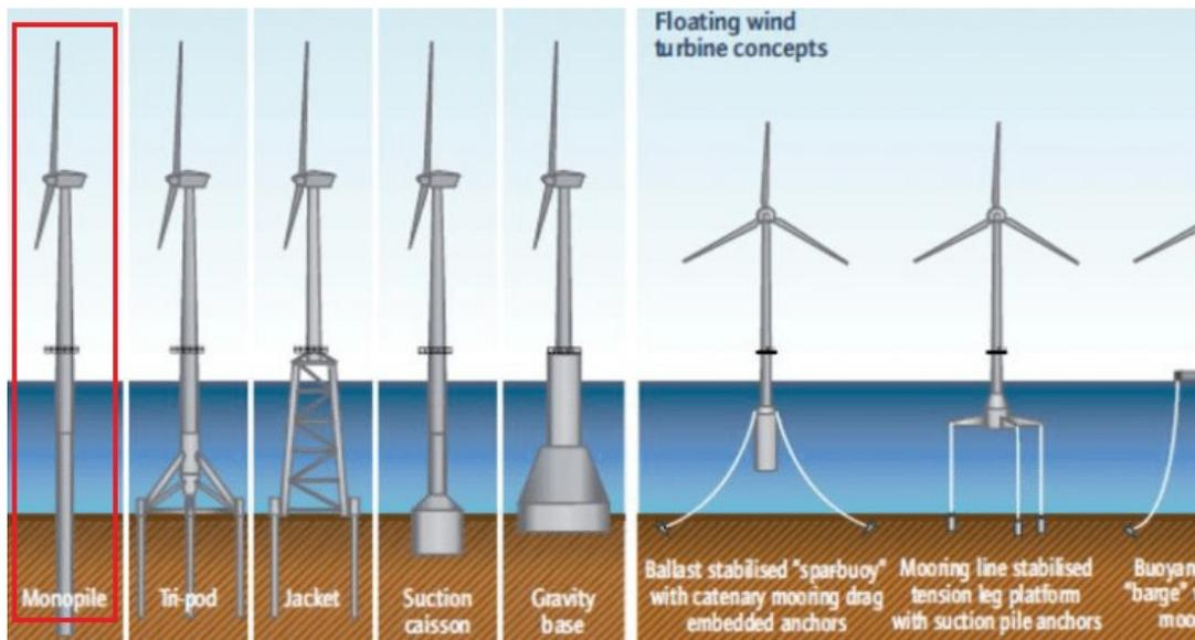
Figure 4.2 Foundation types for an offshore wind farm<sup>5</sup>
