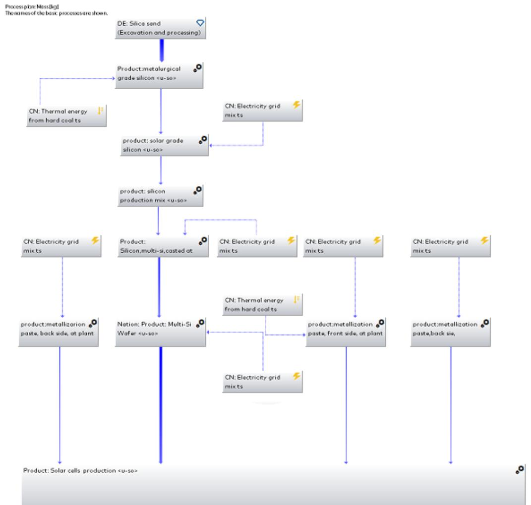
Figure 3.2 Model of manufacturing of solar cells
