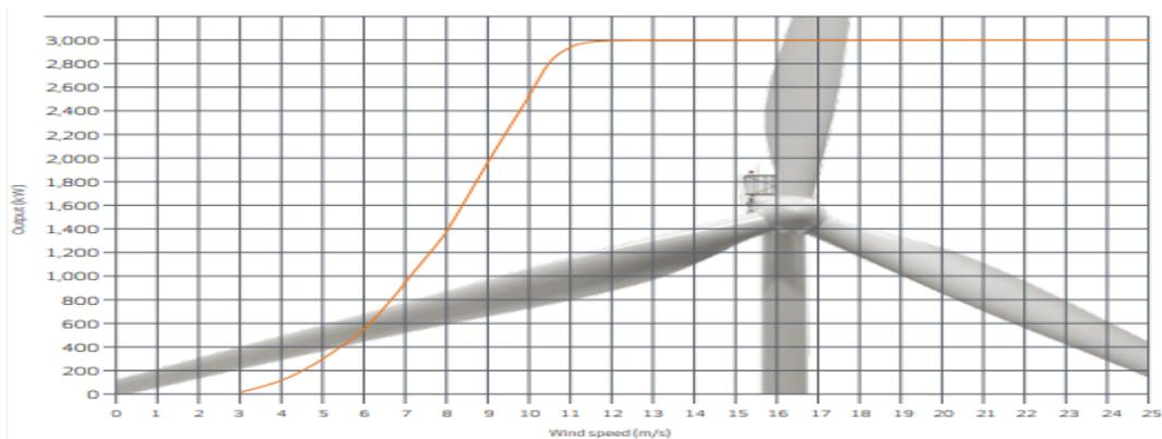
Figure 4.3 Power curve-Vestas V-112-3 MW-Offshore<sup>6</sup>
