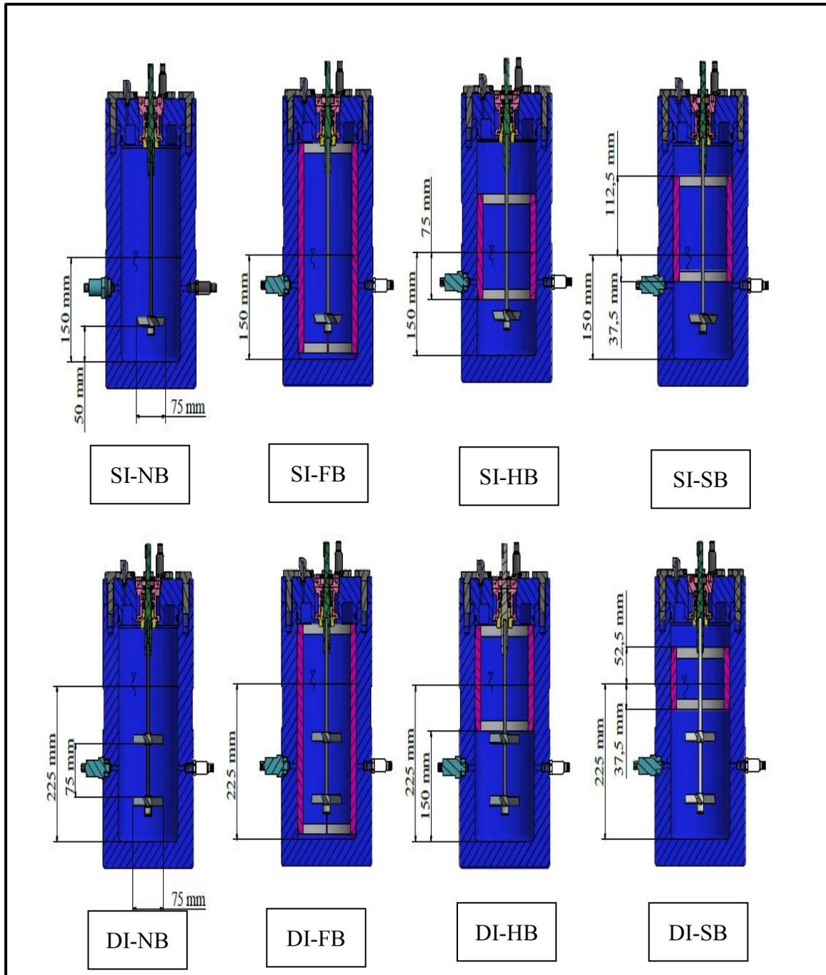
**Figure 5.8** Types of impellers used in this study,
