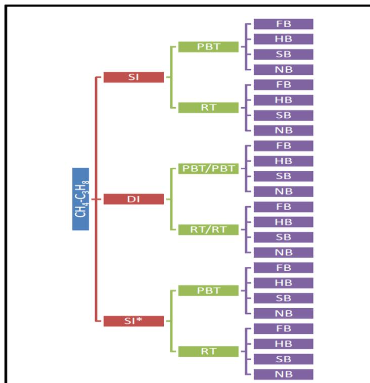
1. **Figure 7.1** Repeatability Diagram showing the impeller – baffle configurations of 24 methane -propane mixture hydrate experiments
