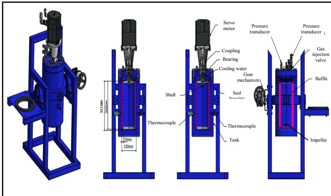
**Figure 5.2** High-pressure stainless steel reactor
