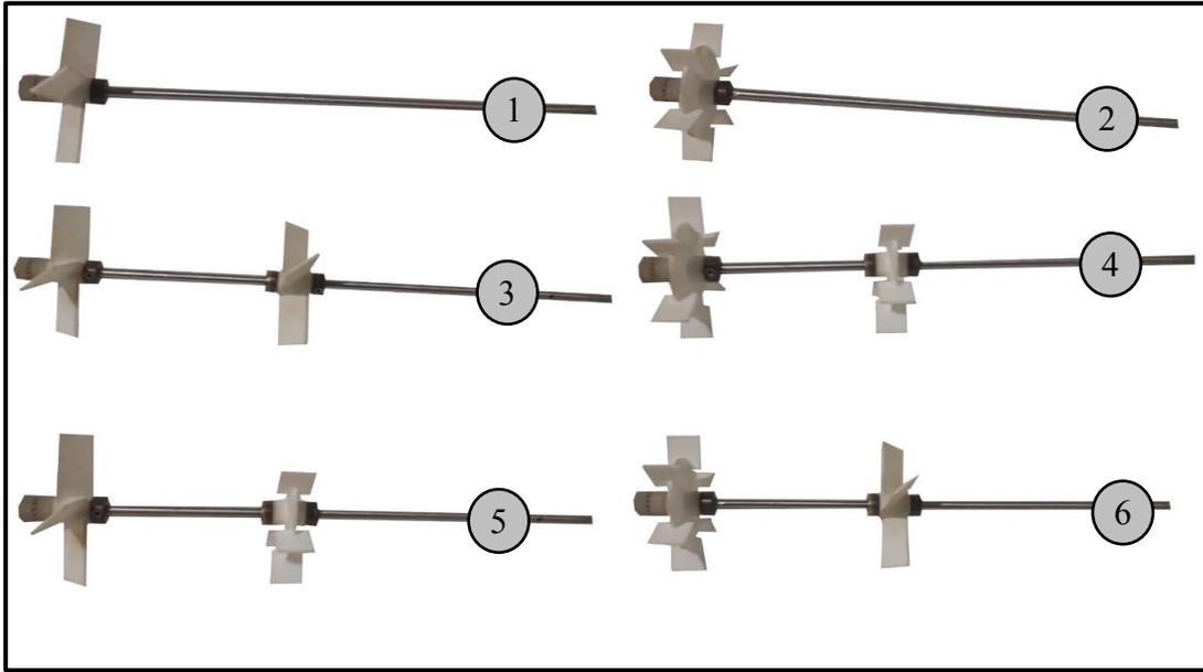
**Figure 5.5** Different impeller arrangements
