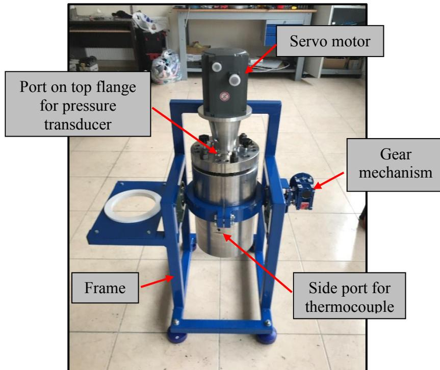
**Figure 5.3** Some components of High-pressure stainless steel reactor
