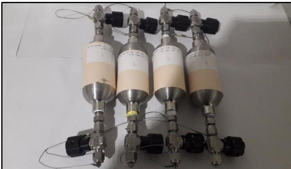
*Figure 5.14* Steel tubes for gas sampling
