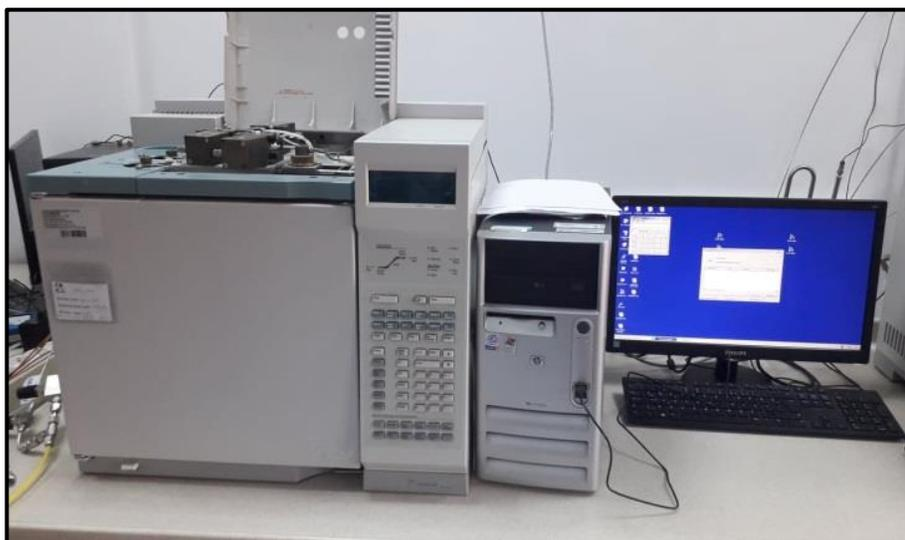
*Figure 5.15* Agilent system 6890 series GC for gas analysis
