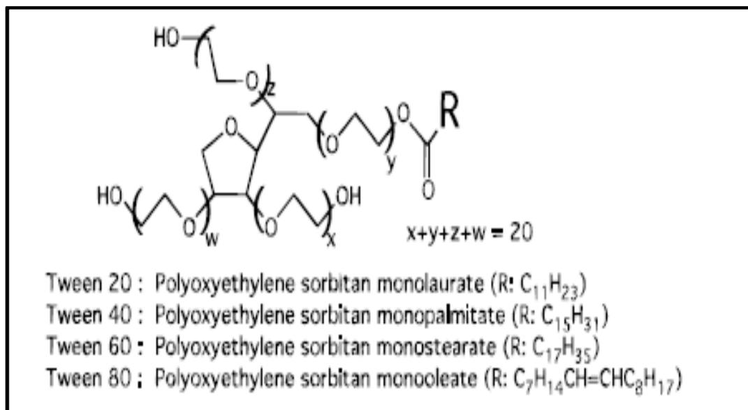
**Figure 3.5** Structure of the ethoxylated sorbitan tween surfactants. The EO groups are randomly distributed over the four available sites [184]
