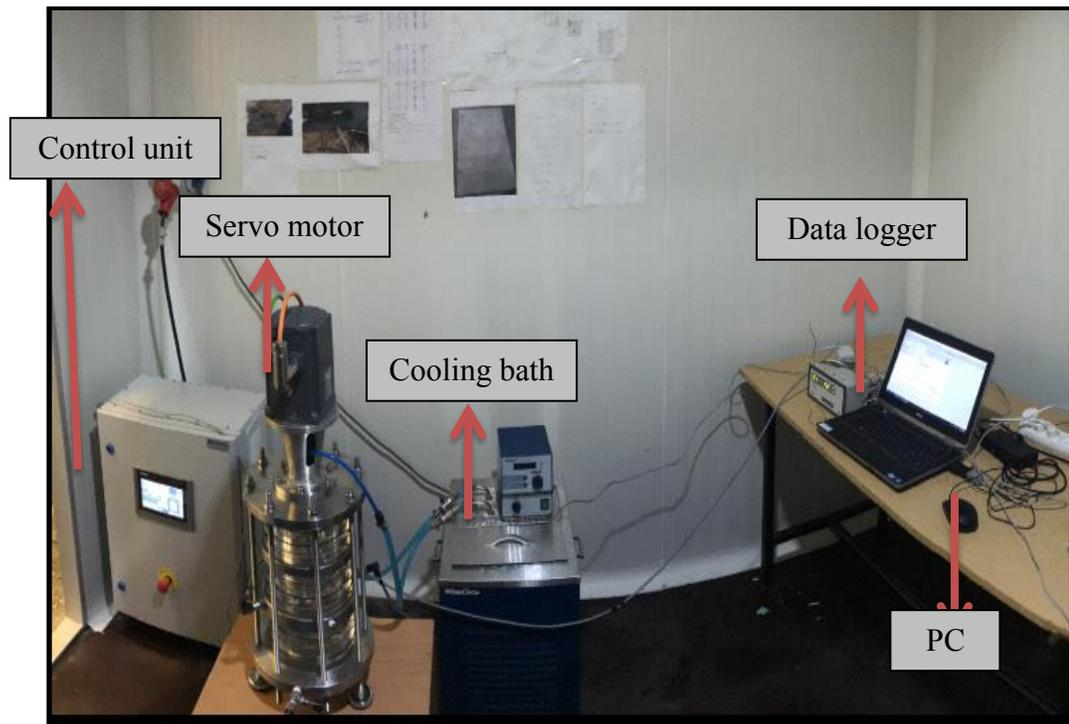
**Figure 5.9** Experimental setup of transparent reactor
