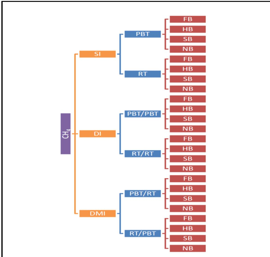
**Figure 6.6** Diagram showing the impeller – baffle configurations of 24 methane hydrate experiments
