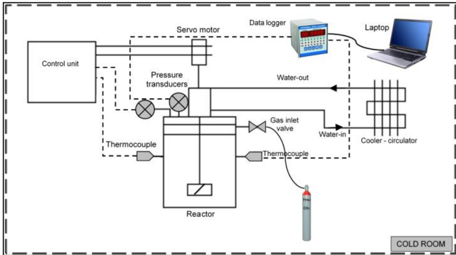
*Figure 5.1* Experimental set-up for hydrate formation
