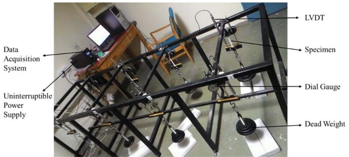
Figure 3.8 General view of the creep test setup
