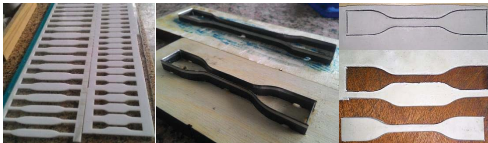
Figure 3.4 Specimen Preparation by Molding and Die cutter
