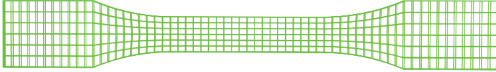
Figure 6.4 The mesh geometry of the specimen
