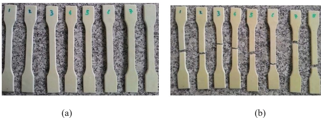
Figure B. 3. Specimen Photos Before (a) and After (b) Tensile tests (TSL-1, 14-day)
