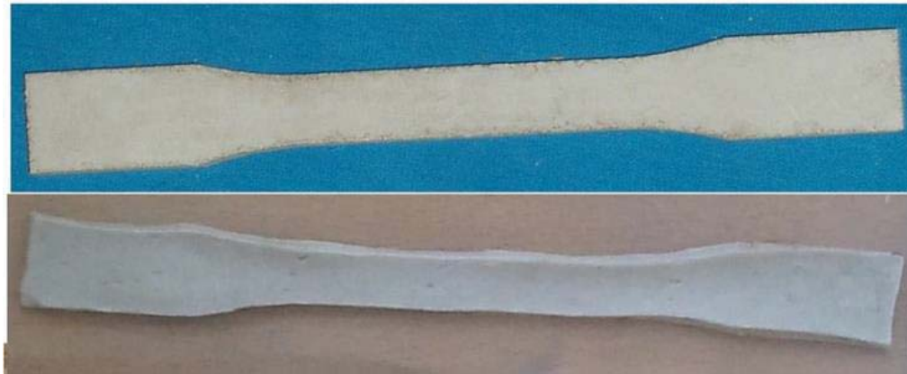
Figure 3.9 Standard and shrunk test specimens (Guner, 2014)
