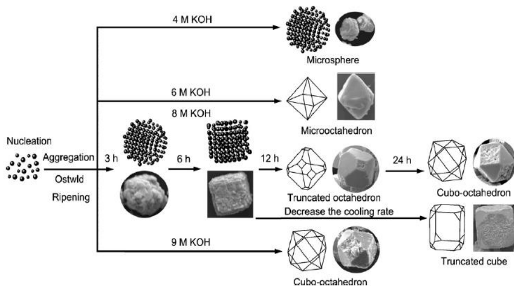
Figure 2.13. A schematic illustration of formation mechanism of BFO under different molar concentration [82].
