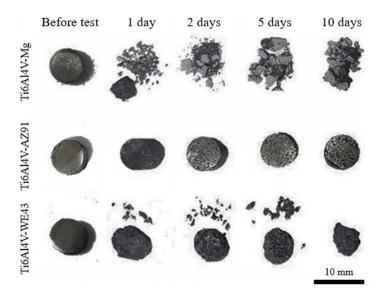
Figure 4.68. Macro-structural changes of composites during in-vitro tests [195].
