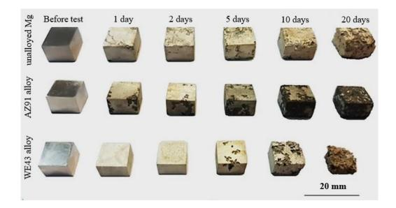
Figure 4.60. Macro-structural changes of Mg/Mg-alloys after immersion in SBF.
