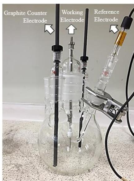
Figure 3.6. The electrochemical cell containing three electrodes.
