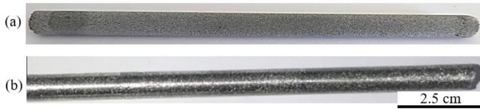
Figure 4.22. Macro images of (a) porous Ti6Al4V alloy rod and (b) manufactured Ti6Al4V-Mg composite rod.
