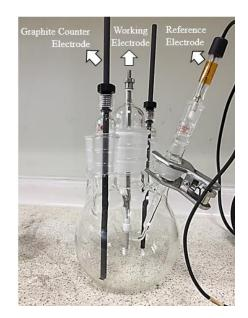
Figure 3.6. The electrochemical cell containing three electrodes.
