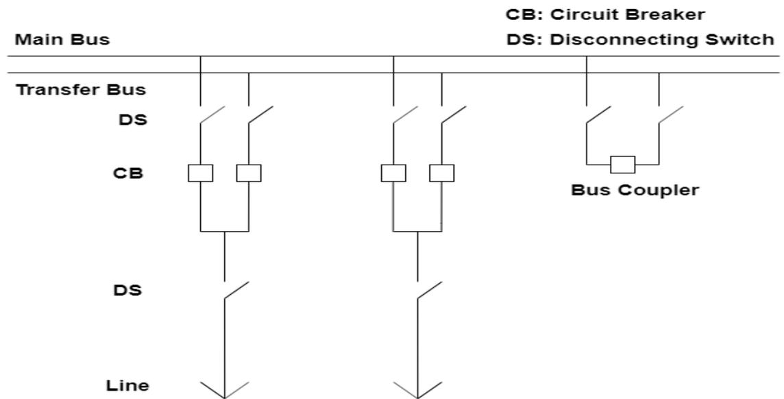
Figure 2.5. Double Busbar Double Breaker Configuration
