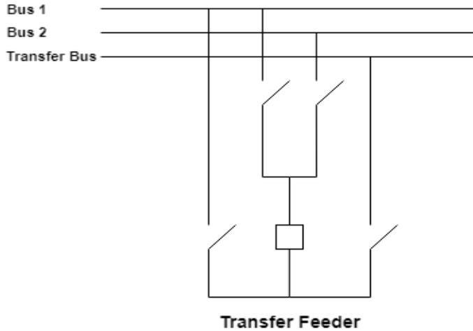
Figure 3.3. A Transfer Feeder Configuration in a Substation
