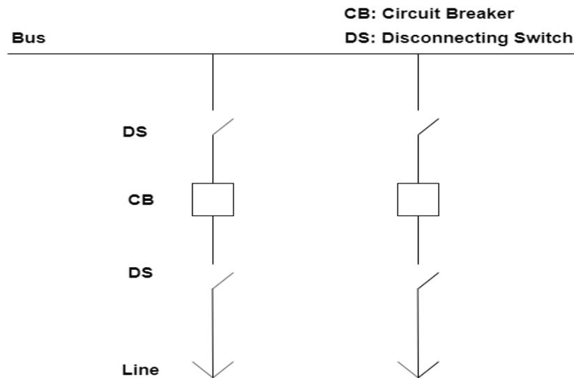
Figure 2.2. Single Busbar Configuration
