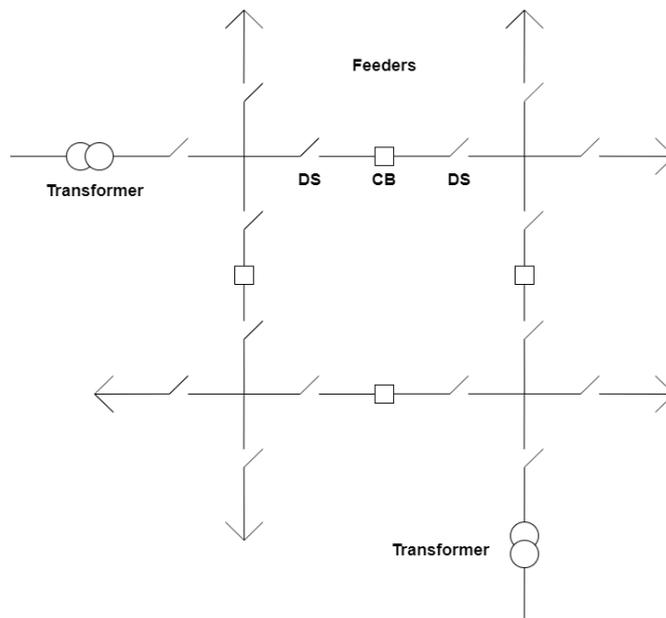
Figure 2.7. Mesh Configuration
