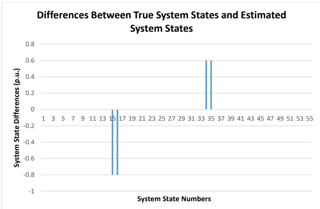
Figure 4.14 Large Scale Substation Scenario Topology Error Detection - Differences Between True System States and Estimated System States for Topological Error in Feeder Bays
