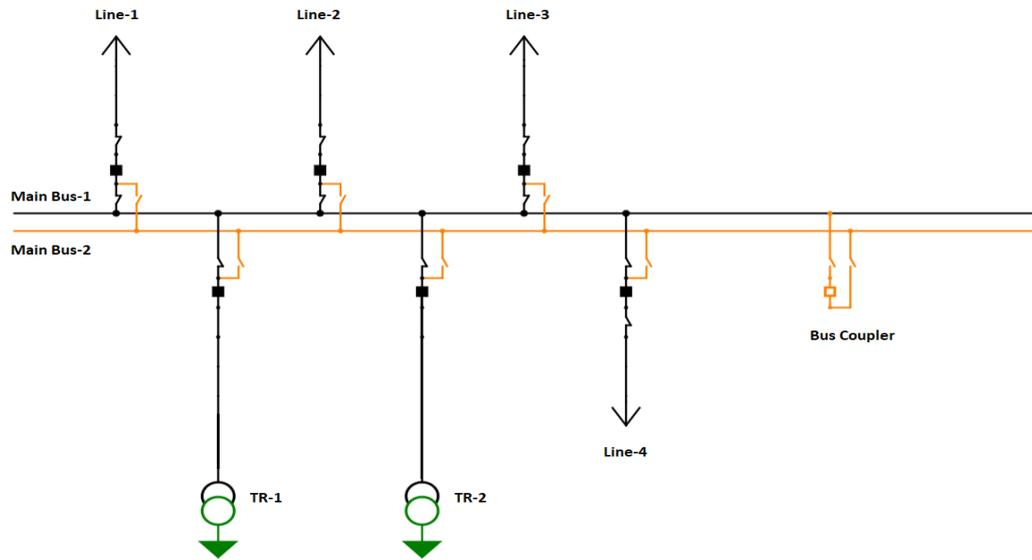
Figure 2.11. A Two Main Buses Configuration Example
