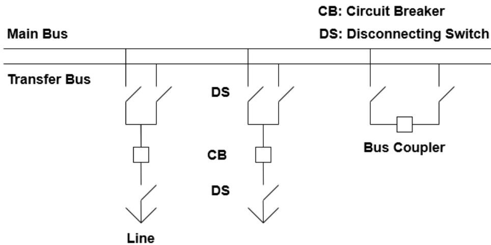
Figure 2.3. Double Busbar Single Circuit Breaker Configuration
