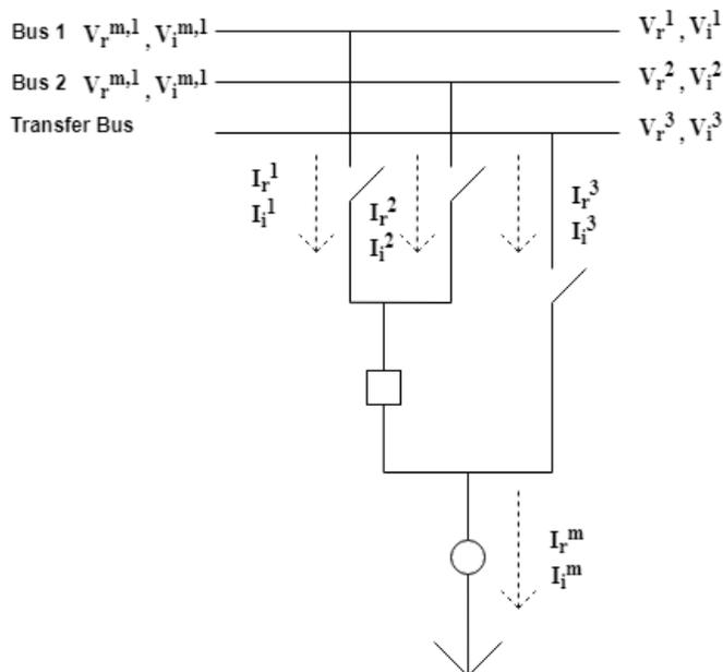
Figure 3.2. Current and Voltage States in a Substation
