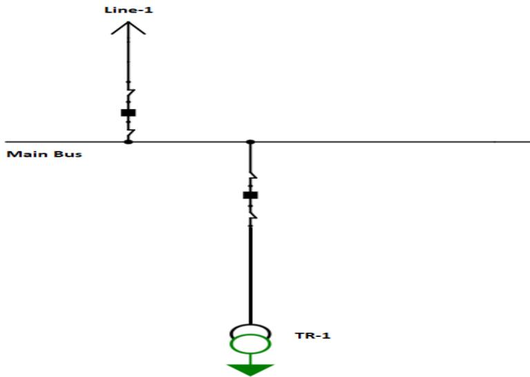
Figure 2.9. A Single Busbar Configuration Example
