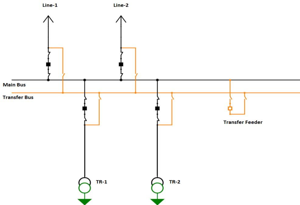
Figure 2.10. A Main Bus and a Transfer Bus Configuration Example
