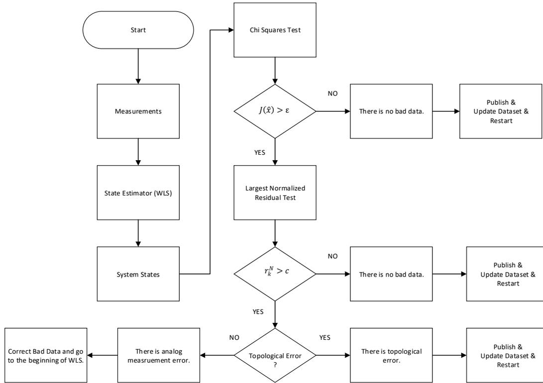
Figure 3.4. Flow Chart of the Bad Data Processor
