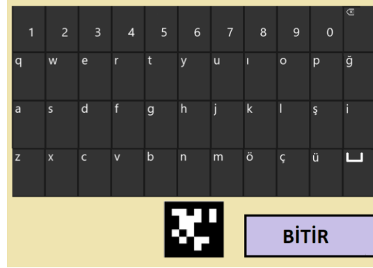
Figure 22: Keyboard with Apriltag tag36h11 marker
