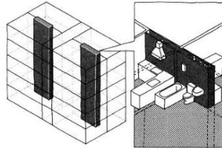
Figure 2.13. Vertical service distribution (Schneider & Till, 2007, p. 198)
