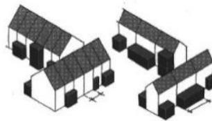
Figure 2.2. Vertical additions (Schneider & Till, 2007, p. 184)
