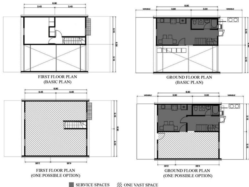
Figure 4.8. Service and post-created vast spaces in Villa Verde Housing (Elemental, 2013)
