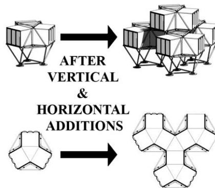
Figure 4.19. Vertical & horizontal additions in Plugin Tower (People's Architecture Office, 2016)
