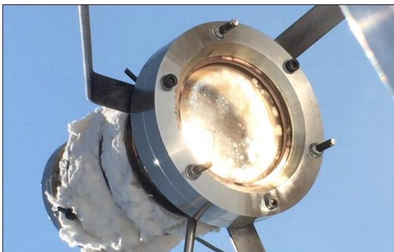
Figure 5.76. Solar reactor during the reforming operation
