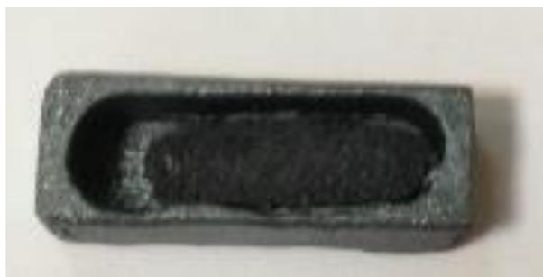
Figure 5.51. 316 stainless steel cartridge with SCFM (6473) after experiment
