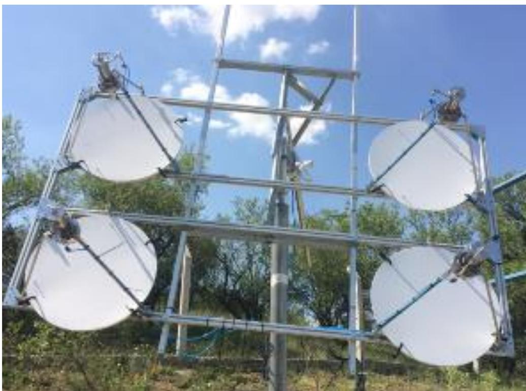
Figure 3.8. Concentrated solar energy pilot unit
