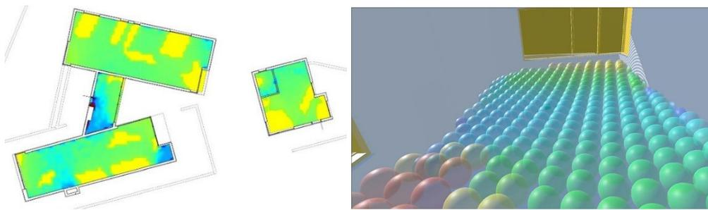
*Figure 3.10.* Autodesk Revit Insight and HoloArch's daylighting visualization
