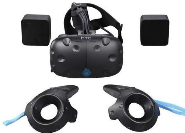
*Figure 3.3.* HTC Vive components<sup>79</sup>
