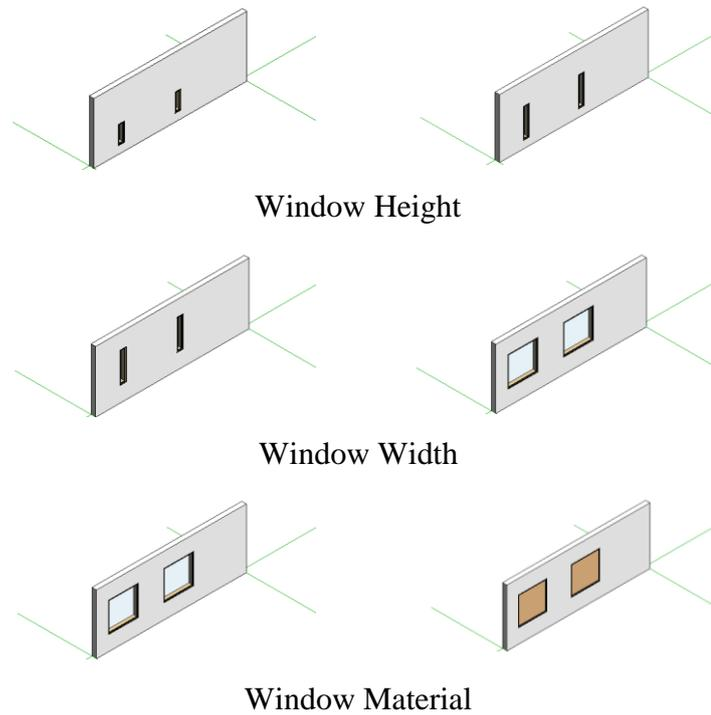
Figure 3.11. Some of the editable type parameters of window families
