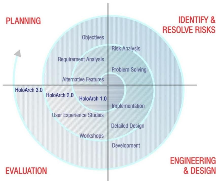
*Figure 3.4.* Spiral software development process model<sup>92</sup> for HoloArch
