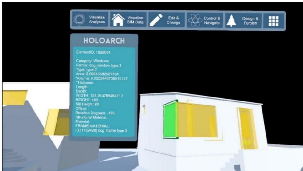
*Figure 3.16.* BIM data visualization of the selected window element
