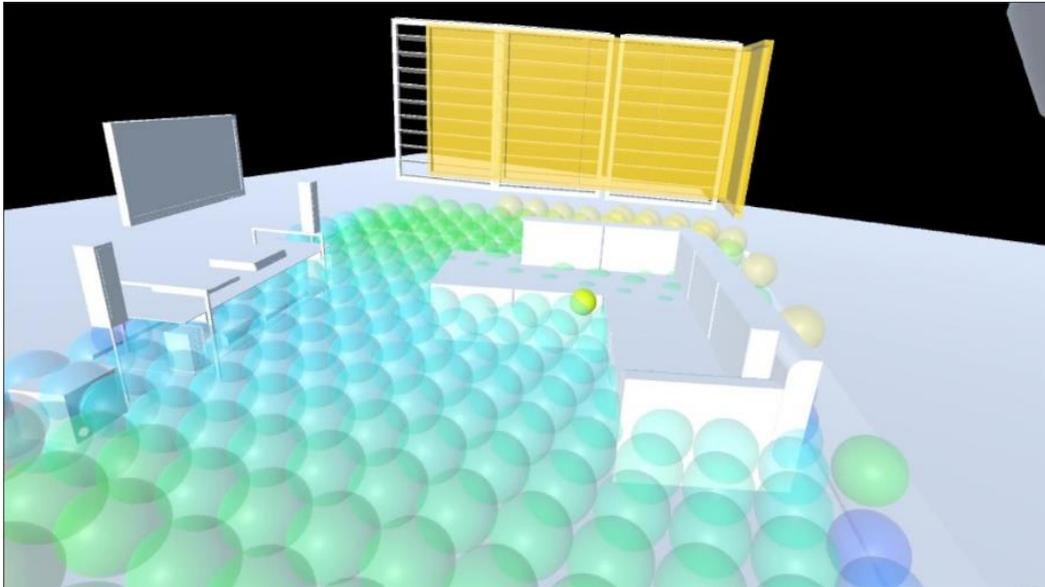
*Figure 3.23.* Space planning according to daylighting simulations
