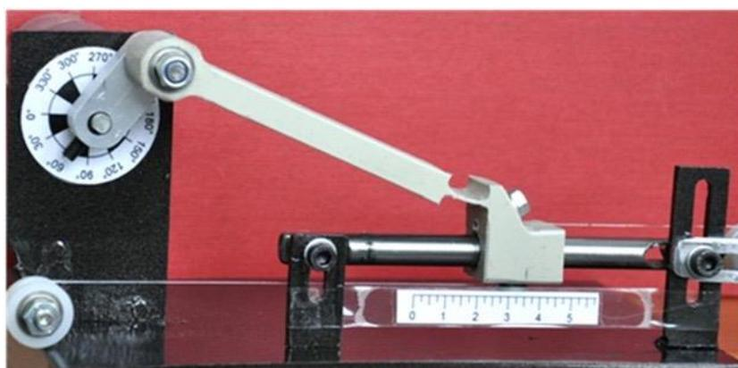
Figure 1.3. Manufactured partially compliant slider-crank mechanism [16]
