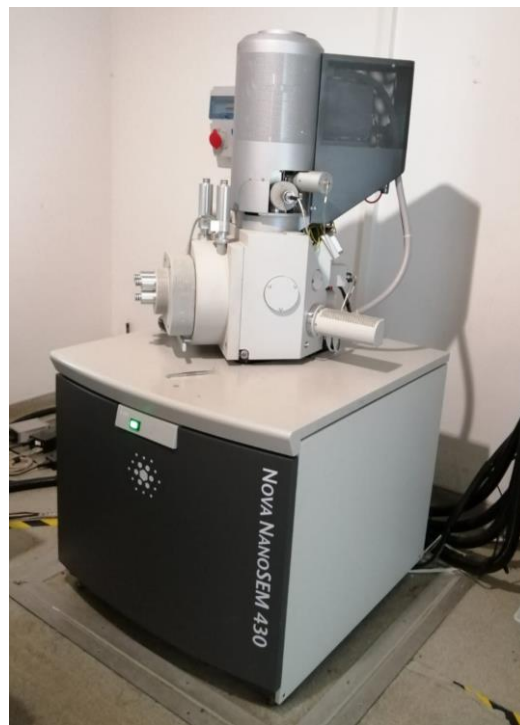
Figure 3. 5 Photography of FEI Nova NanoSEM 430 scanning electron microscope used in this study
