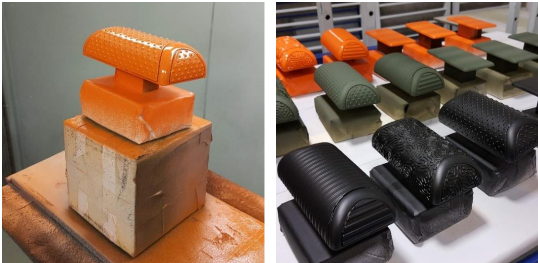
Figure 4.9. Coating process; black, green and orange
