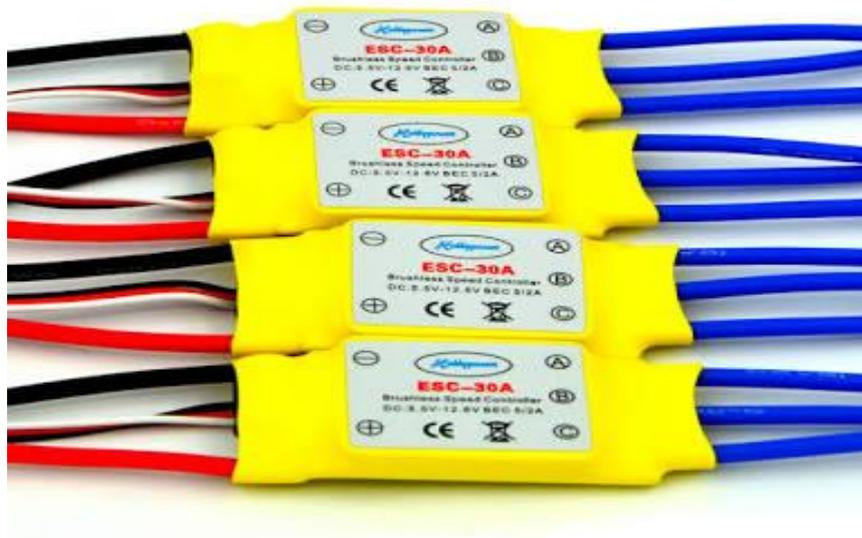
Figure 6.20 ESCs of the Quadcopter System [40]
