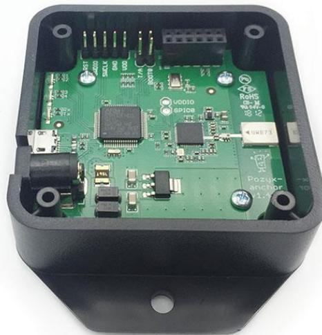
*Figure 6.14 Indoor UWB Localization System Unit Pozyx Anchor [60]*
