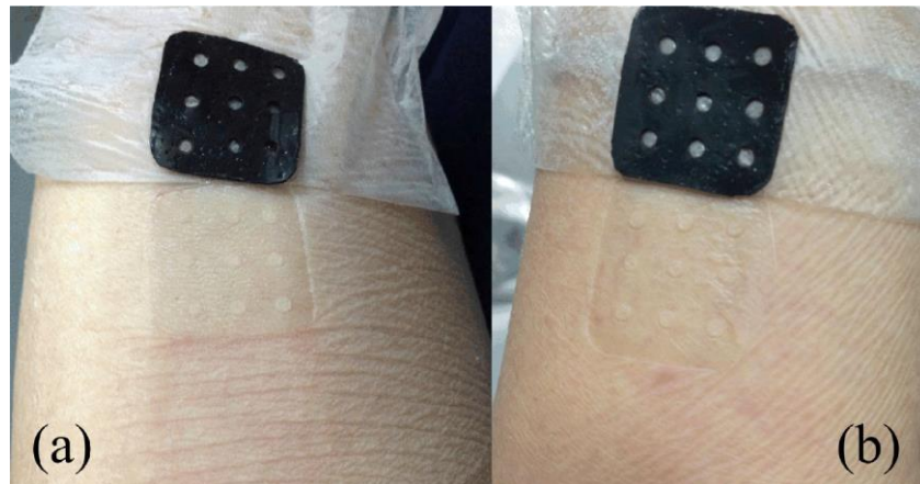
Figure 2.11 Photographs from skin compatibility test. The square electrodes were attached on the forearm. After (a) 1 week and (b) 2 weeks, no skin irritation was observed at either electrode contact area [10].
