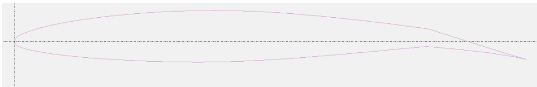
Figure 2.4. NACA 64-210 down airfoil structure
