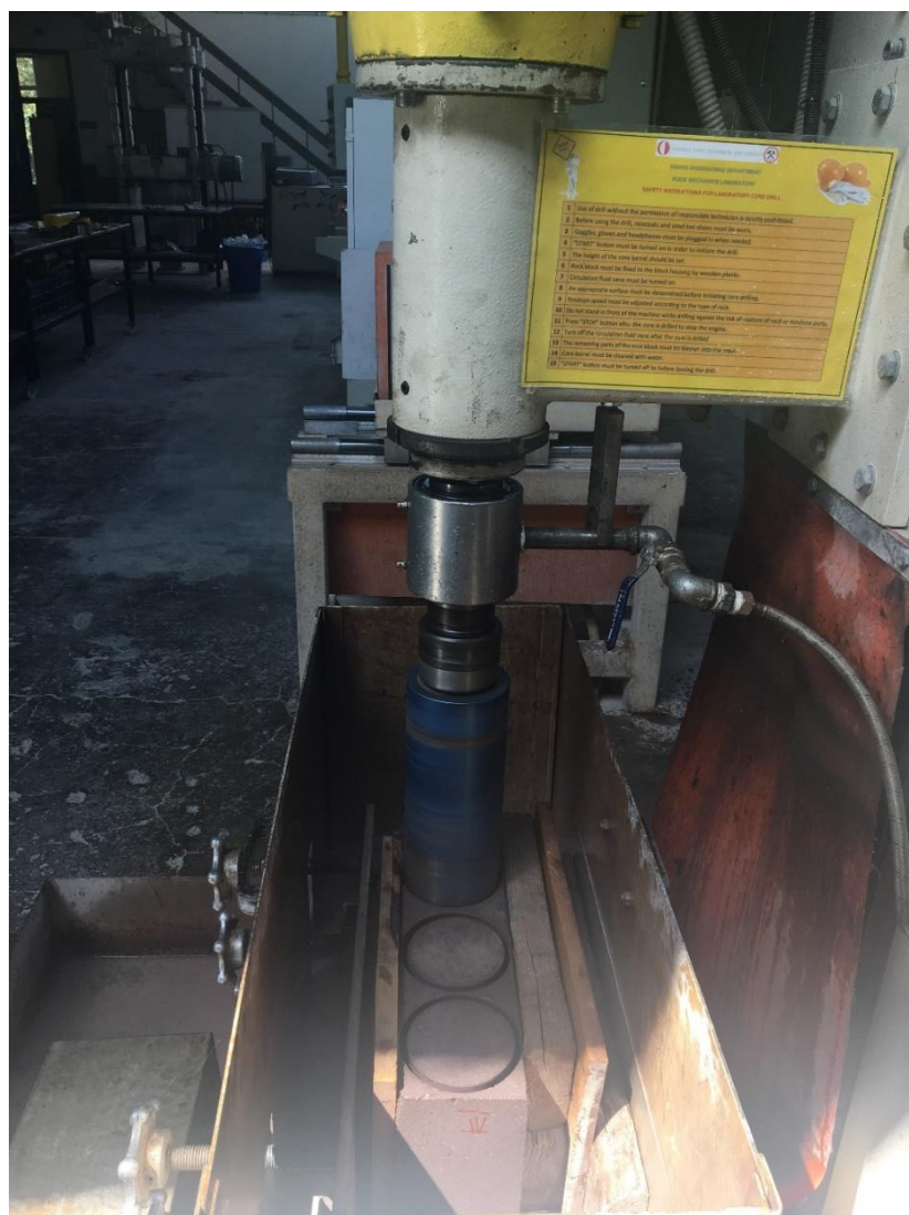
Figure 6.1. Rock coring machine
