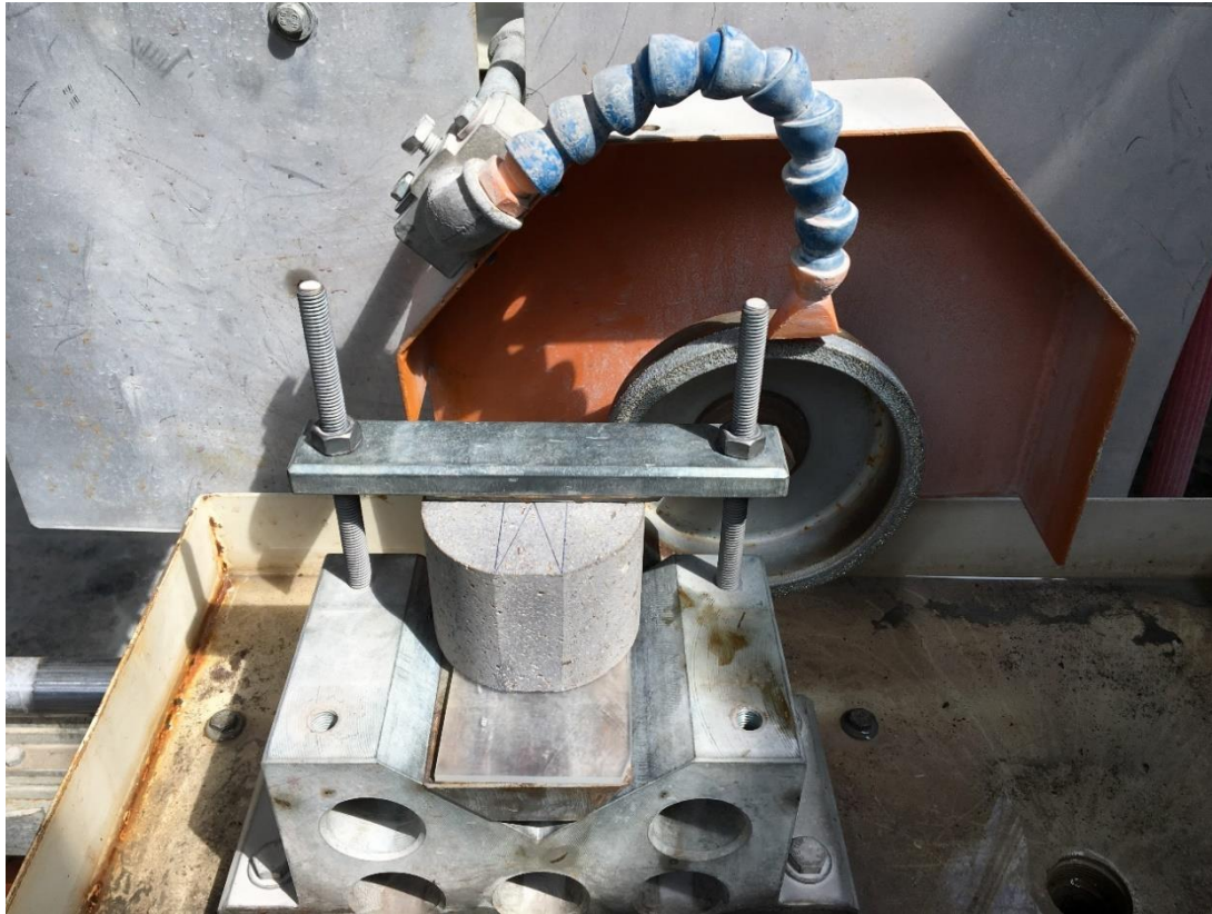
Figure 6.5. Flattening top and bottom ends
