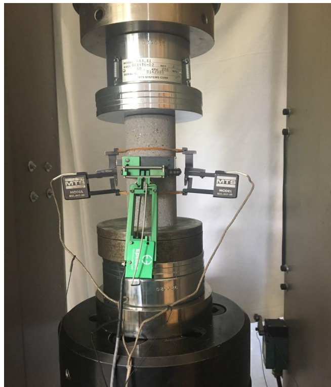
Figure 5.4. Static deformability test specimen with extensometers
