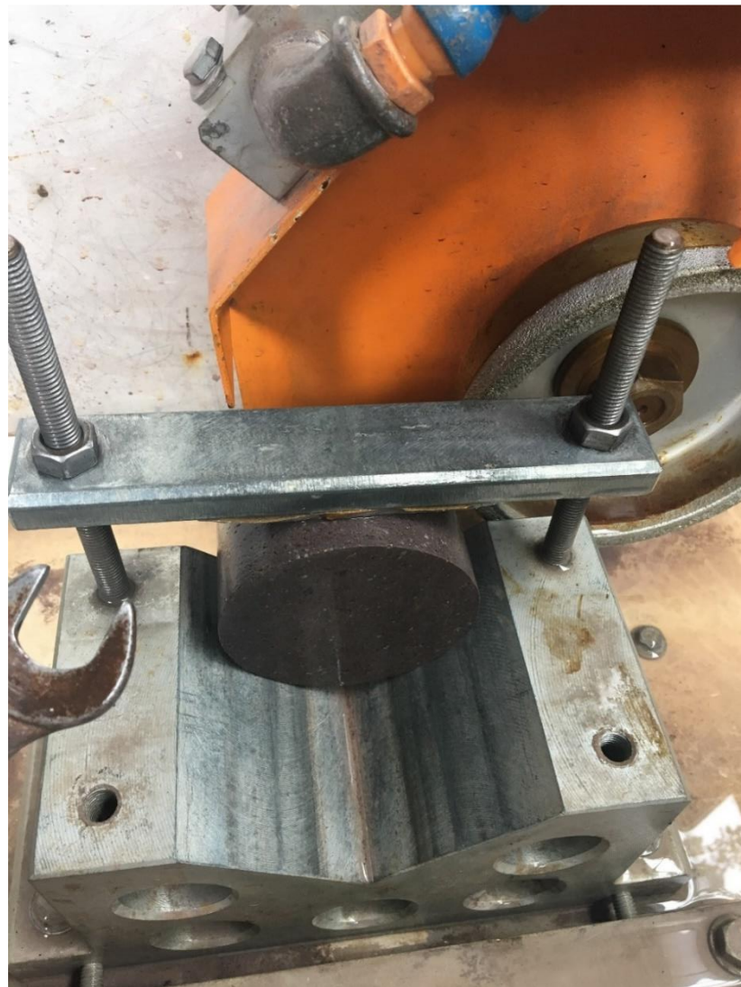
Figure 6.2. Thickness adjustment of specimen
