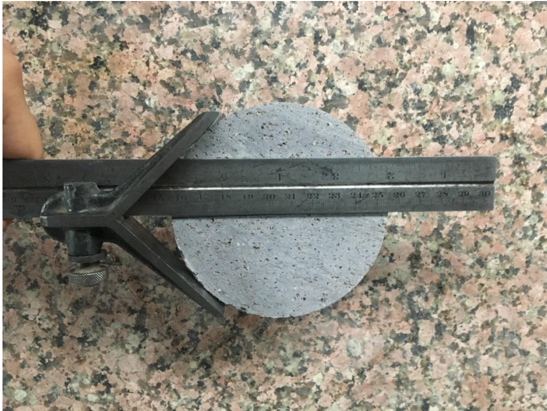
Figure 6.3. Diametral line positioning with the goniometer
