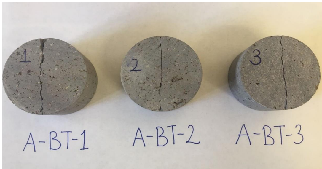
Figure 5.8. Failure pattern of Brazilian disc specimens
