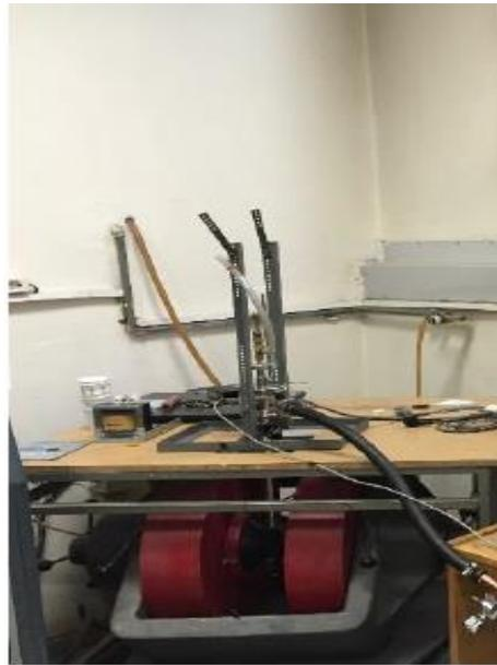
**Figure 3.10** Hall Effect Measurement System.
