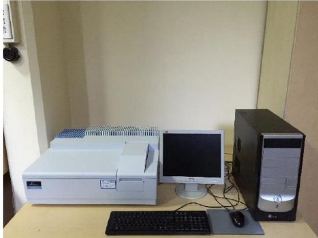
**Figure 3.8** Perkin Elmer Lambda 45 Spectrophotometer.
