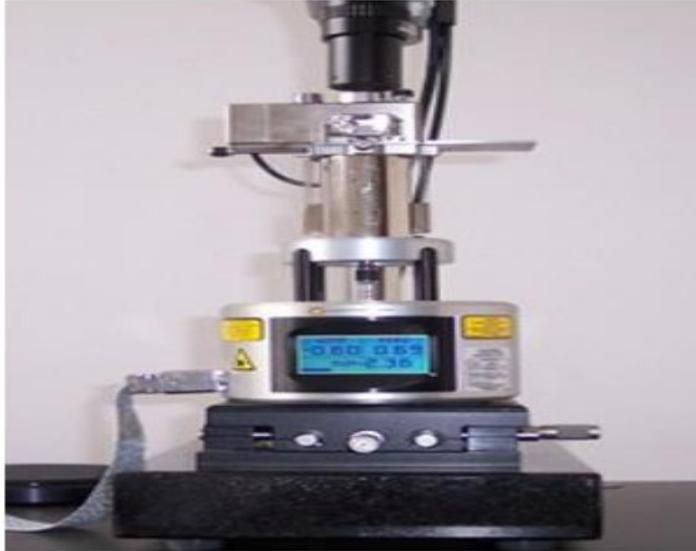
**Figure 3.7** Configuration of Atomic Force Microscopy at Central Laboratory.
