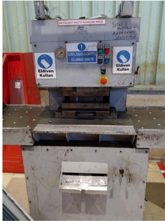
*Figure 3.5. Mechanical tensile test specimen press machine.*
