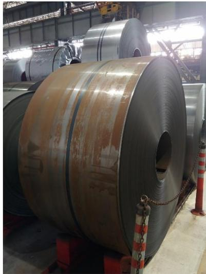
Figure 3.1. Steel strip coil in hot rolled state.
