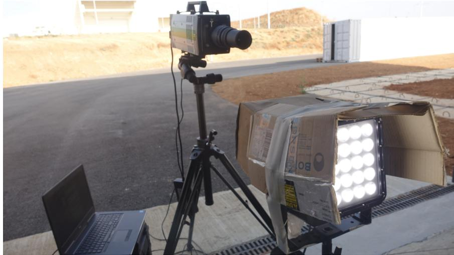
Figure 3.8: Light Source and High Speed Camera
